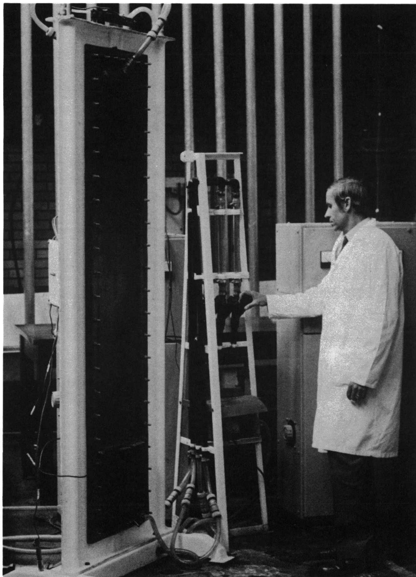
Pilot-scale cell used in the treatment of electroplating rinse water. The cell has a capacity of 20 l/min.
