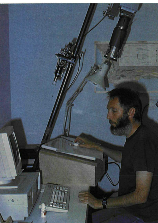
Mr Anton Scholtz at the apparatus he constructed whereby colour slides of cross-sections are projected onto the digitising tablet from which measurements are relayed to the computer.
