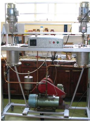
Figure 7: The reactor system with its oil heating system proved far more reliable in heating and maintaining the proper temperature. The small oil reservoir (silver cylinder below reactors) was later replaced with a much larger reservoir of similar shape and fitted with a breathing hole to avoid pressure build-up in the oil circulation system. The system is shown here without insulation cladding.
