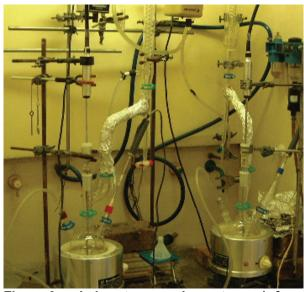
Figure 6: Laboratory equipment used for the synthesis of the first samples of the branched PEO-block-PSU copolymer. A network of cooling- and gas lines, the heating mantles and overhead stirrers as well as stirring motors mounted in a fume hood allows little free-work space. Such a system can only be expanded with difficulty and at high cost.
