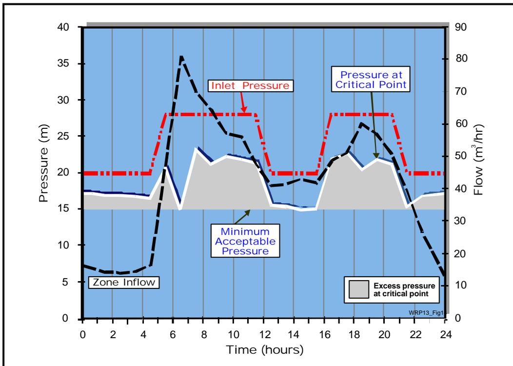
Figure 1.12: Typical zone with time-modulated pressure control
