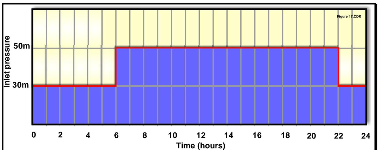
**Figure 2.1 Example of a (two-point) time-modulated pressure profile**
