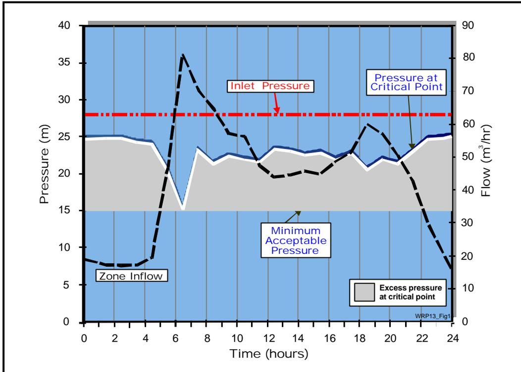
Figure 1.11: Typical zone with fixed-outlet pressure control
