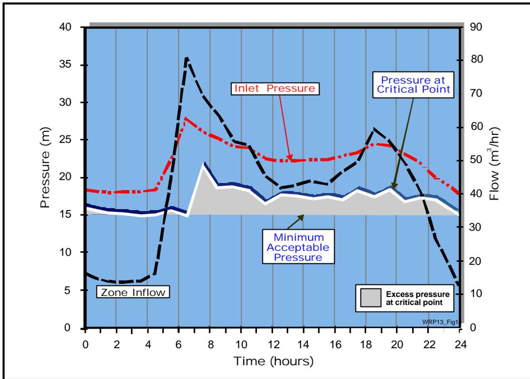
**Figure 1.13: Typical zone with flow-modulated pressure control**
