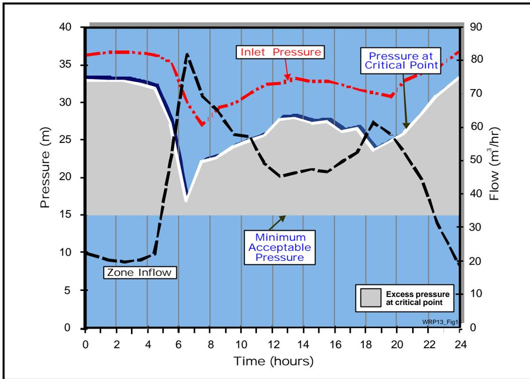
**Figure 1.10: Typical zone with no pressure control**
