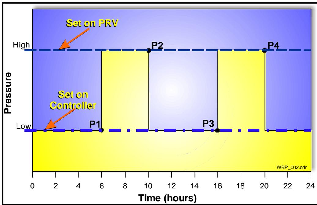
**Figure 1.4: Typical 4-point time modulated pressure profile**
