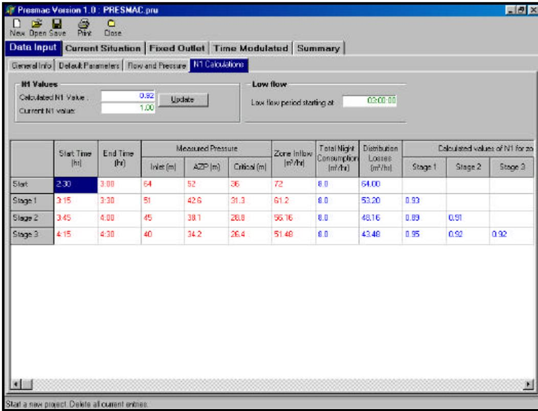
Figure 3.5 : Example of a Pressure Step-Test Analysis
