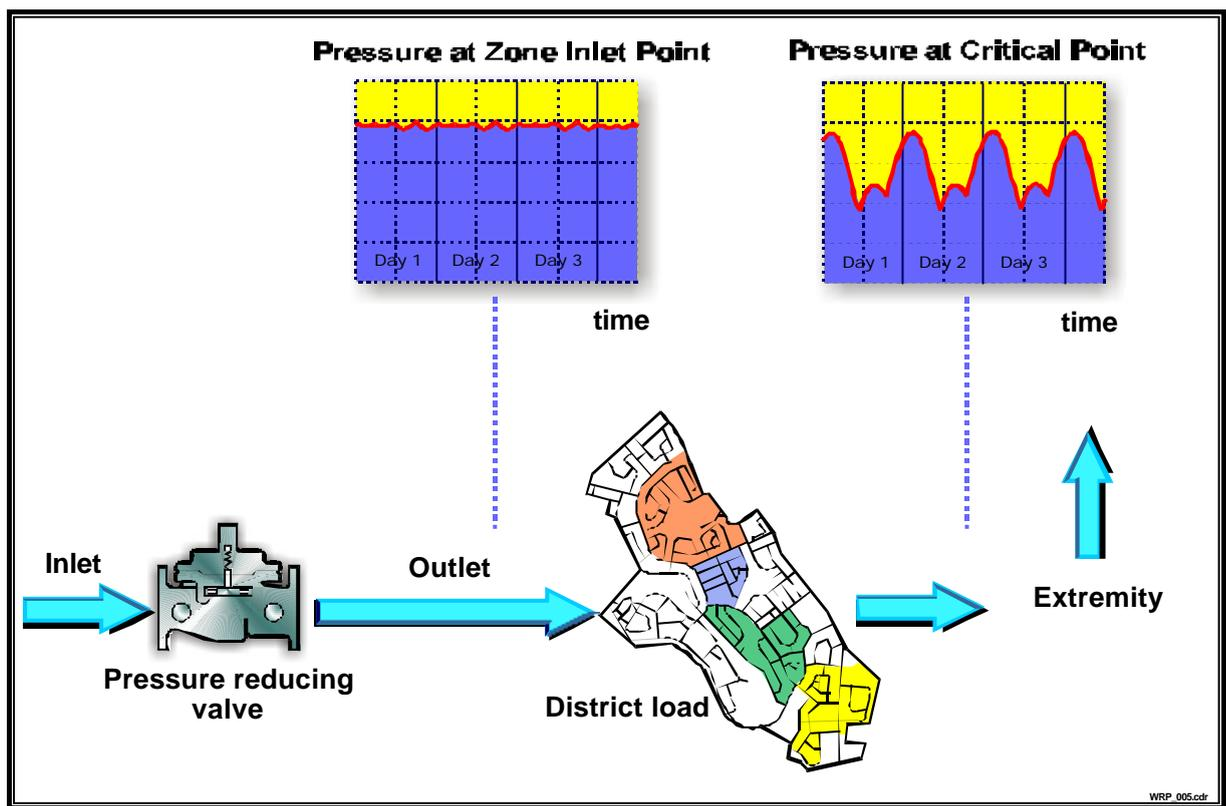
**Figure 1.3: Pressure control using conventional PRV**
