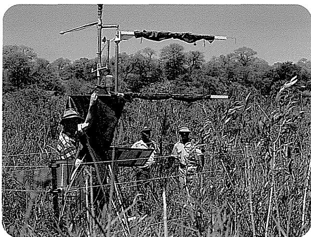
The Bowen ratio equipment and weather station used to monitor evaporation at the reed site in the Kruger National Park.
