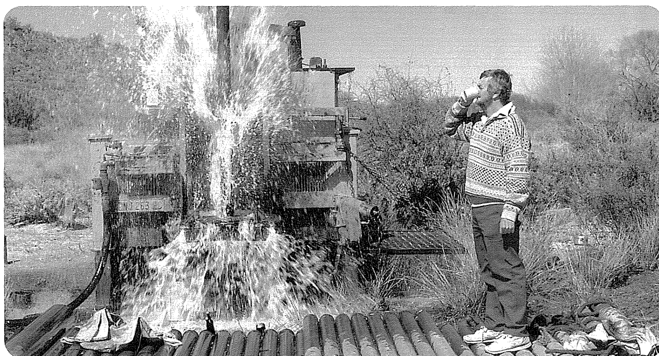
Successful siting of a borehole in the dolerite ring structures in the Karoo, near Victoria-West.
