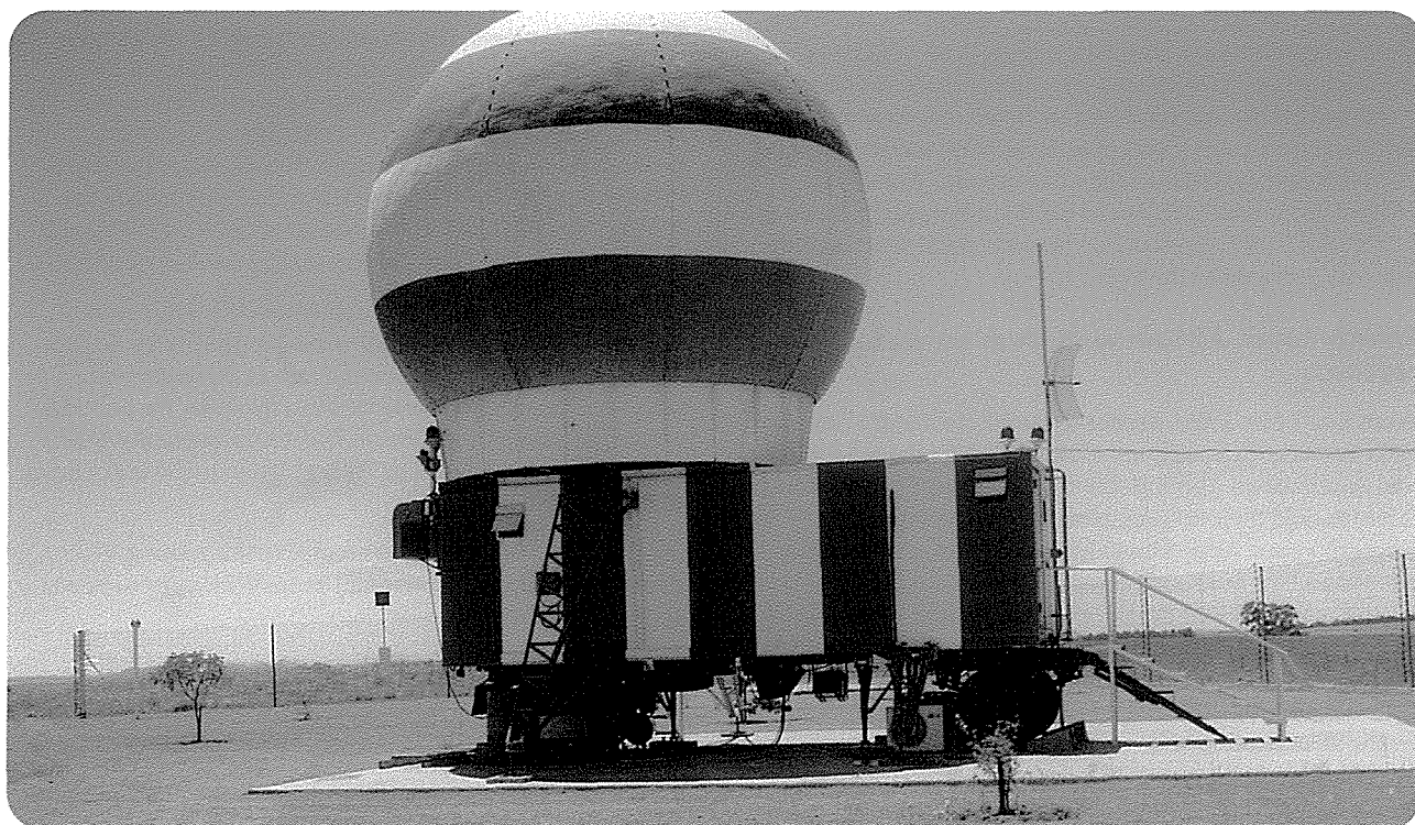
The WRC's MRL-5 research radar, used by the Weather Bureau to develop techniques for real-time monitoring and mapping of rainfall.
