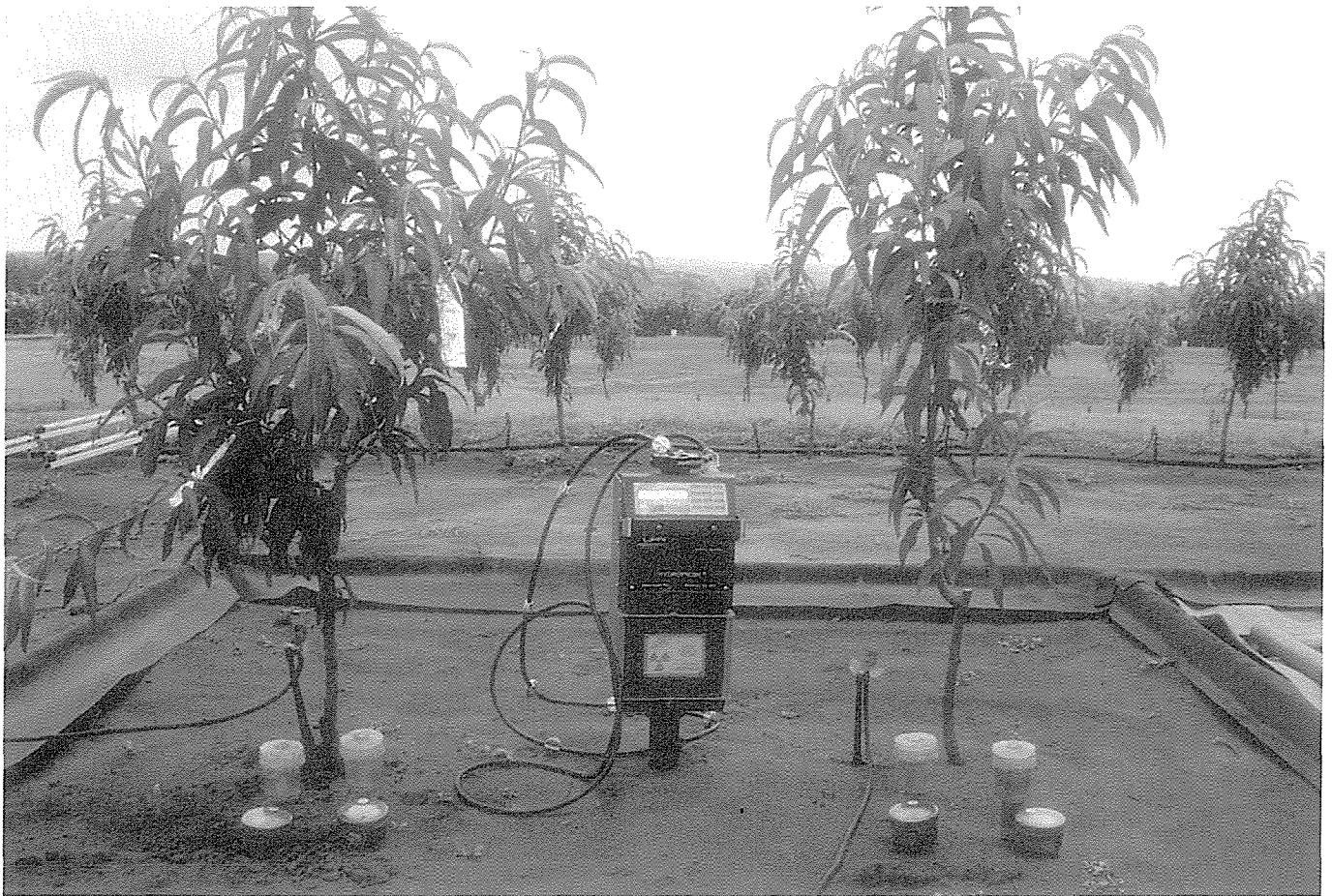
Monitoring the soil-water balance of deciduous fruit trees with a neutron hydroprobe and tensiometers in a weighing lysimeter.
