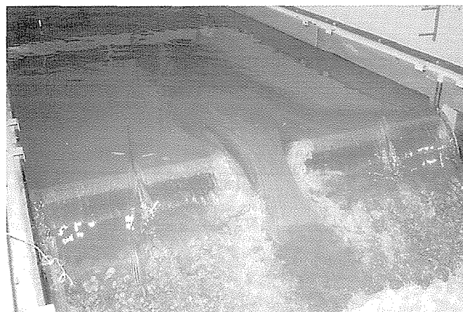
With reference to Project No 442, the above photographs illustrate models investigating flow measurement utilising the sluicing flume in combination with an existing weir.
