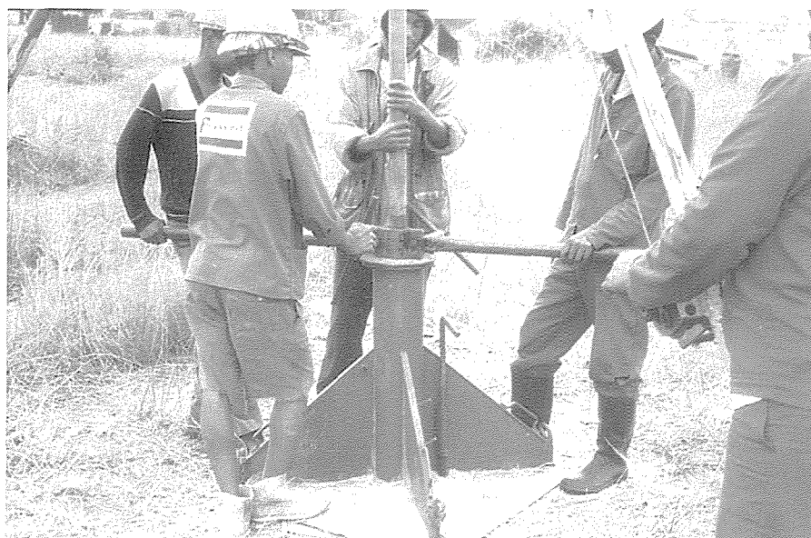
Hand-augering of shallow boreholes, Ubombo Region, KwaZulu-Natal. Hand-augered boreholes serve to identify the nature of the saturated alluvium prior to the sinking of hand-dug wells and will later serve as a pilot study for shallow screened boreholes to supply the communities.
