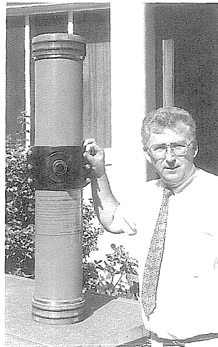
Mr Siegfried Domröse of the Institute for Polymer Science demonstrating a large membrane module.
