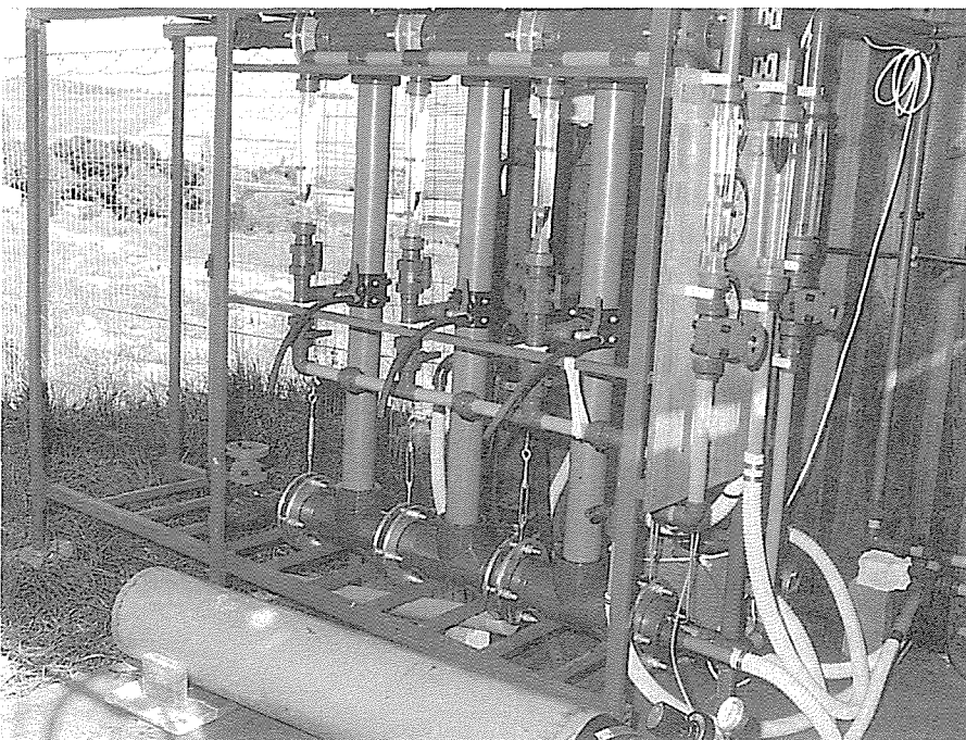
Cross-flow microfiltration unit for rural water supply.
