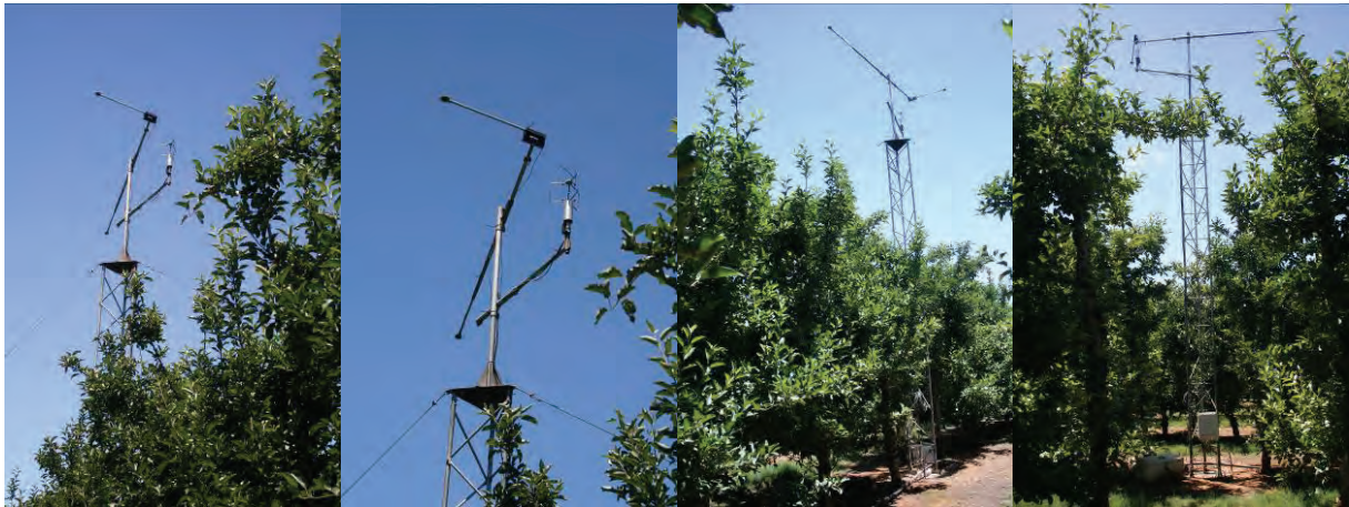
Figure 4 Instrumentation installed at the apple orchard, the sonic anemometer and net radiometers clearly visible above the apple trees
