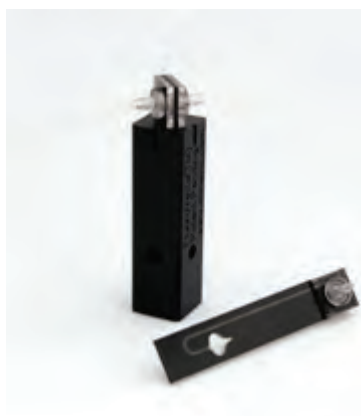
Figure 3: Short path length Fluorovette disposable flow cells as an alternative to more expensive glass and quartz units
