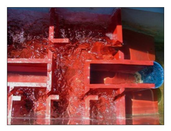
Plate A.1: Twin Channel Vertical Slot Fishway experimental scale model.
