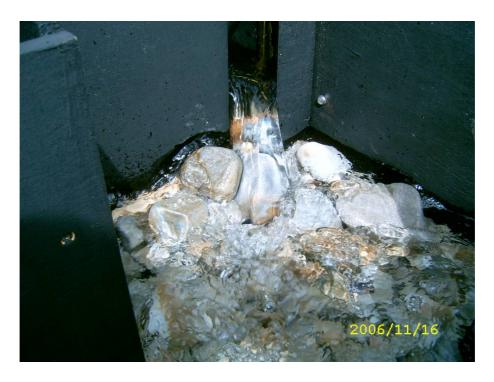
Plate 15: Low flow through wide slot
