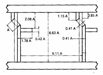
Figure 1: Recommended layout of vertical slot fishway (From Lariner et al., 2002).
