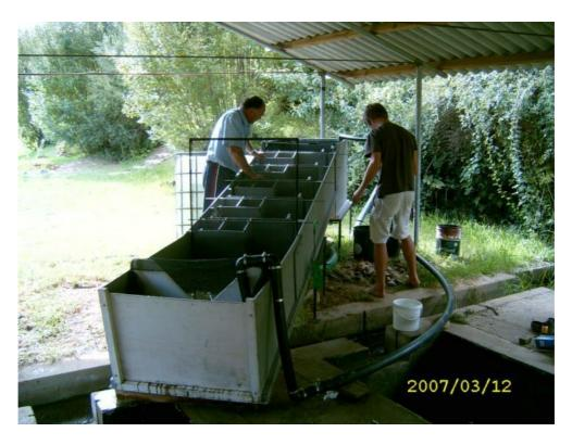
Plate C.1: Portable model of a Twin Channel Vertical Slot Fishway tests at model used for Jonkershoek
