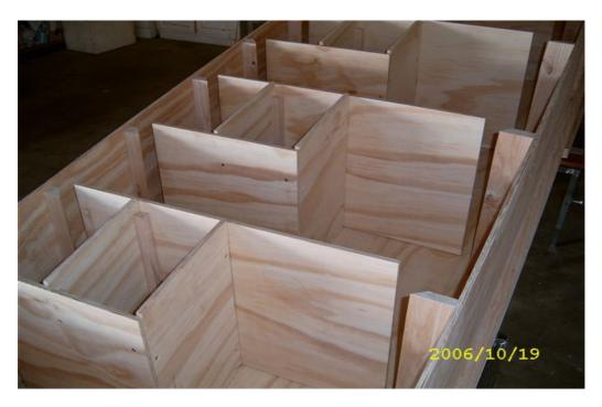
Plate 6: Baffle Detail
