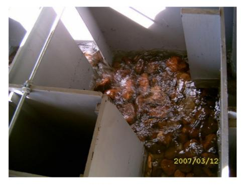
Plate 21: Single layer of rock was placed on the bottom of model.
