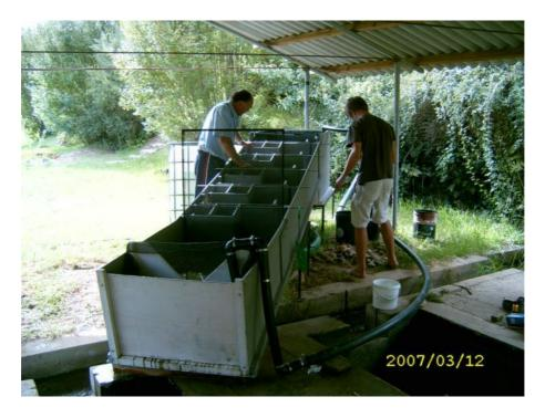
Plate 20: Portable model of a Twin Channel Vertical Slot Fishway model used for tests at Jonkershoek
