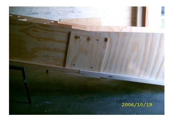
Plate 9: Connection between top tank and channel
