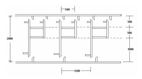
Figure 2: Plan view of proposed Twin Channel Vertical Slot Fishway
