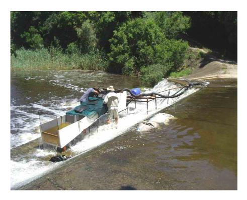
**Plate B.3:** Fishway during a trial run with covering net over channel and siphon pipes
