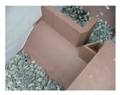
Plate 3: Downstream face of Ogee spillway
