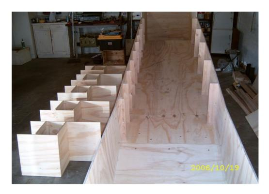
Plate 10: Channel with baffles removed
