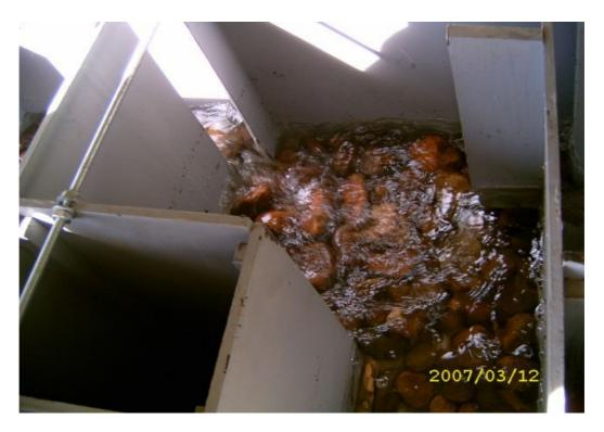
Plate C.3: Single layer of rock was placed on the bottom of model.
