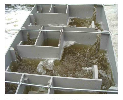
Plate B.6: Fishway channel at high flow (18.9 ℓ/sc)
