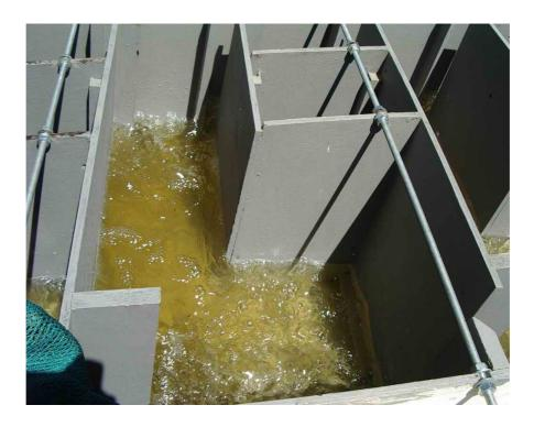
Plate B.4: Fishway channel without stones on bottom at ca 8 ℓ/sec discharge
