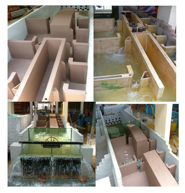
Plate A.2: Various views of the full-scale Twin Channel Vertical Slot Fishway model.
