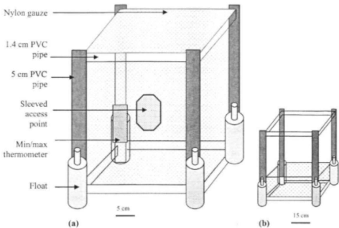
**Figure 5.1** Floating field-cages used to monitor *Stenopelmus rufinasus* impact on *Azolla filiculoides*. (a) Cage design with full gauze covering ('treatment' and 'closed control'); (b) Cage design with 20cm gauze skirt ('open control').
