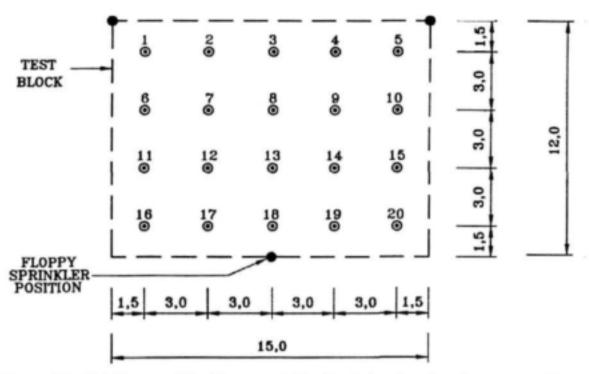
Figure 3.3: Field layout of the Floppy sprinkler block showing the raingauge positions
