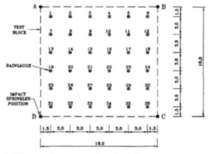
Figure 3.2: Field layout of impact sprinkler blocks showing raingauge positions
