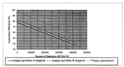
Figure 4.5: Plot of the Regression Curves of Application Efficiency at Silverton as a function of the square of radiation
