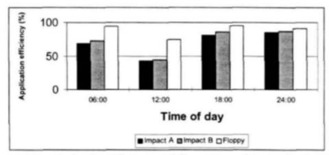
Figure 4.4: Mean Application Efficiency at different times of the day for the Silverton trials for the dragline impact sprinklers and the Floppy permanent system
