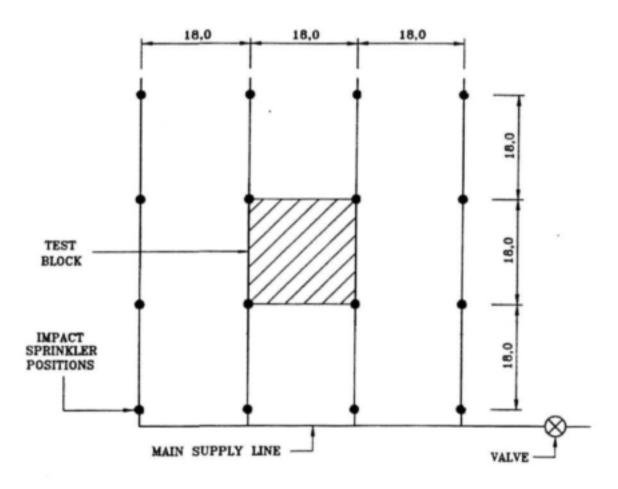
Figure 5.1: Layout of permanent set of impact sprinklers
