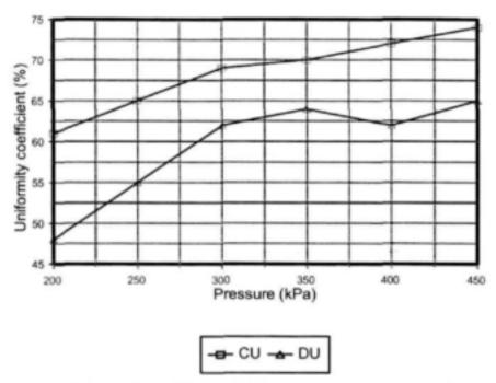
Figure 5.9: Relationship of CU and DU to operating pressure of impact sprinkler B (from laboratory results)
