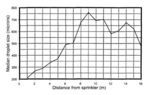
Figure 5.4: Particle size distribution curve with distance from the sprinkler for the impact sprinkler A (Philpott, 1999)
