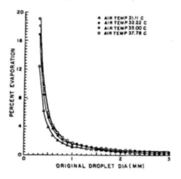
Figure 5.2: Evaporation vs. droplet diameter, no wind (Edling, 1985)
