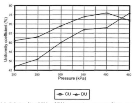
Figure 5.8: Relationship of CU and DU to operating pressure of impact sprinkler A (from laboratory results)
