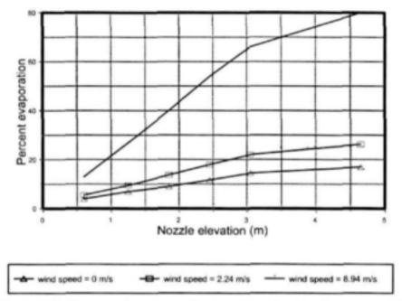
Figure 5.3: Evaporation vs. nozzle elevation, droplet diameter = 0.3 mm (from Edling, 1985)
