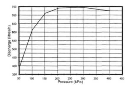
Figure 5.7: Delivery-pressure relationship for the Floppy sprinkler (from laboratory results)
