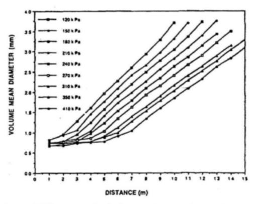
Figure 5.6: Volume means droplet diameters (mm) as a function of distance and pressure for a 4,0 mm circular nozzle (Hills and Gu, 1989)
