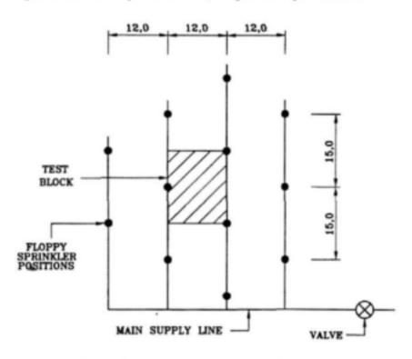
Figure 3.1: Field layout of Floppy sprinkler system
