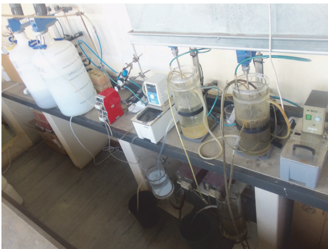
Figure 3.2: Image of the simulated activated sludge wastewater treatment plant
