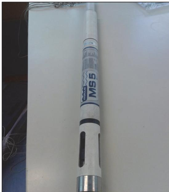
**Figure 4.7: Hydras Multiprobe used to collect online data**
