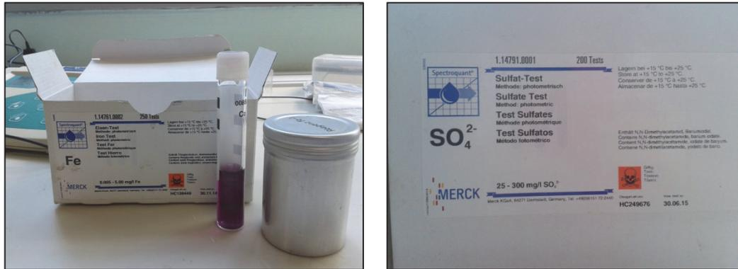
Figure 4.6: Merck iron and sulphate test kits
