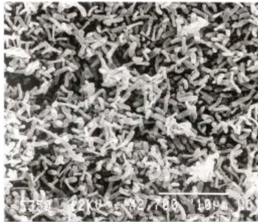
Figure 4.17 Scanning electron micrograph of attached bacterial population from the third section of the reactor that was sampled. A relatively dense, but morphologically uniform bacterial population seems to have developed
