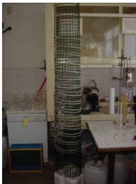
Figure 4.2 Photograph of the Silicone Tubular Reactor laboratory set-up. Silicone tubing was supported on a plastic mesh column
