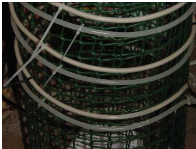
figure 4.5 Photograph of silicone Tubular Fixed Film Reactor showing white biofilm development within the tubing (top tube) compared to a fresh length of silicone tubing attached below each turn for illustrative purposes.
