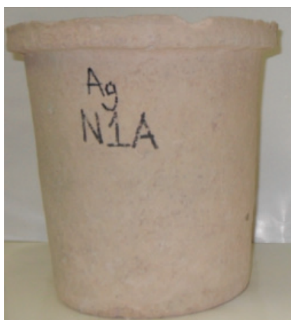
Nanoparticle silver impregnated pots (SIPP-M1) (J5 and J6)
