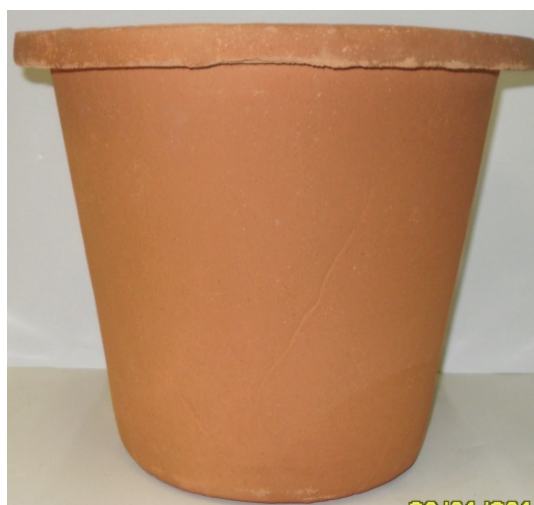
Colloidal silver coated pot (PFP)
