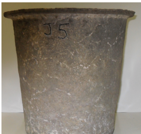
Nanoparticle silver impregnated pots (SIPP-M1) (J5 and J6)
