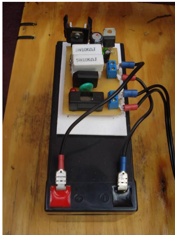
Figure 4.25: Output regulating circuit and storage facility in the form of a 12V battery
