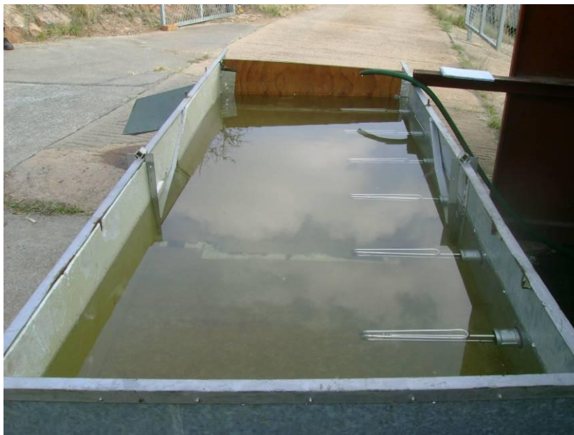
Figure 4.11: Zinc basin with geyser elements used as ballast loads
