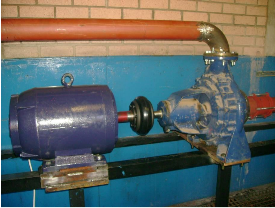
Figure 4.17: Connection between pump-as-turbine and motor
