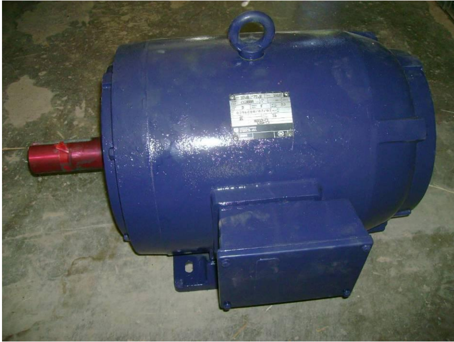
Figure 4.9: Motor from Alstom that is used as a generator
