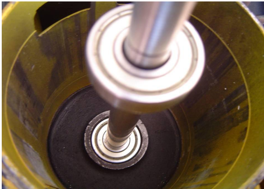
Figure 4.21: The shaft with its bearings on either side of the casing
