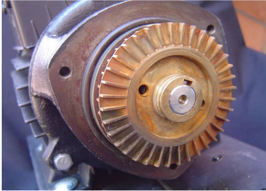
Figure 4.20: The impeller in its casing connected to the shaft
