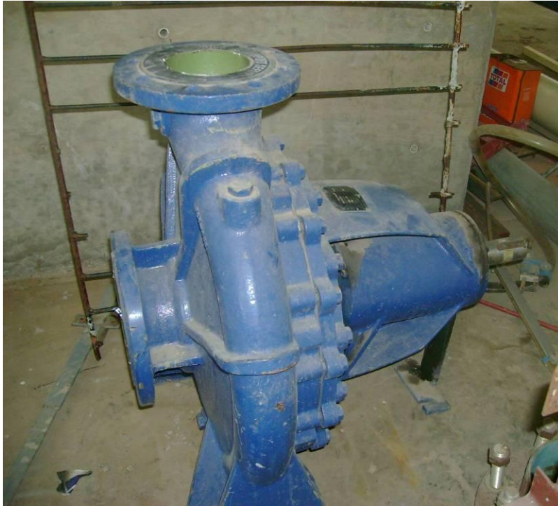
Figure 4.8: Sulzer pump that is used as a turbine(Sulzer AZ 100/400)
