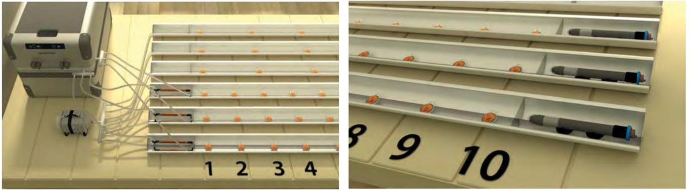
**Figure 3:** Diagram showing experimental setup for estimating thermal preference using thermal gradient tanks, with the cold pole (left) and the warm pole (right).
