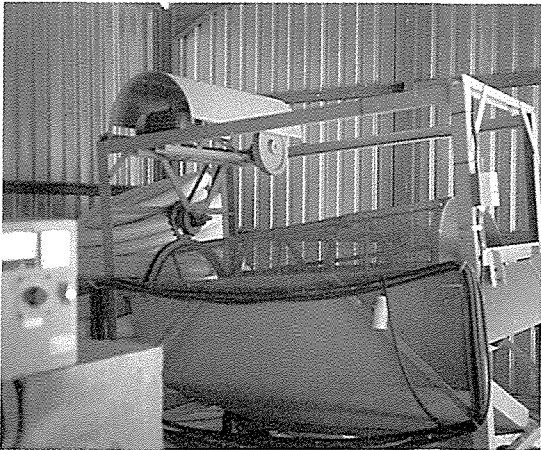
Forced aeration composting of sludge: An effective sludge disinfection and stabilisation process incorporating the use of wood chips which are screened out on completion of the process.
