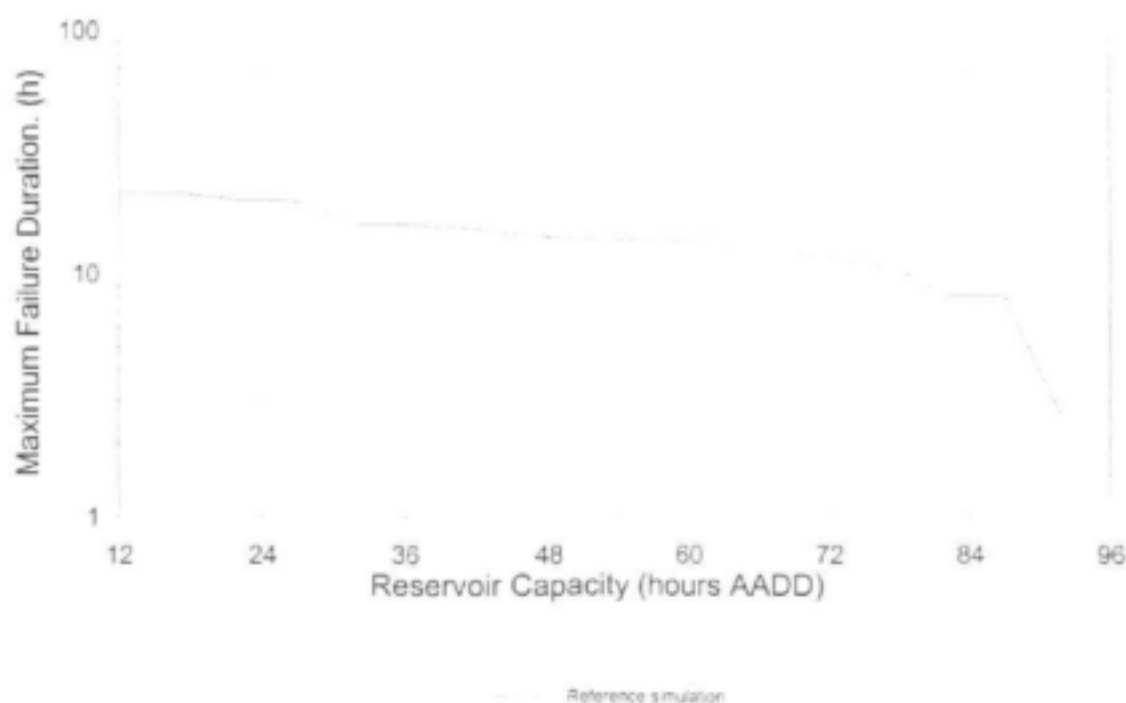
Figure 5.4 Maximum failure duration for a typical Johannesburg reservoir
