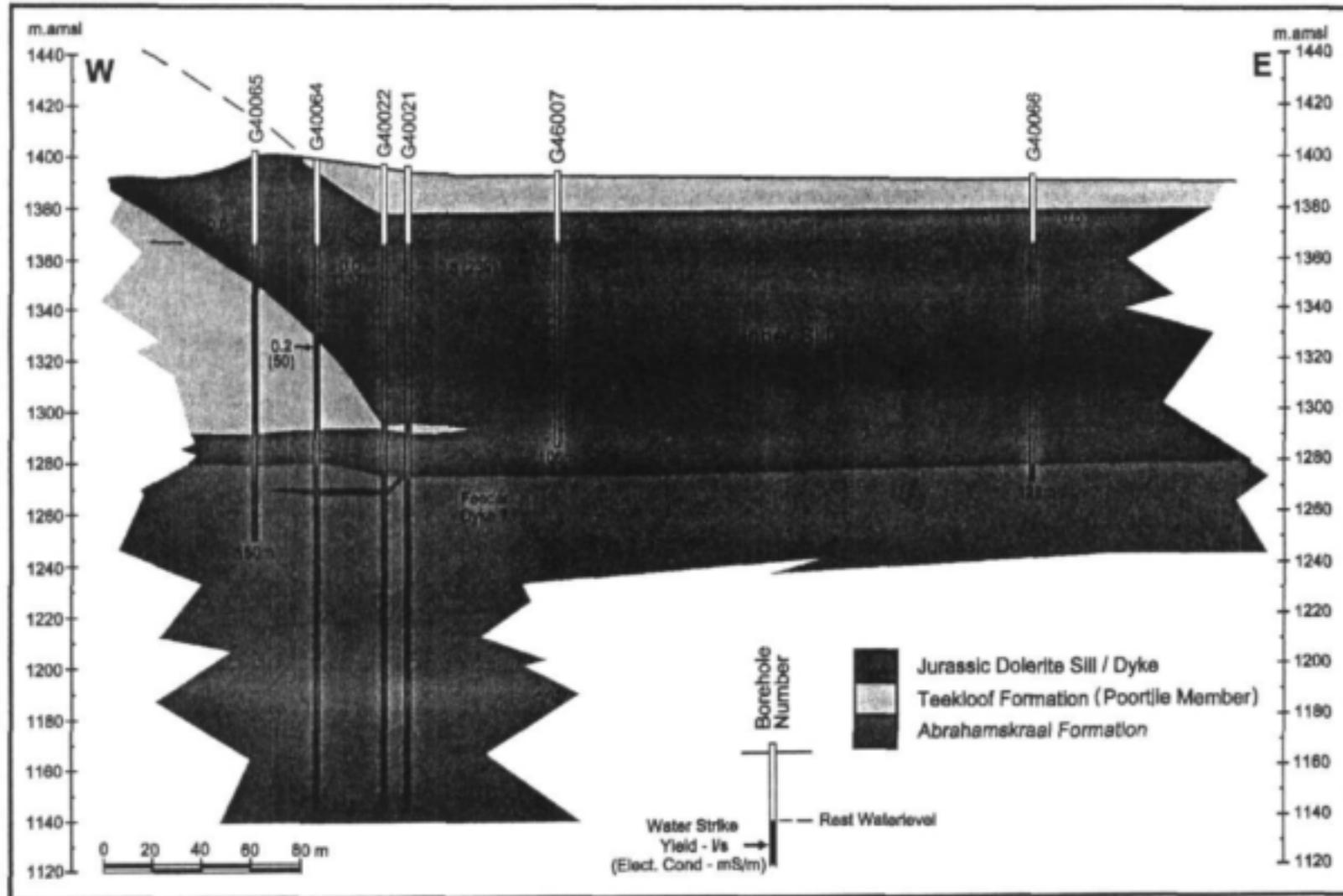
Figure 59: Geohydrological Profile at Exploration Drill Site No. 1
