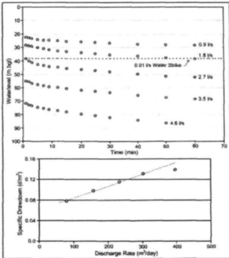
Figure K: Borehole G40199 – Step-Drawdown Test
