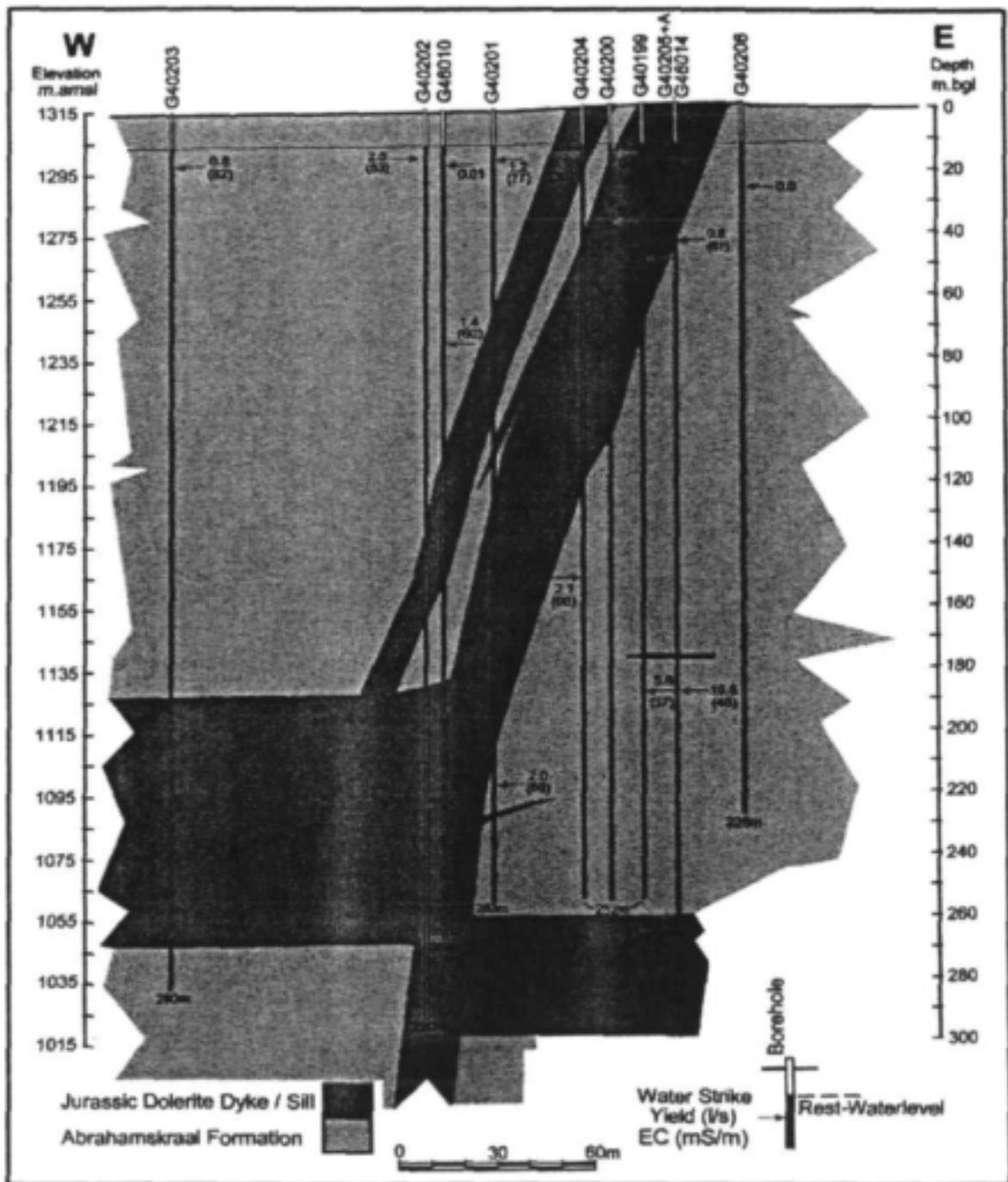
Figure 65: Geohydrological Profile at Exploration Drill Site No. 7
