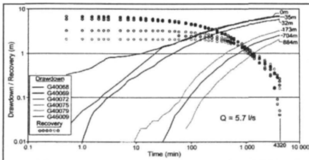
Figure B: Constant Discharge Test of Borehole G40068 – Waterlevel drawdown and Recovery
