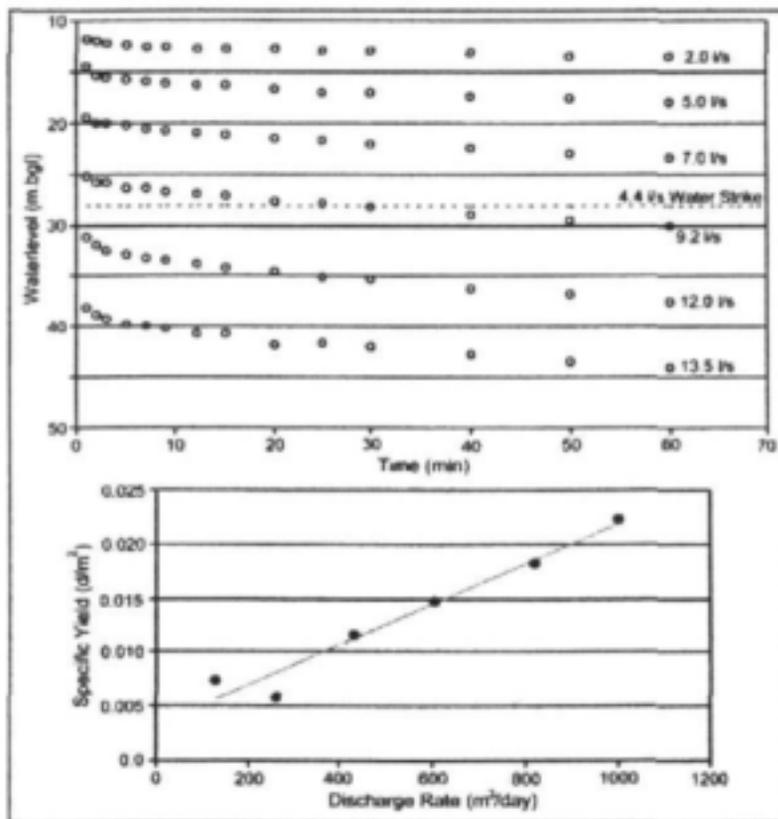
Figure G: Borehole G46005A - Step-Drawdown Test
