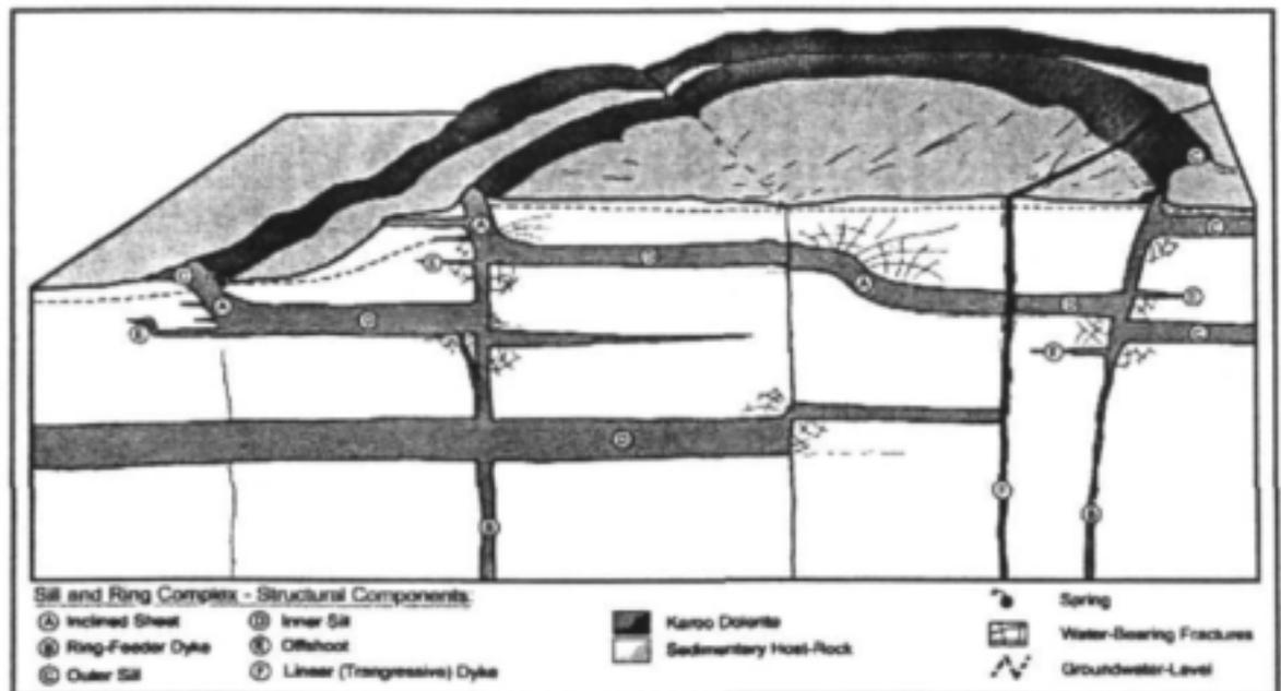
**Figure 70: Schematic Hydro-morphotectonic Model of a Dolerite Sill and Ring Complex**
