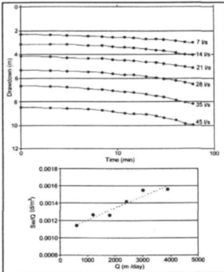
Figure E: Borehole G40082 – Step-Drawdown Test
