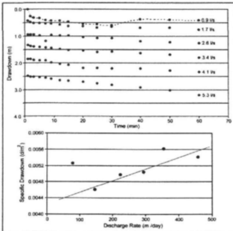
Figure A: Borehole G40068 – Step-Drawdown Test
