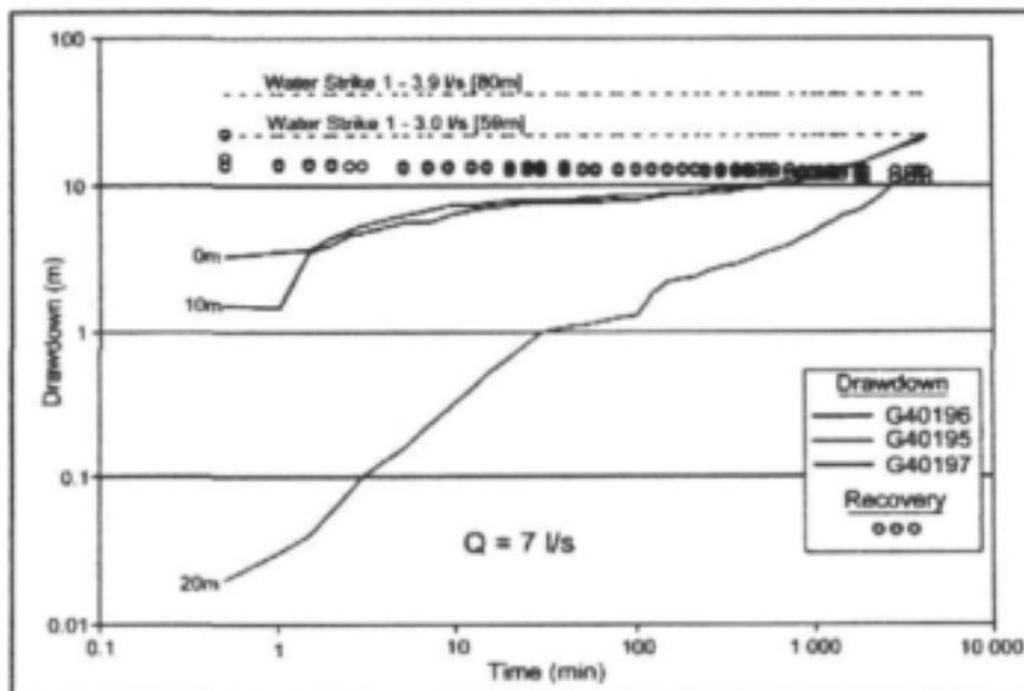
Figure J: Constant Discharge Test of Borehole G40196 – Waterlevel drawdown and Recovery
