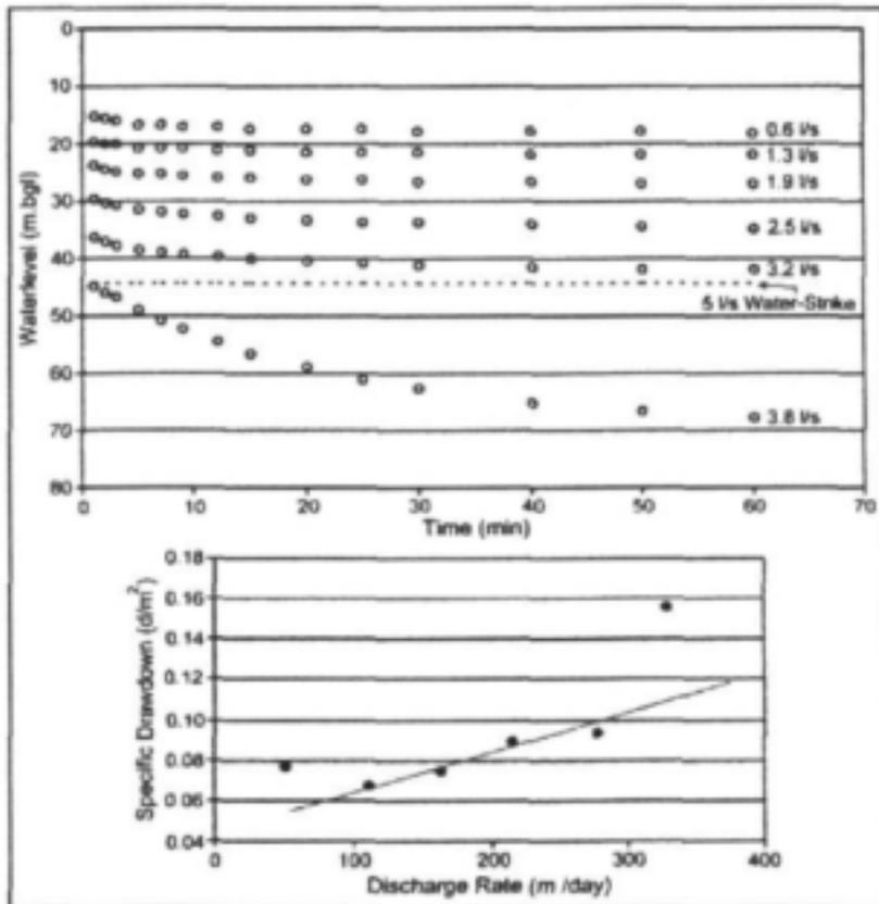
Figure C: Borehole G40078 – Step-Drawdown Test
