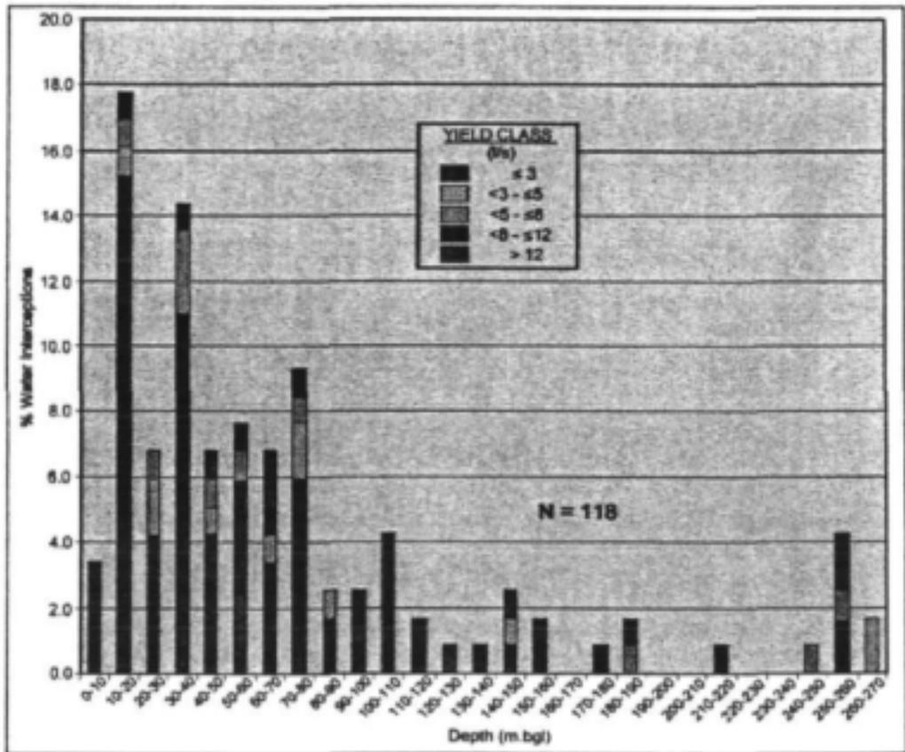
**Figure 69: Histogram showing percentages of water interceptions and relative percentages of drillstem yields per 10m drilling depth intervals below ground surface**
