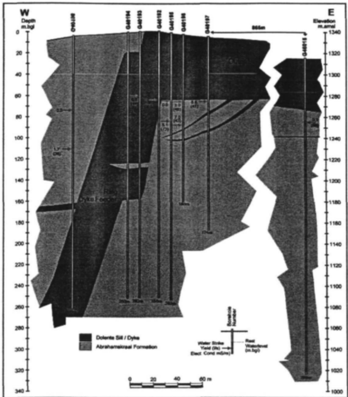
Figure 64: Geohydrological Profile at Exploration Drill Site No. 6
