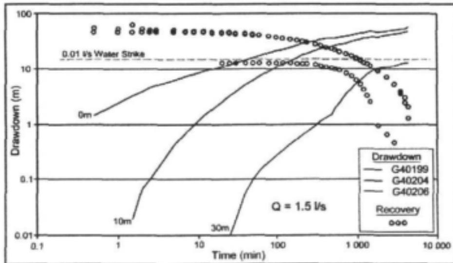
Figure L: Constant Discharge Test of Borehole G40199 – Waterlevel drawdown and Recovery
