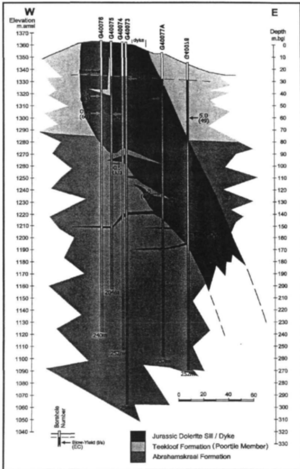
**Figure 61: Geohydrological Profile at Exploration Drill Site No. 3**
