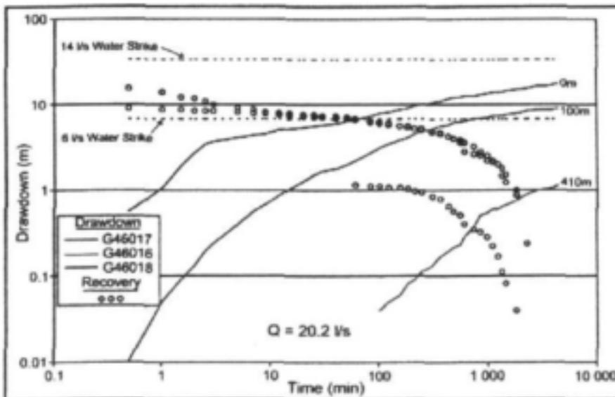
Figure N: Constant Discharge Test of Borehole G46017 - Waterlevel drawdown and Recovery
