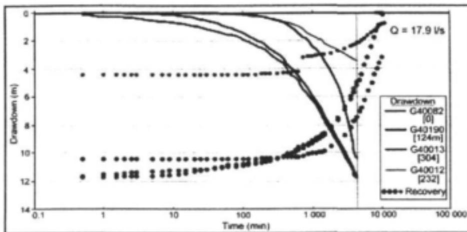
Figure F: Constant Discharge Test of Borehole G40082 – Waterlevel drawdown and Recovery
