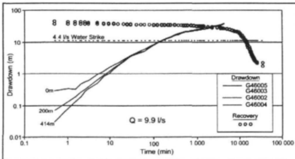
Figure H: Constant Discharge Test of Borehole G46005A - Waterlevel drawdown and Recovery
