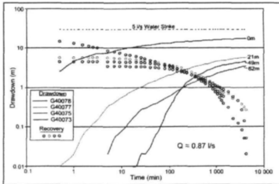
Figure D: Constant Discharge Test of Borehole G40078 – Waterlevel drawdown and Recovery
