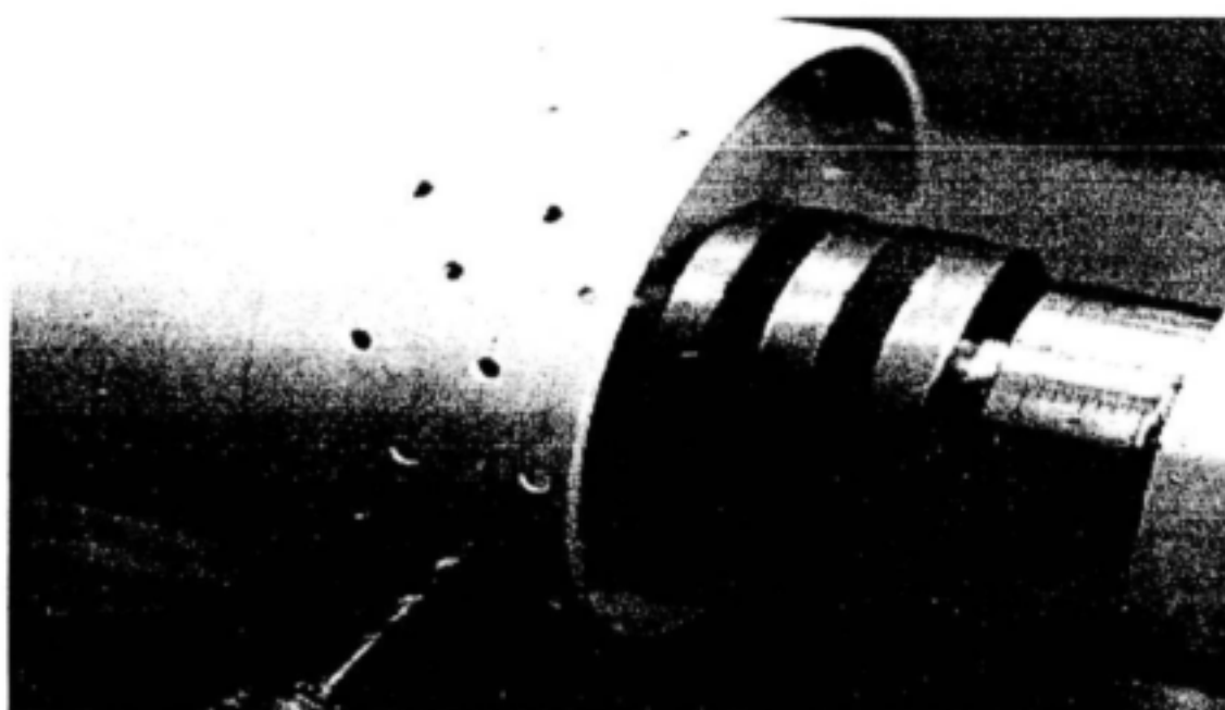
FIGURE 3.4 SHROUD DETAIL WITH FOUR ROWS OF KEY-IN HOLES ARRANGED IN A STAGGERED PATTERN
