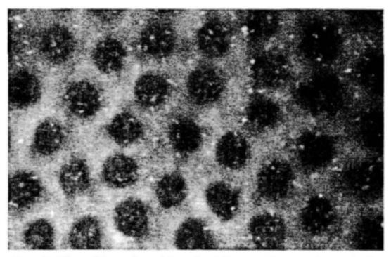
Figure 28. View of the surface of the polysulphone capillary membrane after inoculation with PAO1 and staining with acridine orange. The image was taken by scanning laser confocal microscope, focusing at various depths inside the voids.
