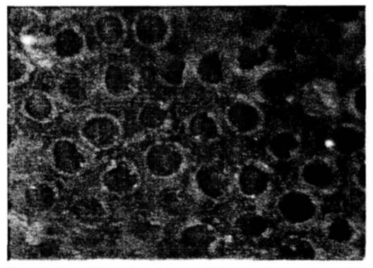
Figure 27. View of the surface of the polysulphone capillary membrane after inoculation with PAO1 and staining with acridine orange. The image was taken by scanning laser confocal microscope, focusing at various depths inside the voids.
