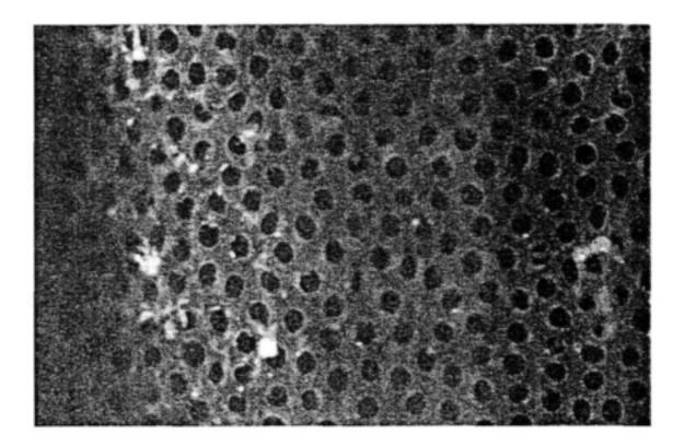
Figure 23. View of the surface of the polysulphone capillary membrane after staining with fluorescein. The image was taken by scanning confocal laser microscope.
