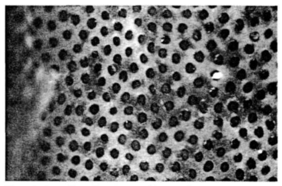
Figure 24. View of the voids in the polysulphone capillary membrane before inoculation with PAO1 and staining with acridine orange. The image was taken by scanning laser confocal microscope, focusing at various depths inside the voids.
