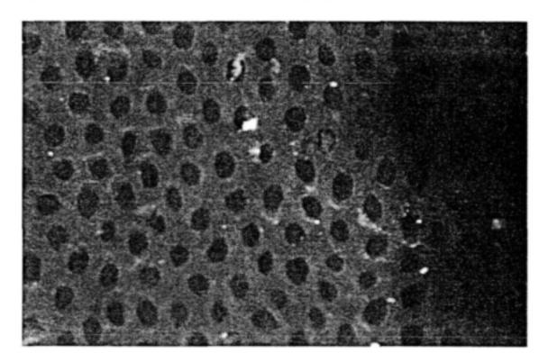
Figure 22. View of the surface of the polysulphone capillary membrane after staining with acridine orange. The image was taken by scanning laser confocal microscope.
