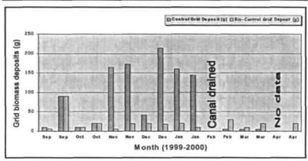
Figure 4.7: The effect of bio-control on the productivity of Cladophora glomerata, based on instream biomass assessments (Experiment 2: 1999-2000).
