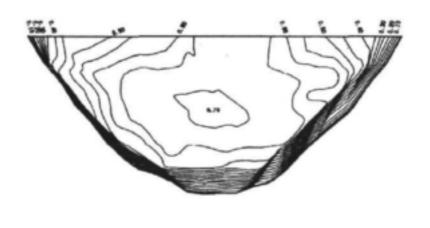
Figure 3.9: Flow distribution patterns at the intake of the Ramah-2 Canal calculated at medium and high flow conditions.
