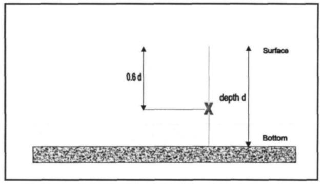
Figure 3.4: Diagrammatic presentation of the Six-tenths Method (One-point Method) for the measurement of flow velocities.
