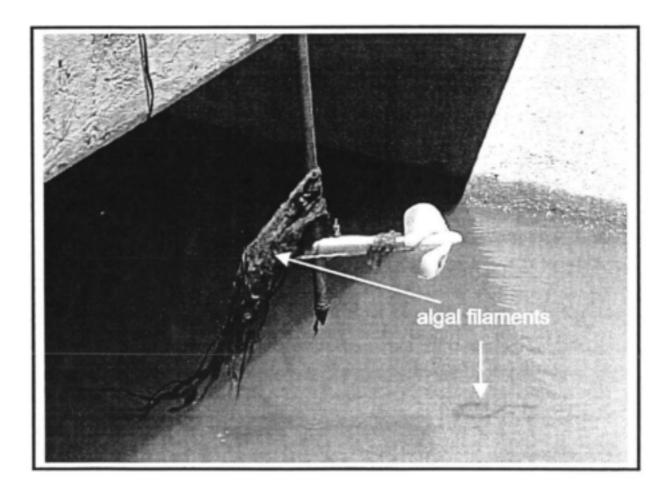
Figure 3.5: Filamentous algae (Cladophora glomerata) tangled around the propeller of a flow meter during flow velocity measurements in the Ramah Canal System.
