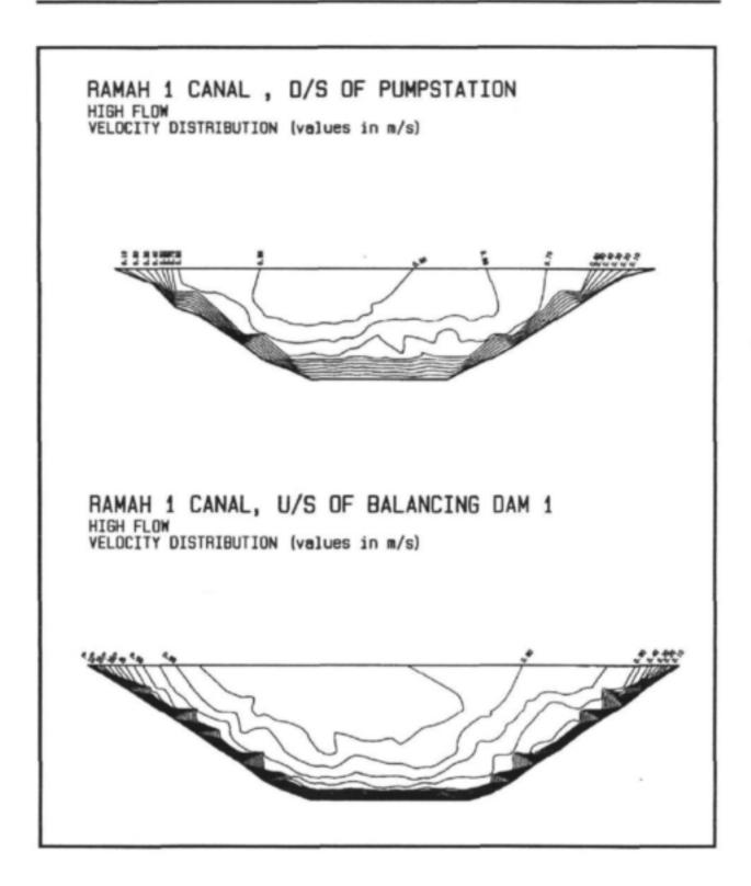
Figure 3.7: Flow distribution patterns at the intake and outflow of the Ramah-1 Canal calculated at high flow conditions.
