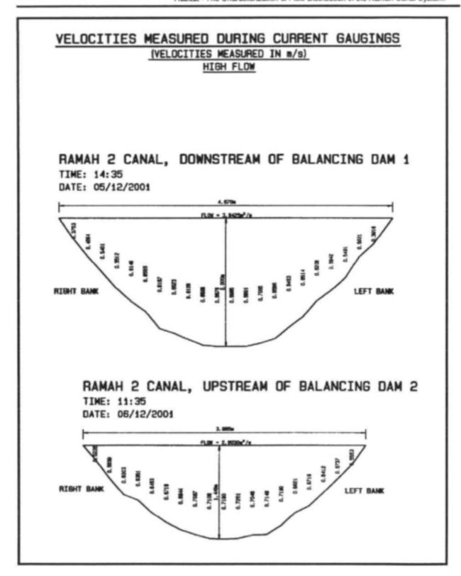
Figure 3.8b: Flow velocities measured at the intake and outflow of the Ramah-2 Canal during medium and high flow conditions.
