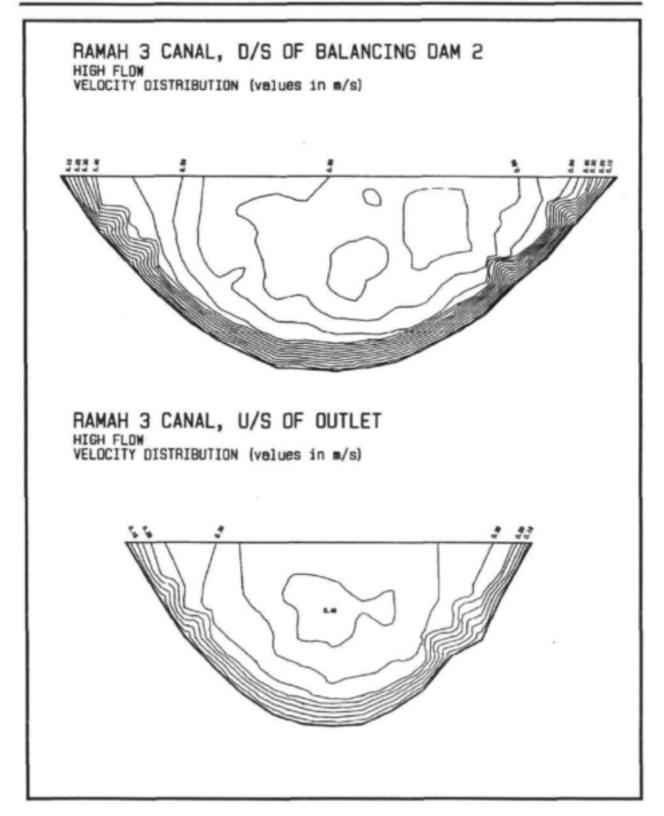
Figure 3.12: Flow distribution patterns at the intake and outflow of the Ramah-3 Canal calculated at high flow conditions.
