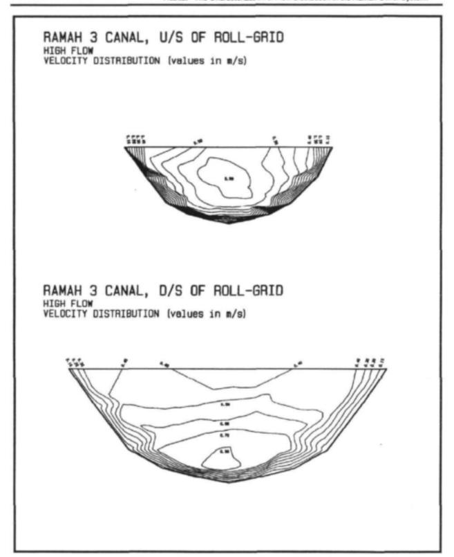
Figure 3.13: Flow distribution patterns at the roll-grid calculated under high flow conditions.
