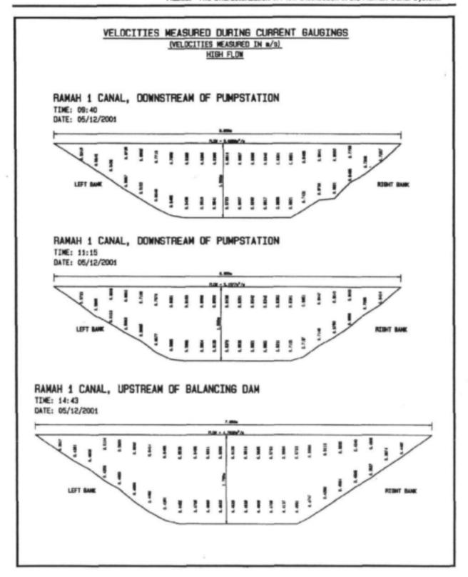
Figure 3.6b: Flow velocities measured at the intake and outflow of the Ramah-1 Canal during medium and high flow conditions.
