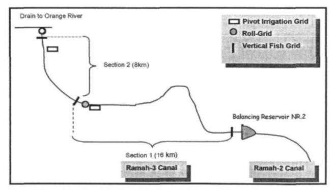
Figure 4.2: Experimental outlay of the Ramah-3 Canal into two sections, separated from each other by vertical fish grids.
