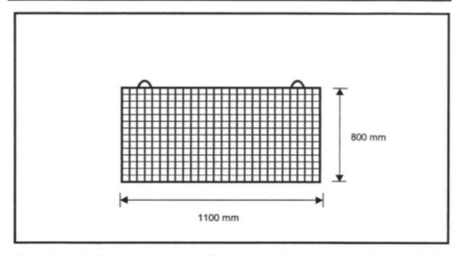
Figure 4.4: A diagrammatic presentation of a standard pivot abstraction grid in the Ramah-3 Canal.
