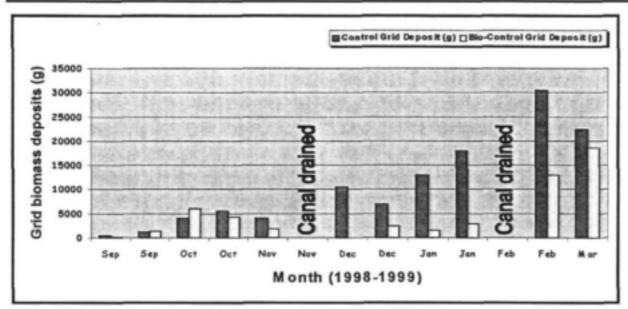
Figure 4.6: The effect of bio-control on the productivity of *Cladophora glomerata*, based on irrigation grid yields (Experiment 1: 1998-1999).
