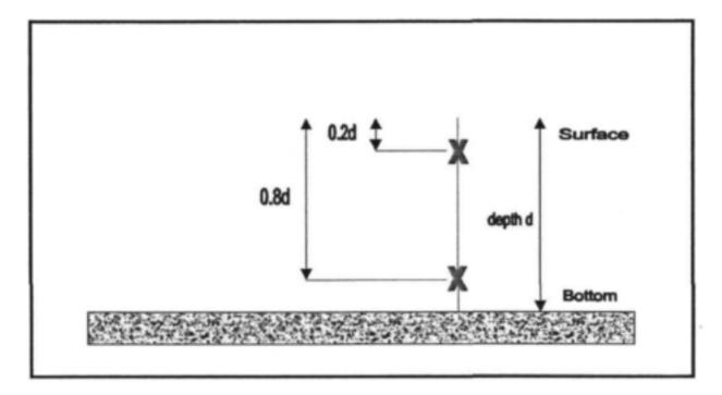
Figure 3.3: Diagrammatic presentation of the Two-point Method for the measurement of flow velocities.
