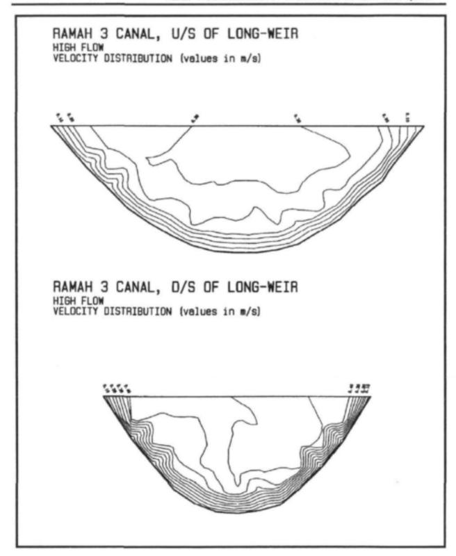
Figure 3.14: Flow distribution patterns at the long-weir in the Ramah-3 Canal calculated at high flow conditions.
