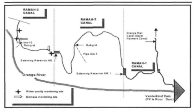
Figure 4.1: A diagrammatic presentation of the Ramah Canal System of the Orange-Riet River Government Water Scheme.
