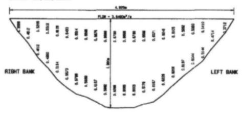
Figure 3.8a: Flow velocities measured at the intake and outflow of the Ramah-2 Canal during medium and high flow conditions.
