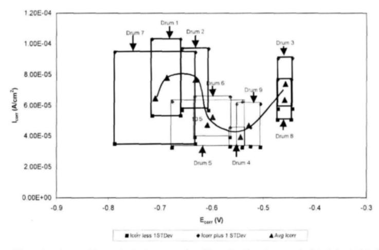
Figure 5.7 I<sub>corr</sub> and E<sub>corr</sub> values from rapid scanning tests representing different treatments grouped within 1 standard deviation below and above the average values and shown with a trend line.
