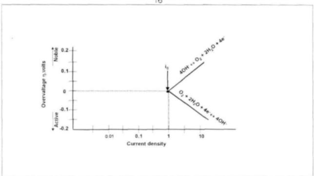
Figure 2.4 Activation-polarization curve of an oxygen electrode
