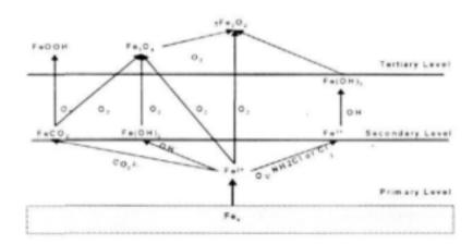
Figure 2.1 Anodic reaction pathways for iron in contact with neutral to alkaline water (Adapted from Loewenthal et al., 1986)
