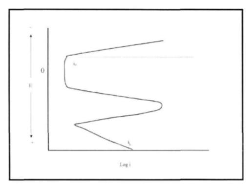
Figure 2.7 Passivation of mild steel at different applied potentials (redrawn from Fontana (1987))
