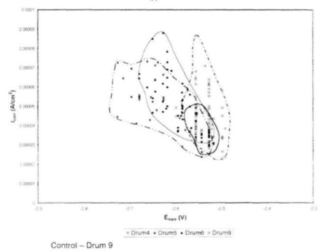
Figure 5.5 Clustered data of measured current (I<sub>corr</sub>) versus potential (E<sub>corr</sub>) in rapid scanning tests in water containing different silicate concentrations compared with a control without any additives.
