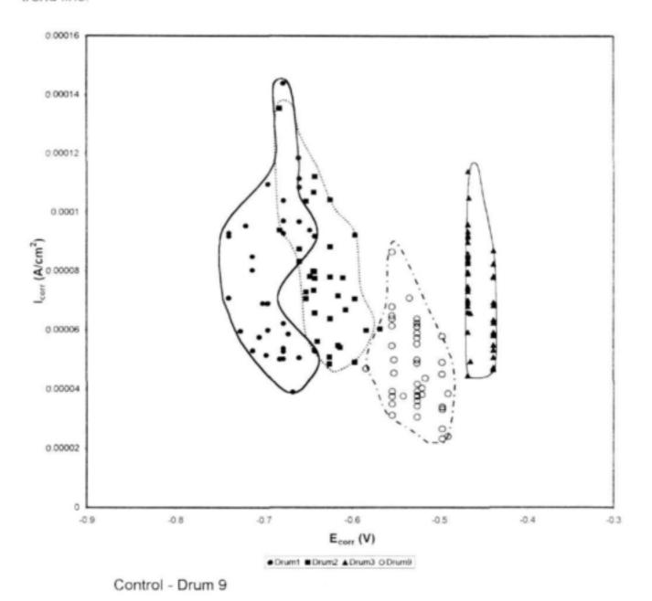
Figure 5.4 Clustered data of measured current (I<sub>corr</sub>) versus potential (E<sub>corr</sub>) in rapid scanning tests in water containing different monochloramine concentrations compared with a control without any additives.
