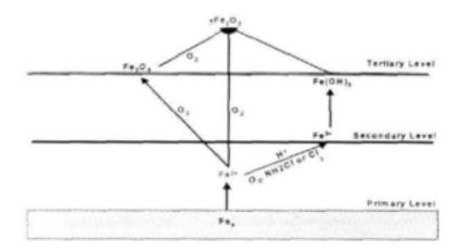
Figure 2.2 Anodic reaction pathways of iron under acidic conditions (Adapted from Loewenthal et al., 1986)
