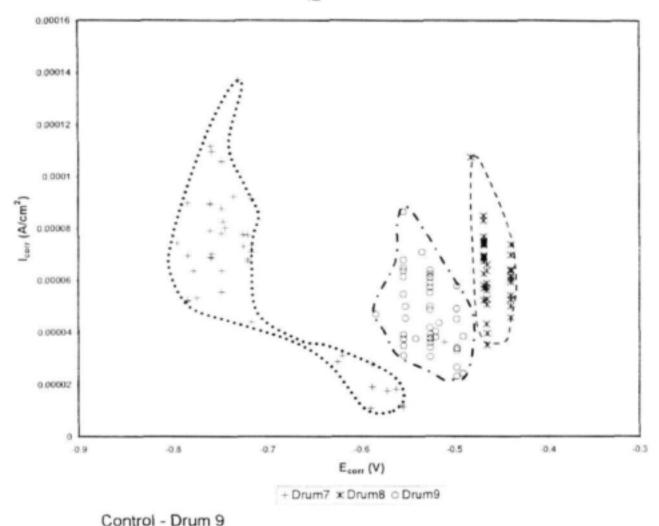
Figure 5.6 Clustered data of measured current (I<sub>corr</sub>) versus potential (E<sub>corr</sub>) in rapid scanning tests in water containing mixtures of monochloramine and silicate at different concentrations compared with a control without any additives.
