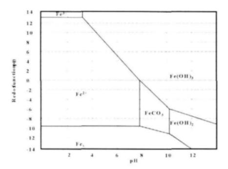
Figure 2.3 pe-pH diagram for metastable equilibrium of the iron-carbonate-water system. Fe<sub>T</sub> = 10<sup>-5</sup> moles/t, C<sub>T</sub> = 10<sup>-3</sup> moles/t and temperature 25 °C. (Redrawn from Loewenthal et al., 1986).
