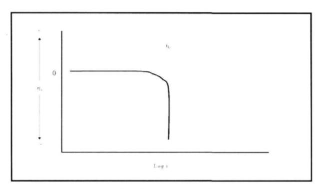
Figure 2.5 Concentration polarization curve for a reduction process (redrawn from Fontana (1987)
