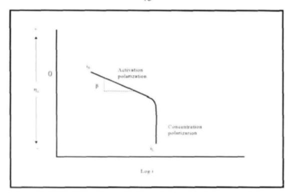
Figure 2.6 Combined polarization curve for activation and concentration polarization for a reduction process (redrawn from Fontana (1987)
