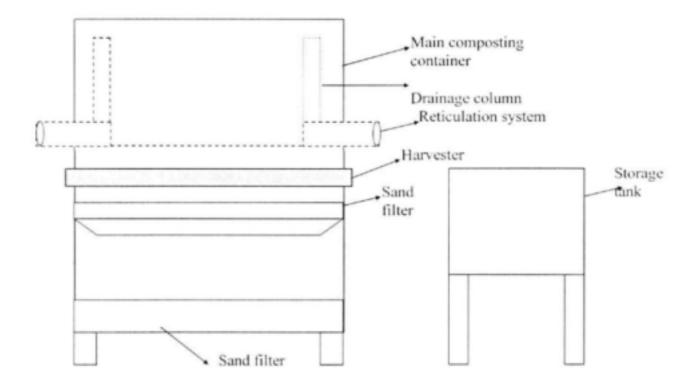
Figure 6.2 Schematic drawing of pilot-plant - View from the top
