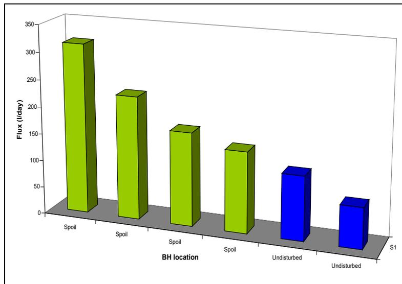
**Fig. 6.14: Groundwater fluxes in rehabilitated mine pits and undisturbed geology at a coalmine.**
