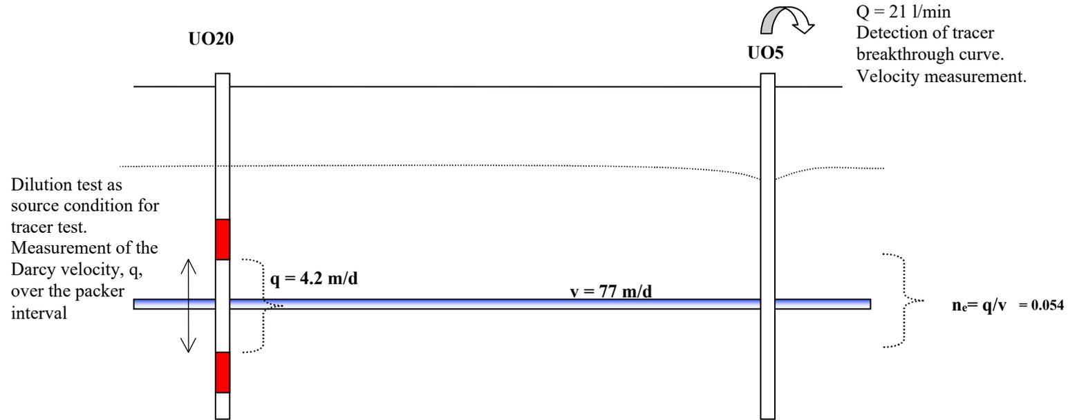
It was found that the peak of the tracer breakthrough does not represent the mean adjective velocity of the fracture zone, since for the same velocity, the peak of simulated breakthrough curves is displaced in time for different values of longitudinal dispersivity. Therefore, a model was developed to analyse tracer breakthrough curve for pore velocity, longitudinal dispersivity and the aquifer thickness according to equation 4.7 in chapter 4.
