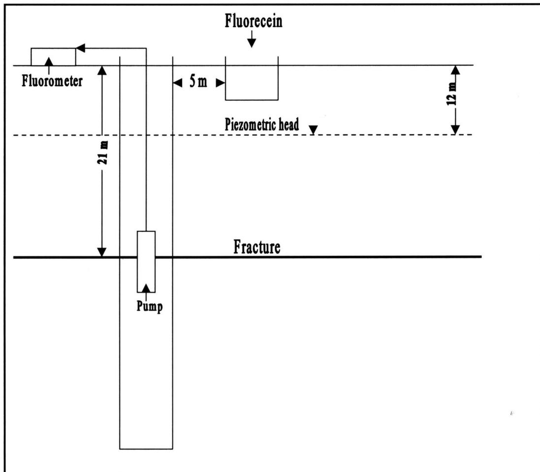
**Figure 6.7: Graphic representation of tracer test setup for the unsaturated zone at the Campus Test Site.**
