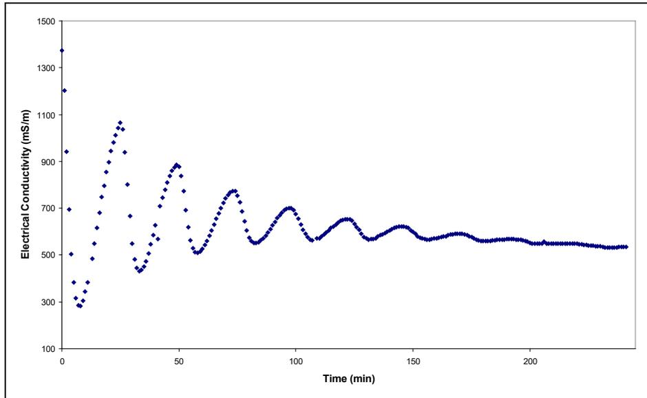
**Fig. 4.5: Measured field curve with spiked tracer injection.**
