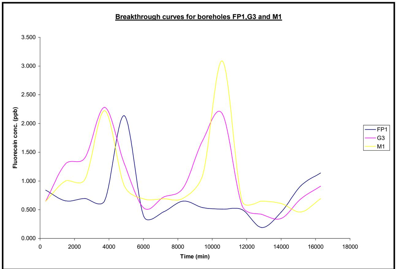
**Figure 6.19: Apparent Fluorecein breakthrough curves in boreholes FP1, G3 and M1 for a period of 1600 minutes.**
