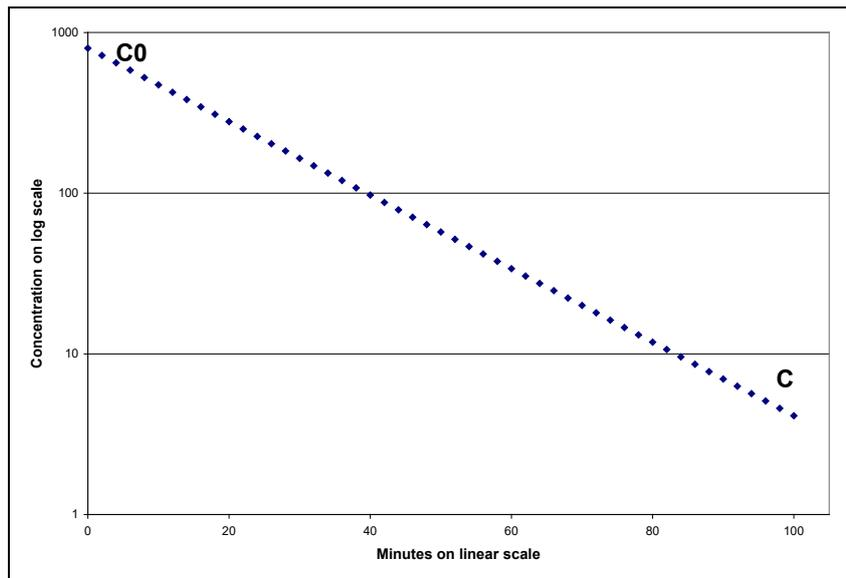
**Fig. 4.1: Illustration of a typical dilution curve**
