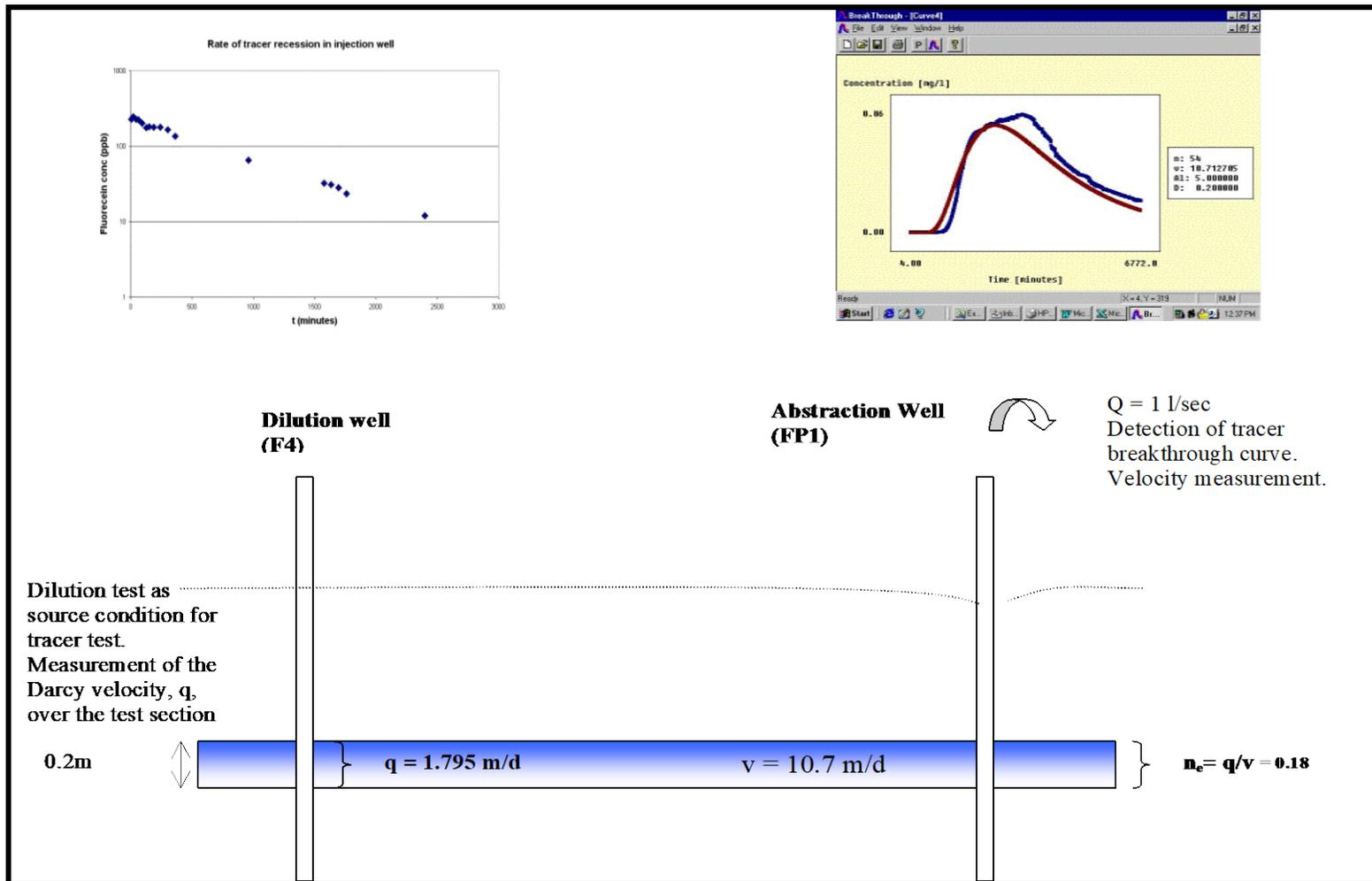
Figure 6.17: Output of analytical model used to determine the groundwater velocity.
