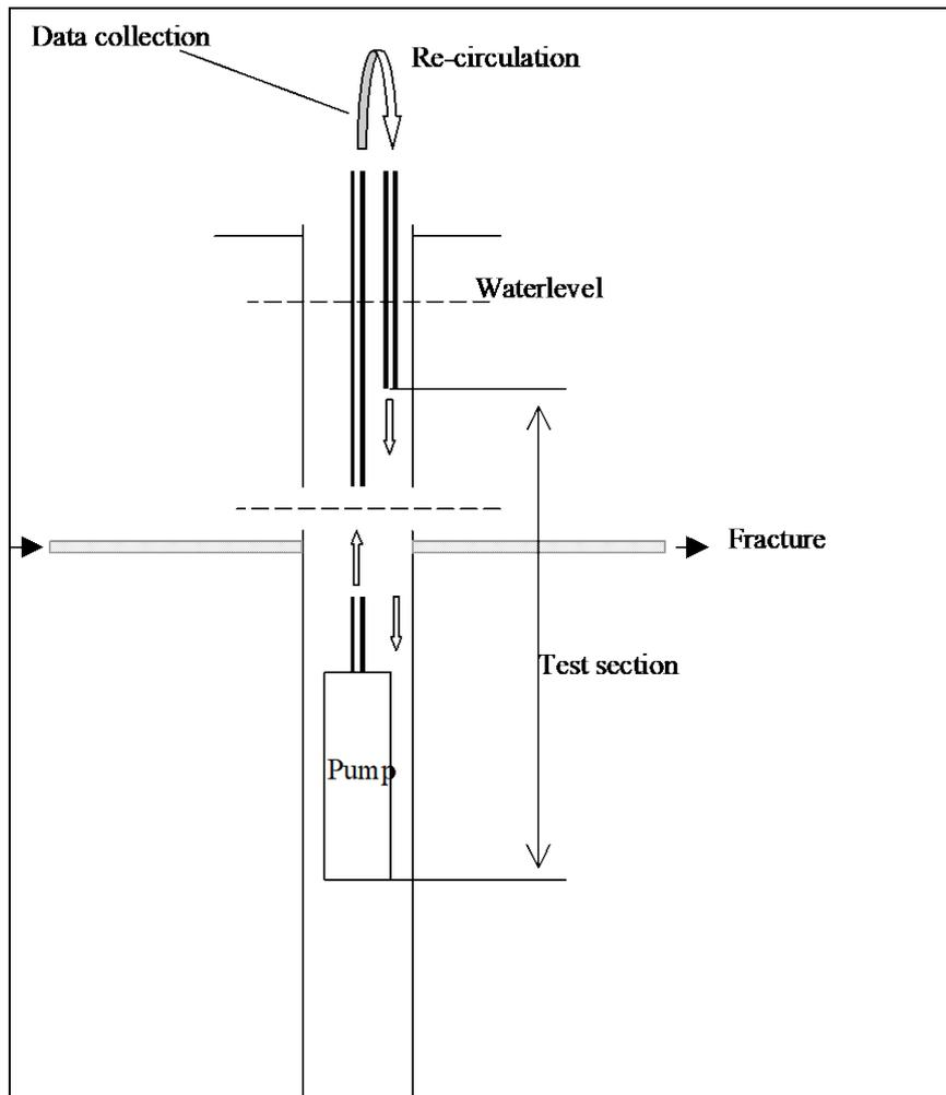
**Fig. 4.4: Illustration of the design of the open well dilution test.**
