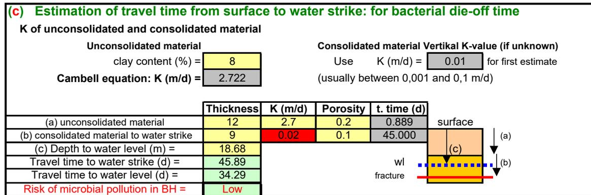
**Figure 6.20: Estimation of travel time from surface to water strike with emphasis on the K-value of 0.02 m/d suggested by the programme BPZONE.**
