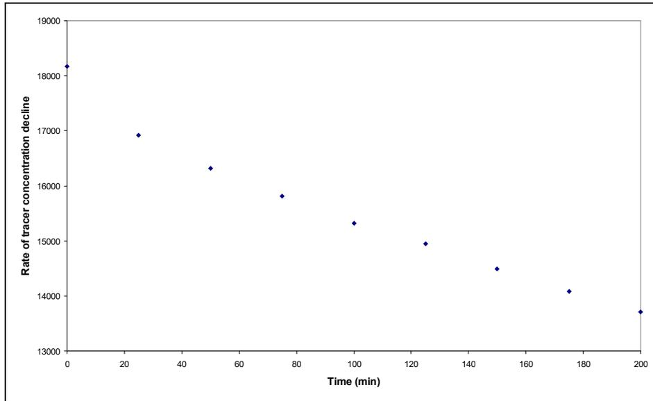
**Fig. 4.6: Integration below each of the measured tracer plumes allows the calculation of the rate of tracer concentration decline due to groundwater advection.**
