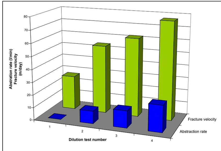
**Fig. 6.5: Groundwater velocities, established at UO20 at different pumping rates in UO5.**
