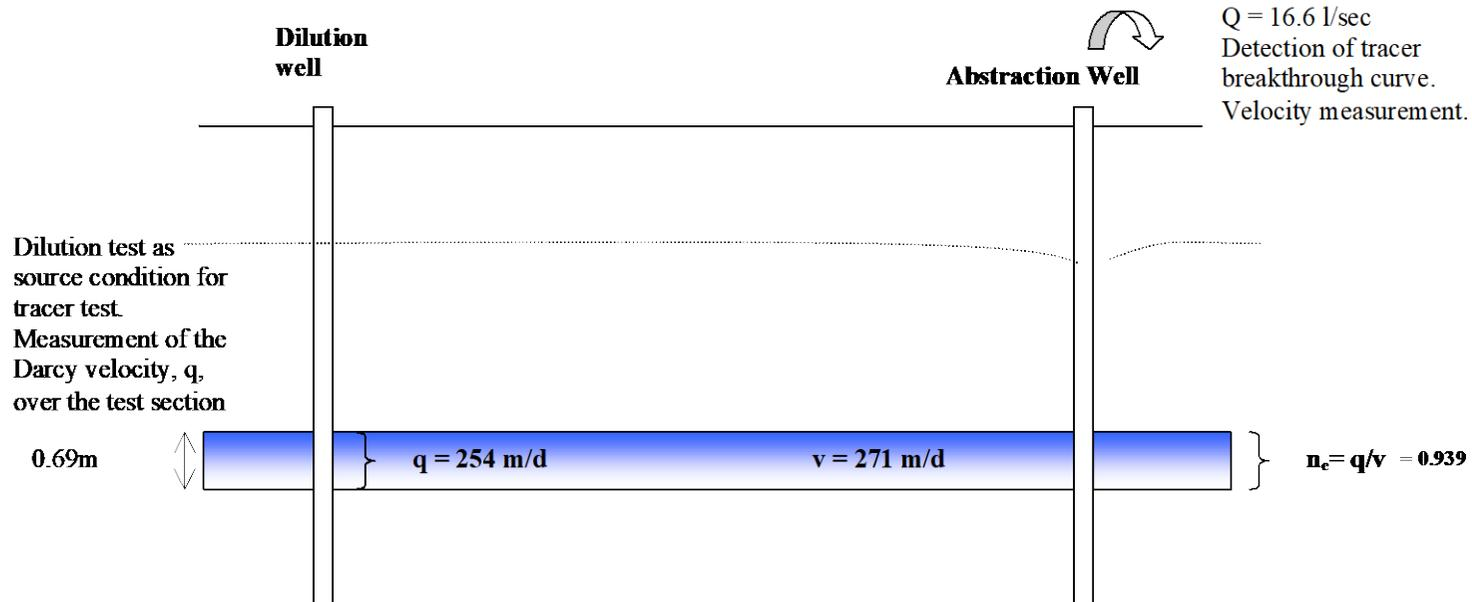
**Figure 6.9: Hartbeesfontein: Kinematic porosity calculation at the scale of the saturated thickness in the borehole.**
