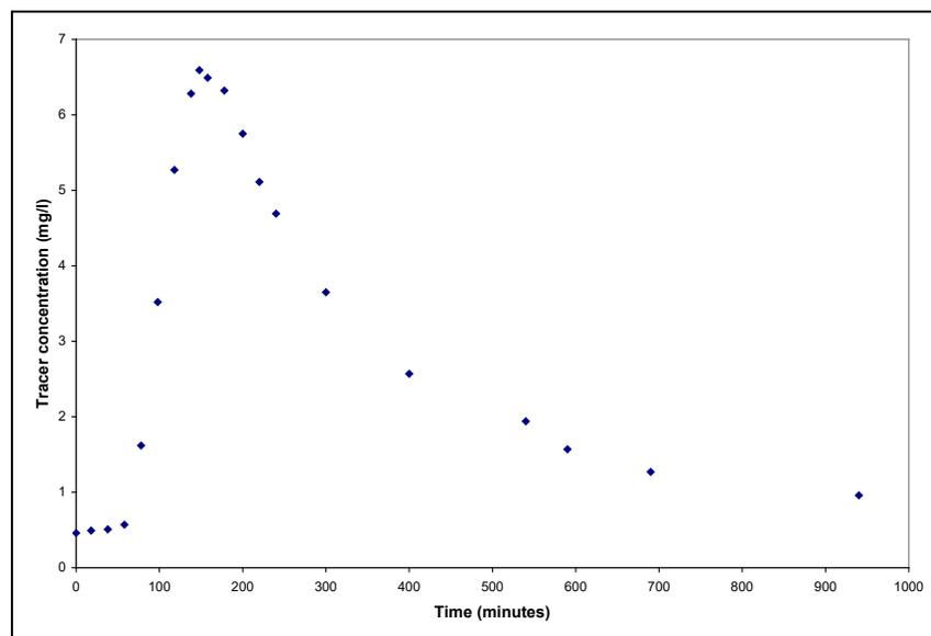
**Fig. 4.2** Illustration of a breakthrough curve detected at the pumping well.
