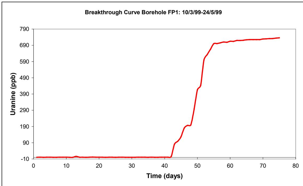
**Figure 6.21: Breakthrough curve measured in borehole FP1 for a period of 75 days.**
