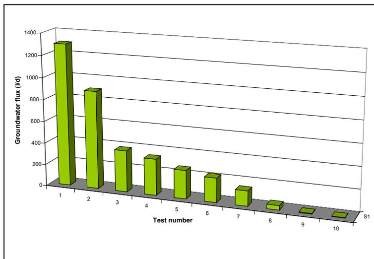
**Fig. 6.13: Dilution tests conducted below a slimes dam indicate much higher fluxes than the rest of the aquifer.**
