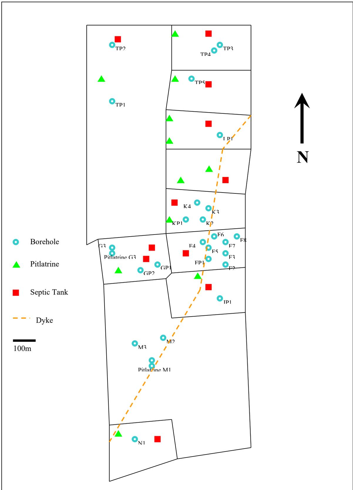
**Figure 6.15: Meadhurst Test Site with the borehole, pitlatrine and septic tank positions.**
