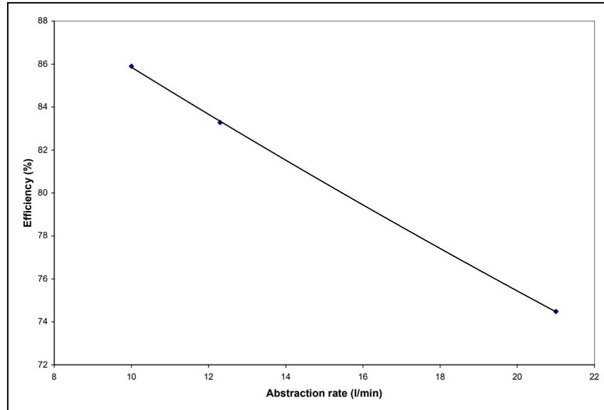
**Fig. 4.3: Well efficiency of UO5 on the Campus Terrain**
