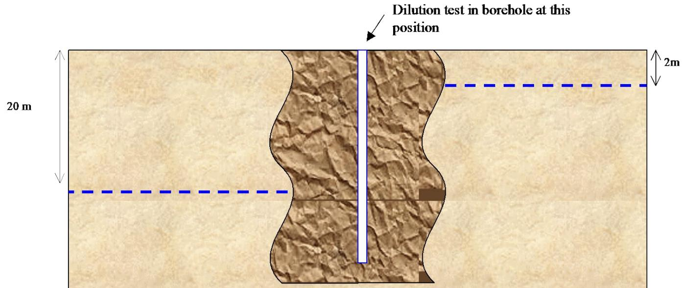
**Figure 6.12: Rustenburg: Establishing the likeliness of groundwater flow along preferred pathways along the side of the dyke.**
