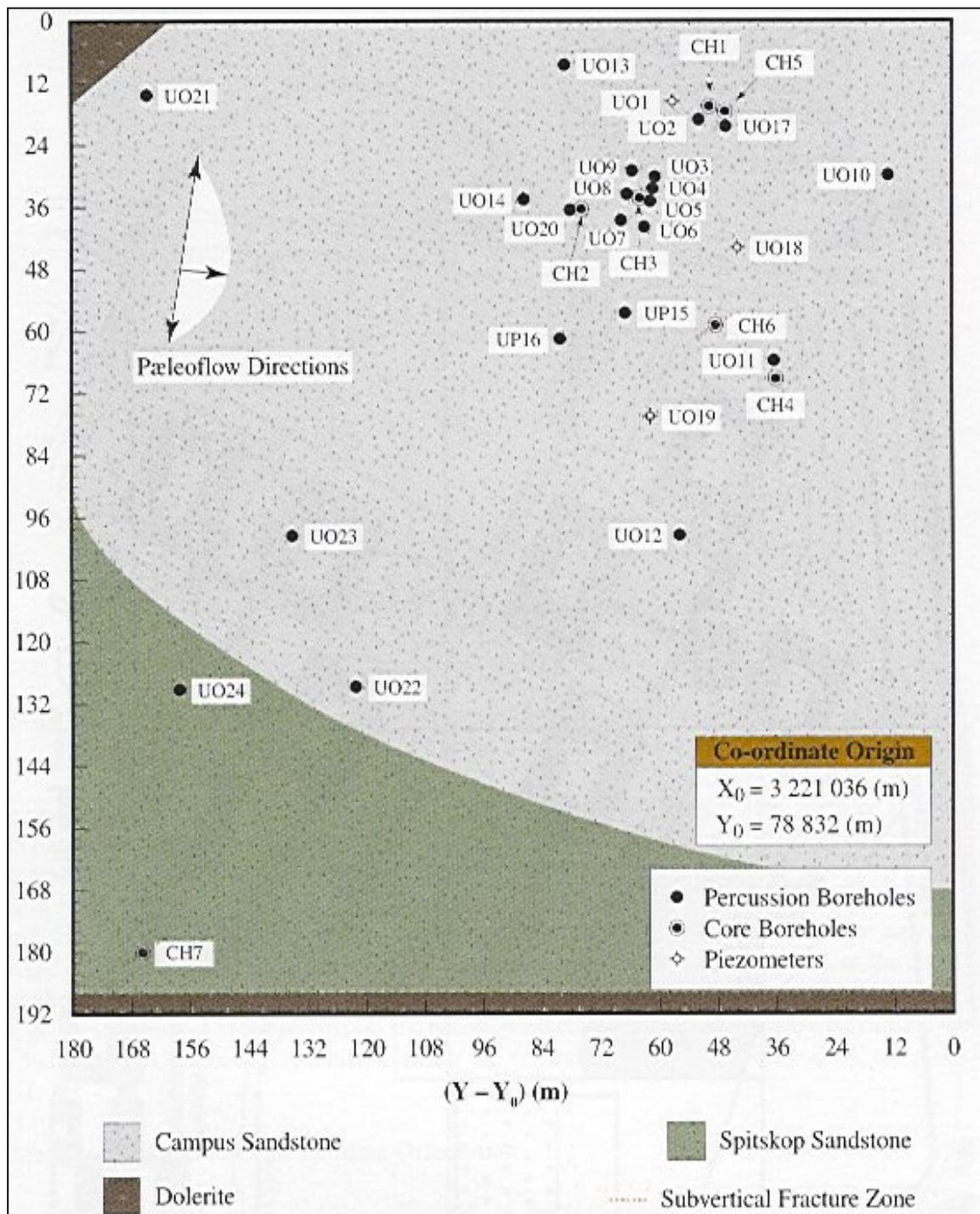
**Fig. 6.1: Borehole positions of the Campus Test Site**
