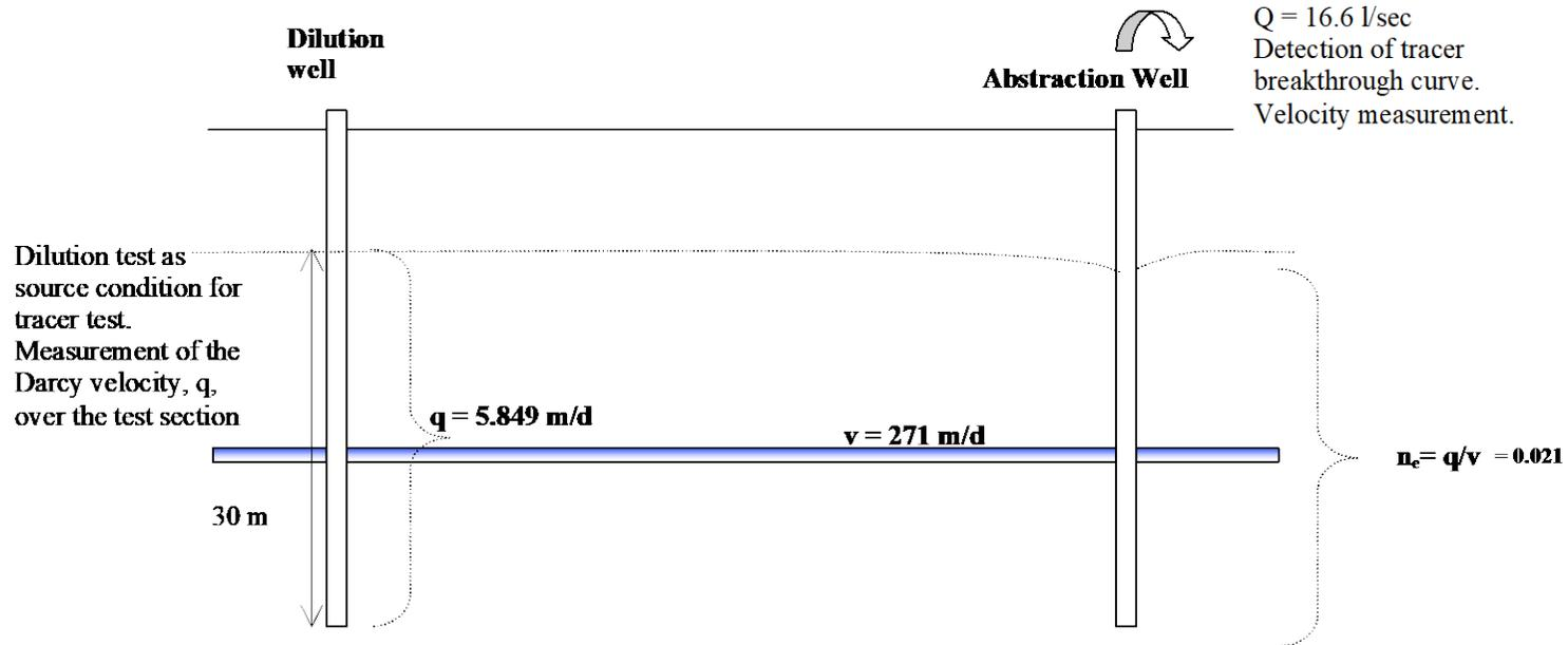
Figure 6.10: Jacobsdal: Velocity measurements in dolerite sill, with interlacing units of Karoo sediments.
