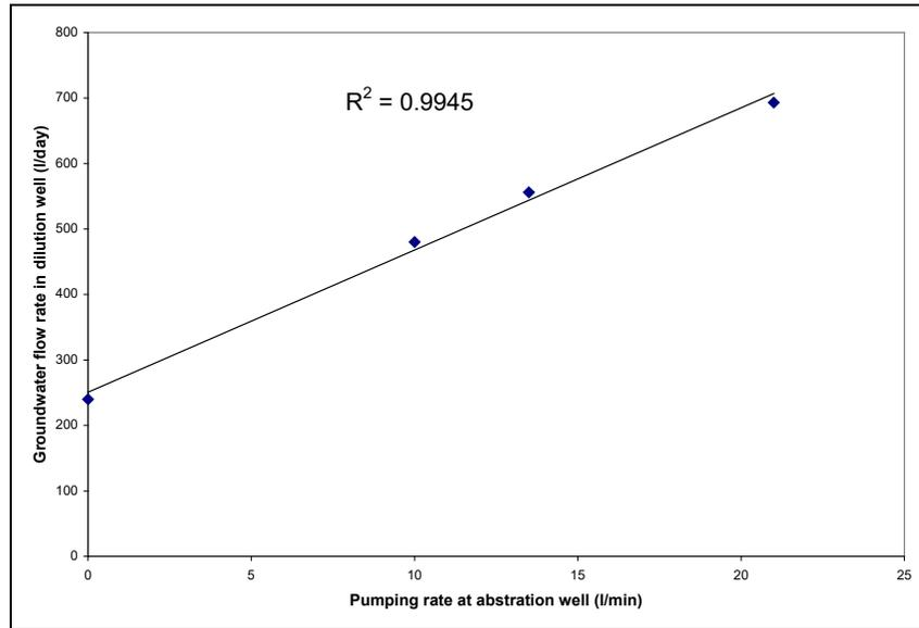
**Fig. 6.4: Groundwater flow rate at UO20 versus the pumping rate in UO5.**
