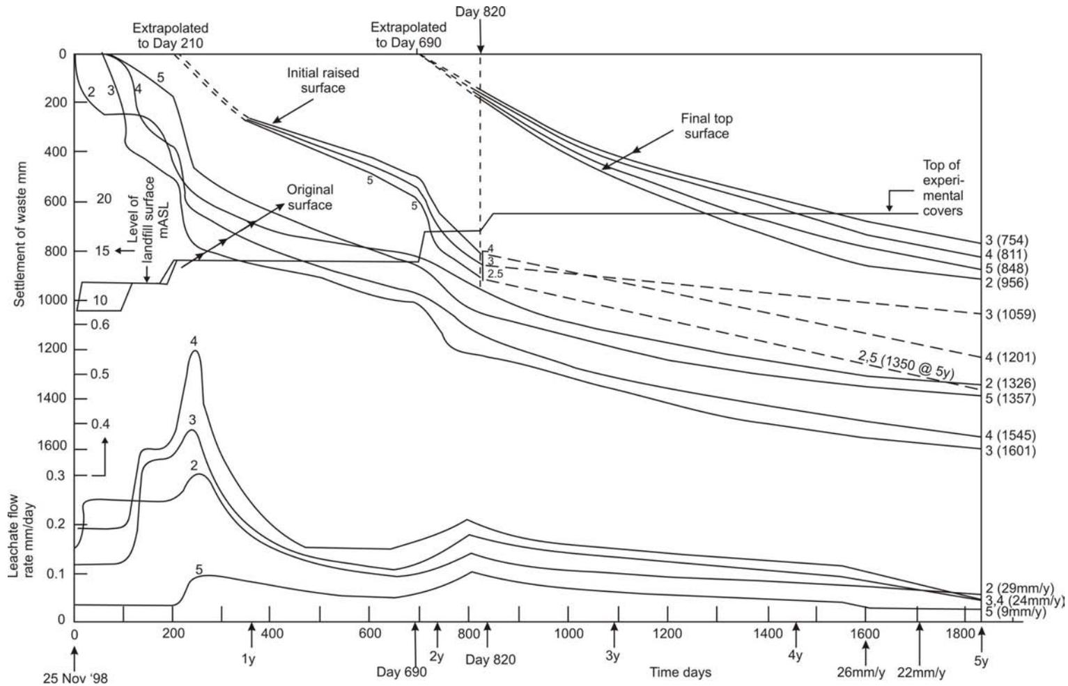
**Figure 6** Records of settlement and leachate flow during the 5 year duration of the raising experiment
