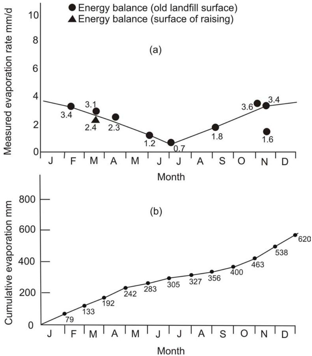
**Figure 10** Evaporation from landfill surface assessed by surface energy measurements
