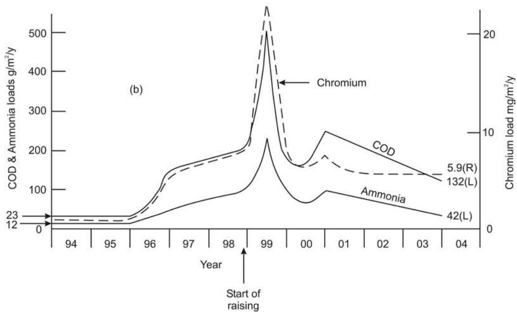
**Figure 9(b)** Variation of chemical loading of leachate for COD, Ammonia and Chromium before and during raising experiment
