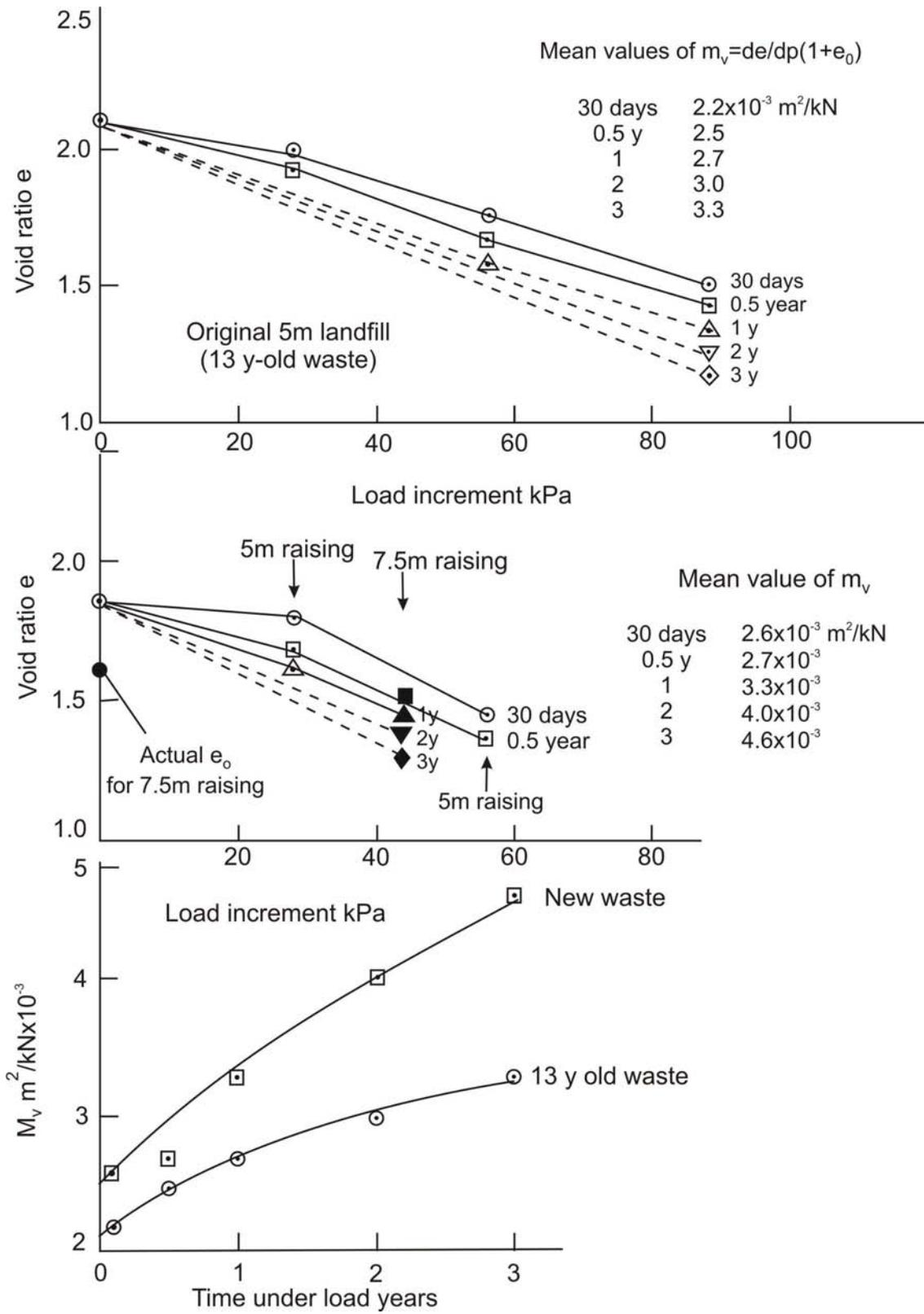
Figure 7 Compression characteristics of waste
