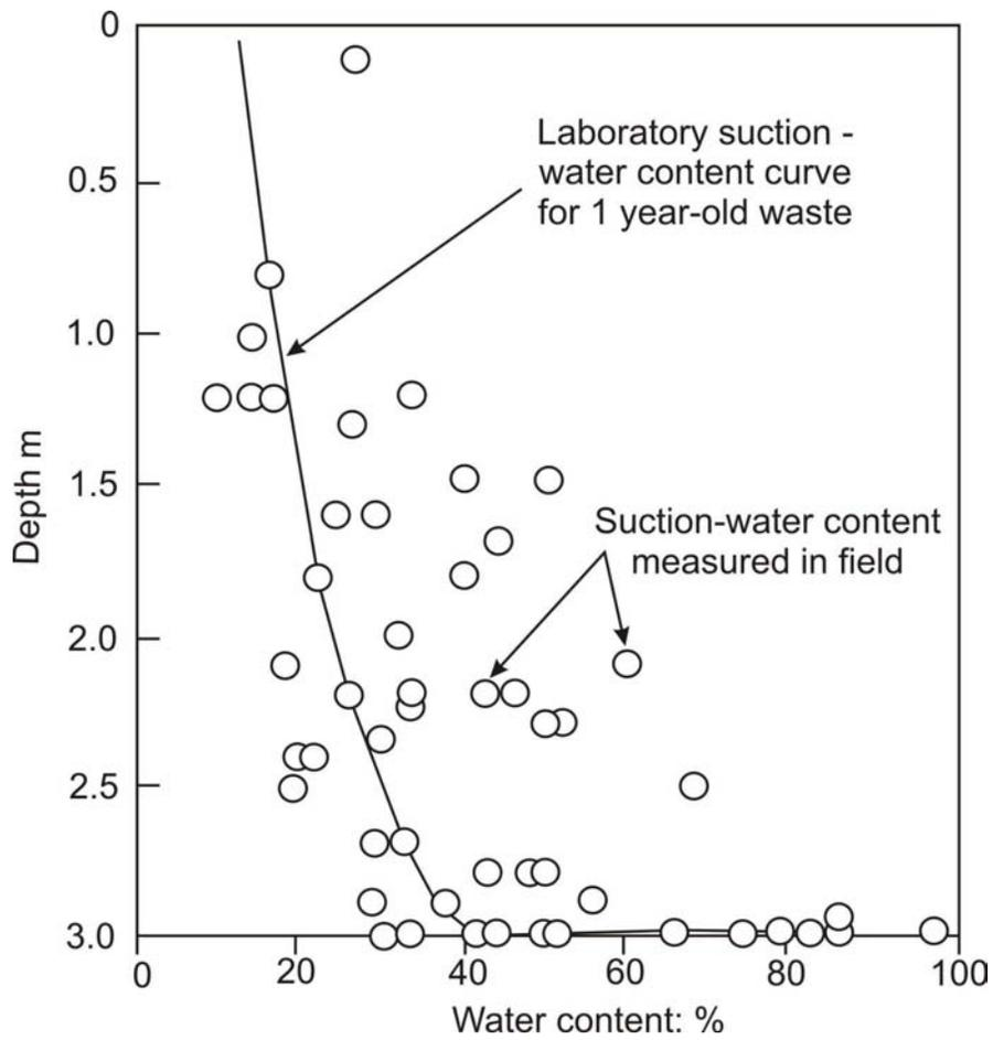
**Figure 3** Comparison of water content-depth measurements in a lysimeter of municipal solid waste with laboratory suction-water content relationship for the waste
