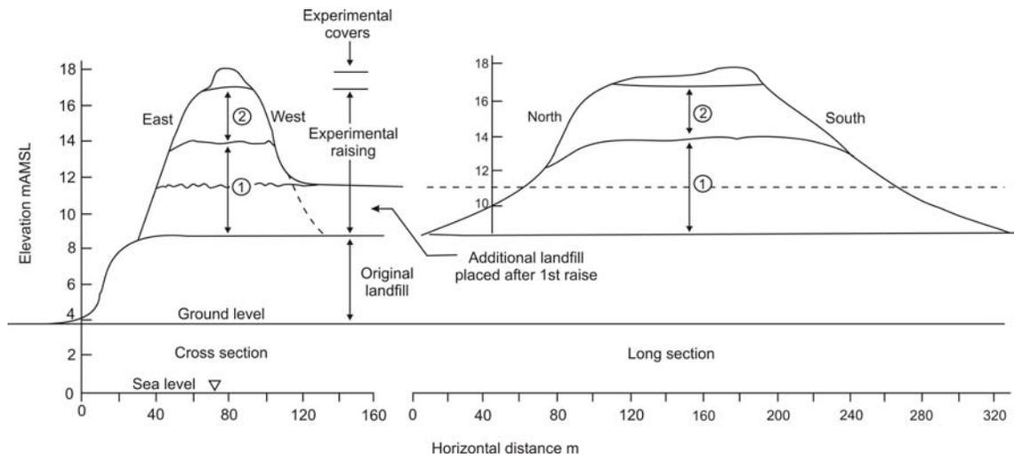
**Figure 5** Transverse and longitudinal profiles of raised portion of landfill (vertical scale exaggerated)
