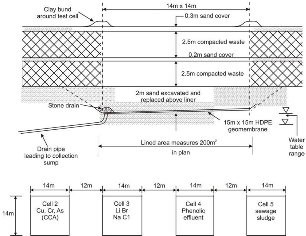
**Figure 4** Arrangement of observation cells (or lysimeters) at Coastal Park landfill
