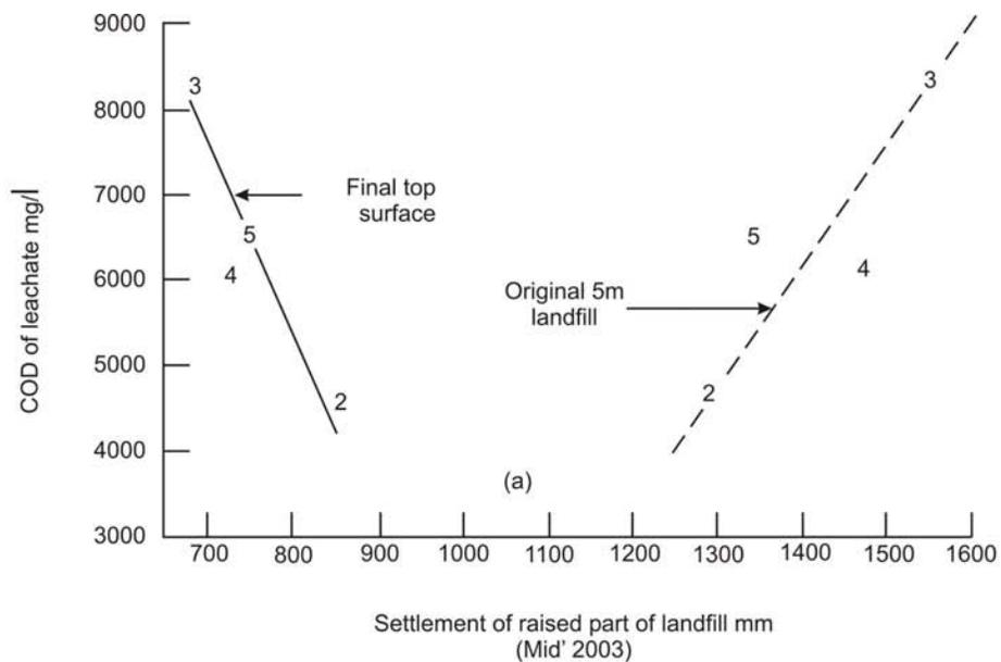
**Figure 9(a)** Correlations between settlement of original landfill surface and final raised surface and Chemical Oxygen Demand of the leachate
