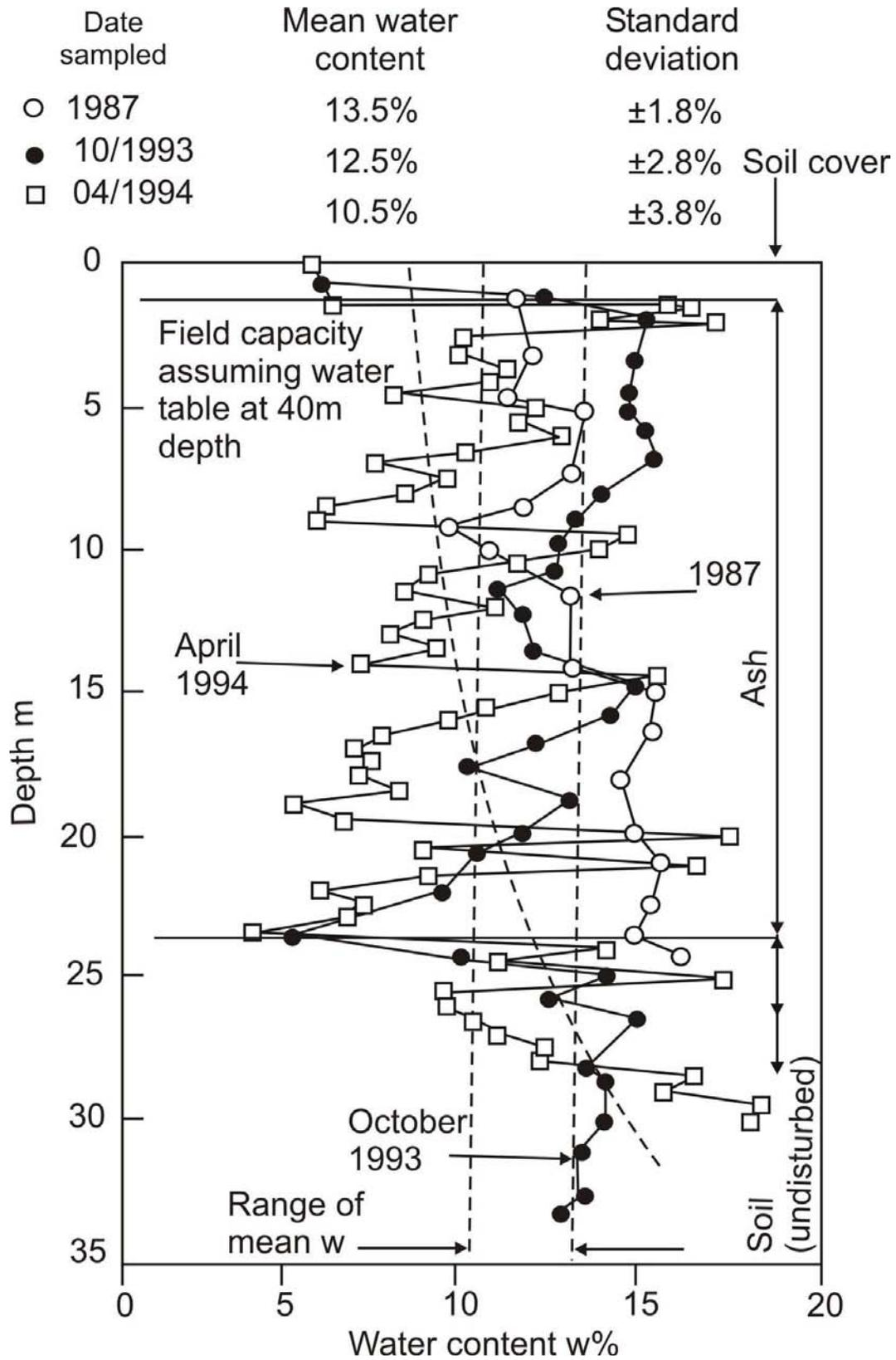
**Figure 2** Comparison of water content-depth measurements in a dump of power station ash with laboratory suction-water content relationship for the ash
