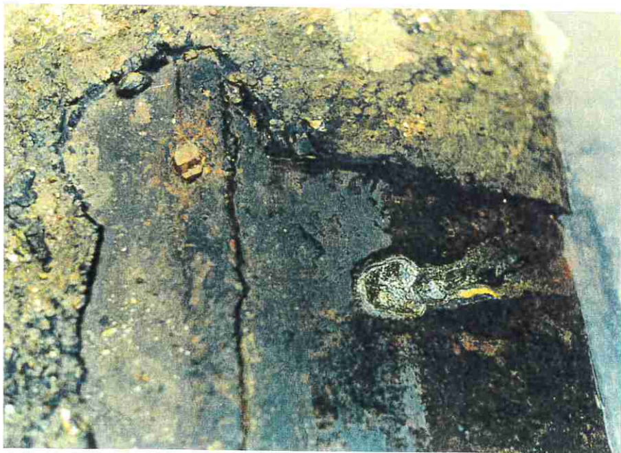
Figure 4: Stray current on pipe samples after cleaning (note - melted parts). Magnification: X0,5.
