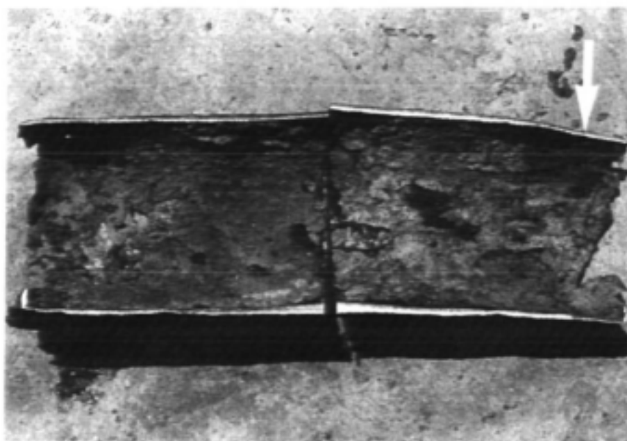
Figure 3: General type corrosion (N.B. thinning wall arrowed). Magnification: X0,4.
