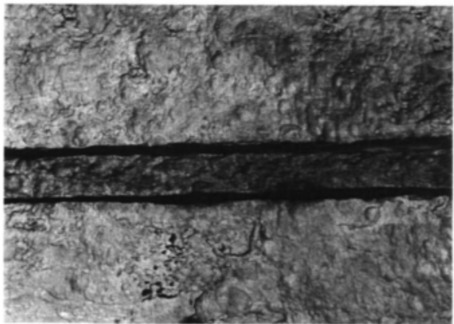
Figure 6(b): Weld attack (HAZ) mild steel pipe (inside). Magnification: X0,6.
