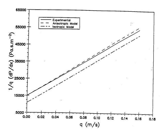
Figure 3: Comparative results for anisotropic foamlike material.
