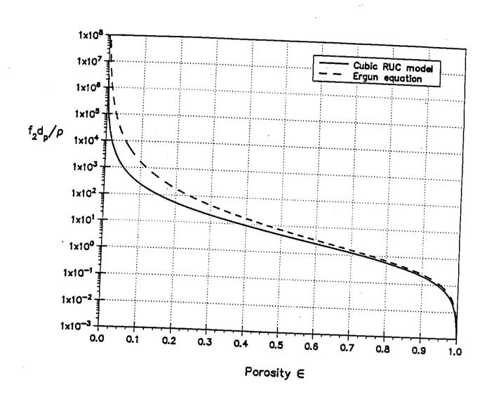
Figure 7: Form drag in granular medium.
