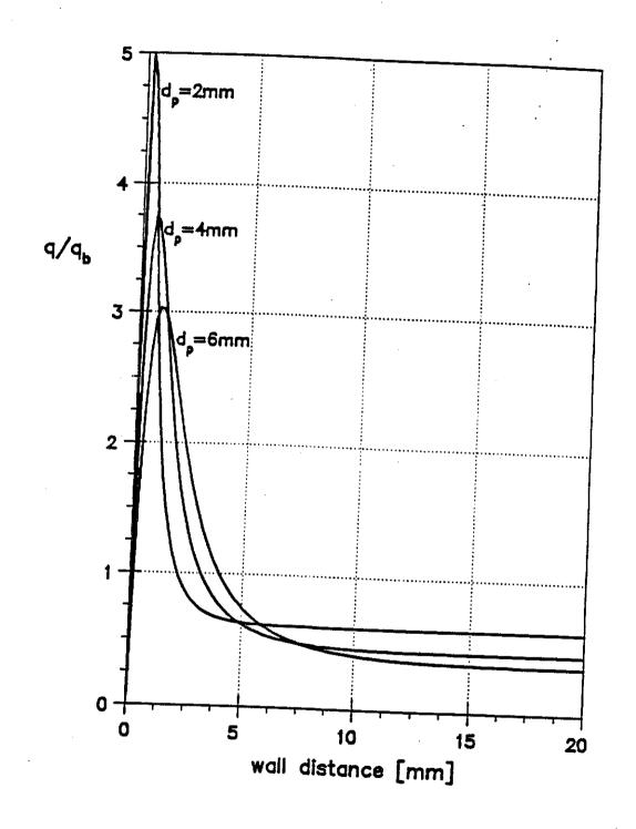
Figure 9: Flow profiles for granular medium in a circular tube
