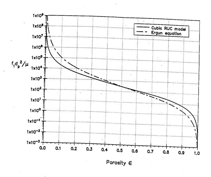
Figure 6: Viscous drag in granular medium.
