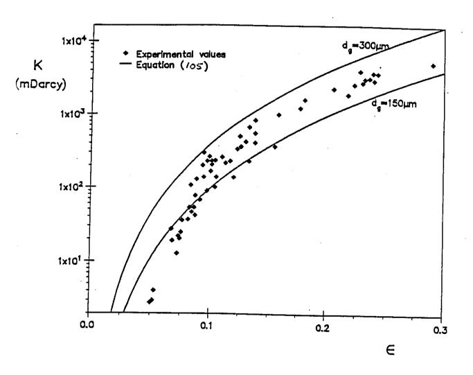
Figure 13: Experimental results for Fontainebleau sandstone.
