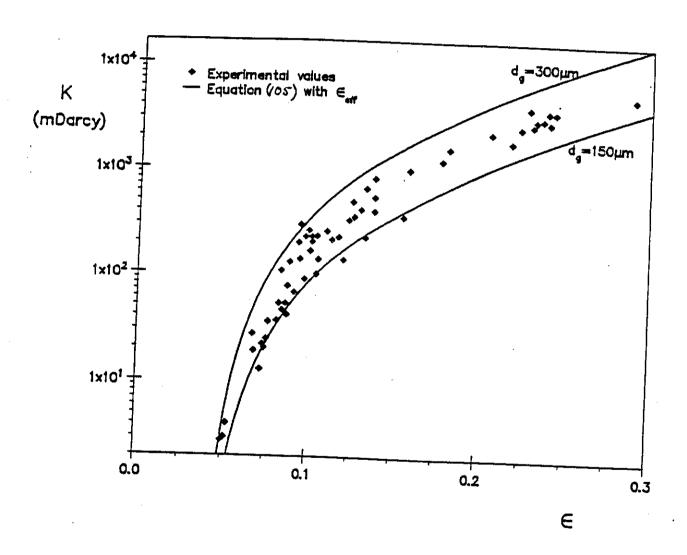
Figure 15: Final results for Fontainebleau sandstone.
