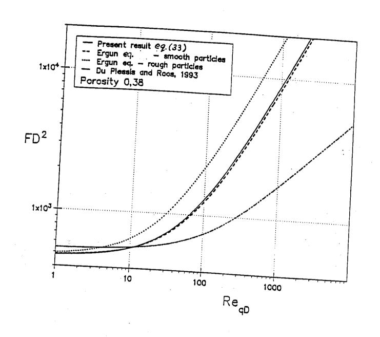
Figure 2: Comparison of results against Ergun equation for granular media.
