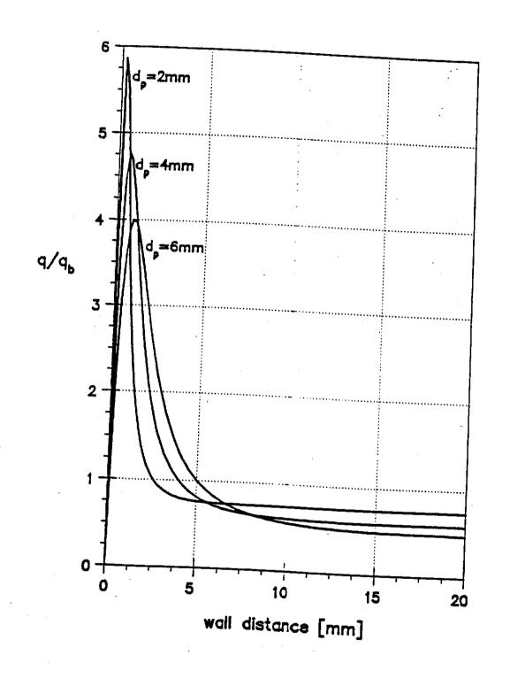
Figure 8: Flow profiles for granuler medium between parallel plates.
