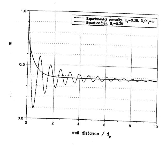
Figure 4: Porosity distribution near external wall.
