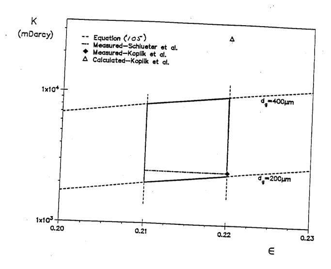
Figure 11: Results for Massilon sandstone.
