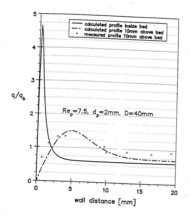
Figure 10: Flow profile inside and 10mm above a tubular packed bed.
