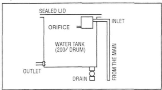
Figure 5.1: 200 & storage tank fitted with a regulating orifice
