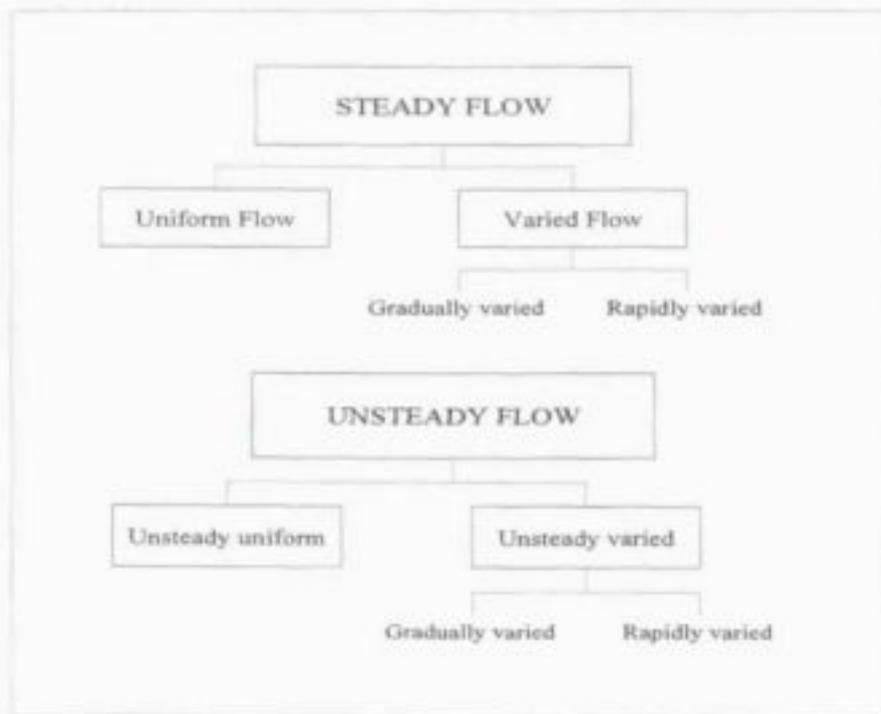
**Figure 5.2** Summary diagram of different flow types
