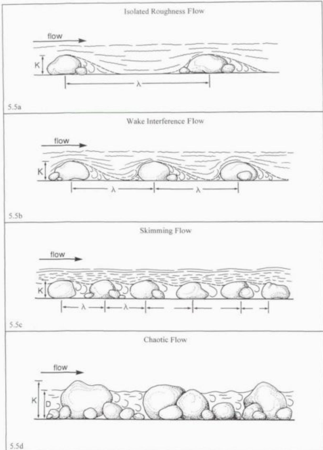
Figure 5.5 Roughness flow classes (after Davis and Barmuta and Gordon *et al.* 1992)
