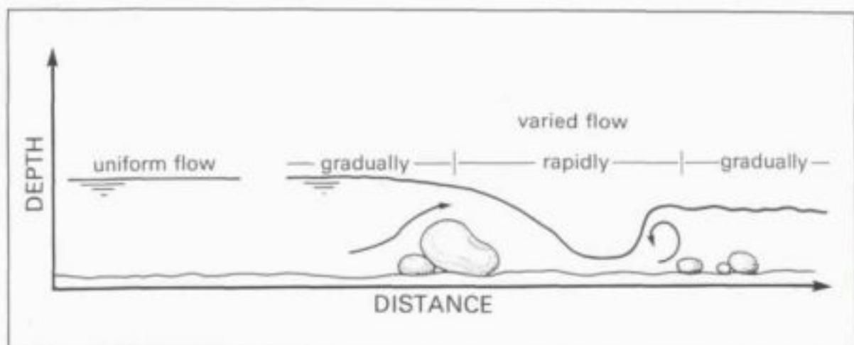
**Figure 5.3** Classification of open channel flow.
