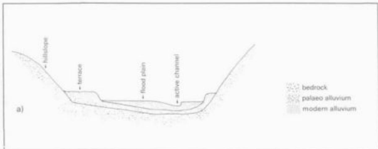
Figure 3.4 Cross sectional form of a humid river system
