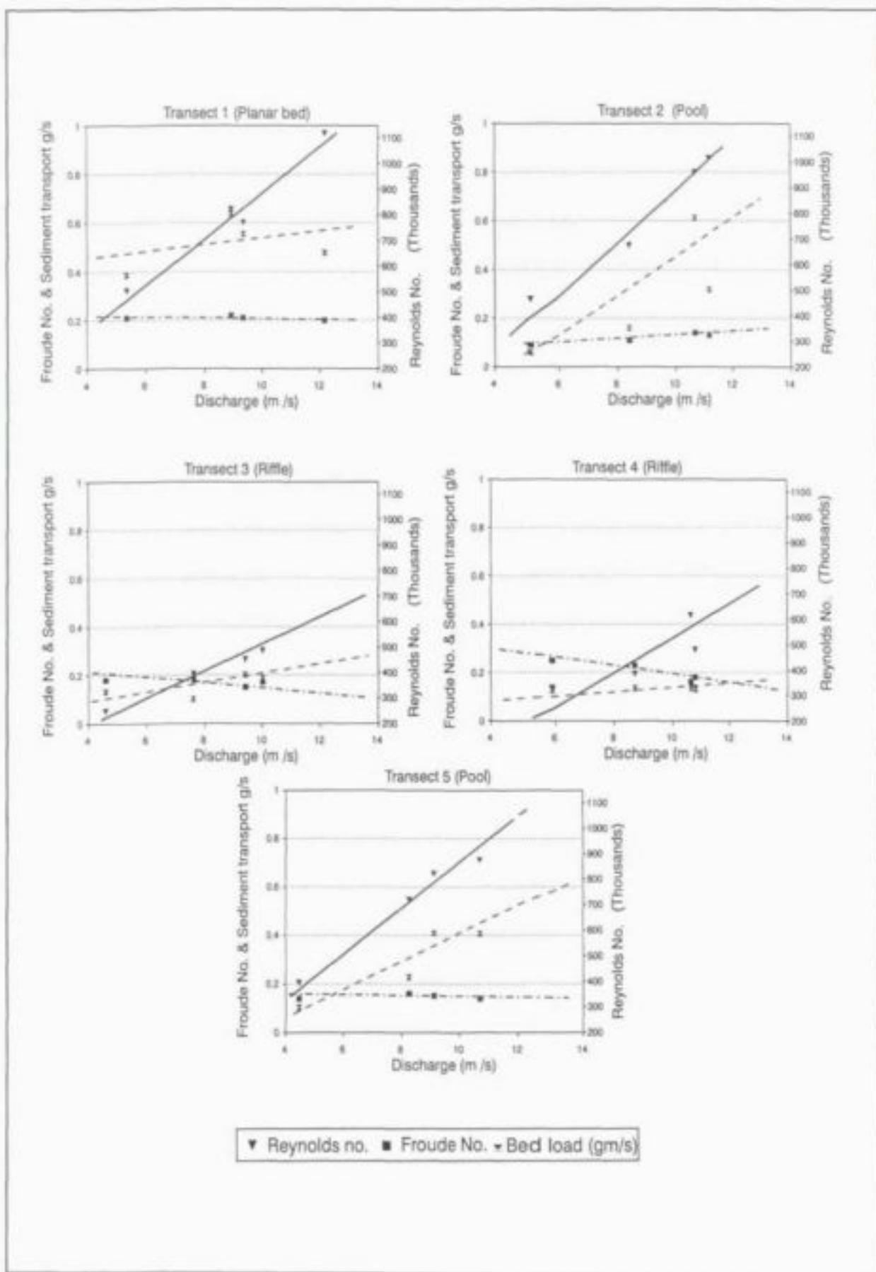
Figure 6.6 Changes in hydraulic indices and bedload transport with discharge
