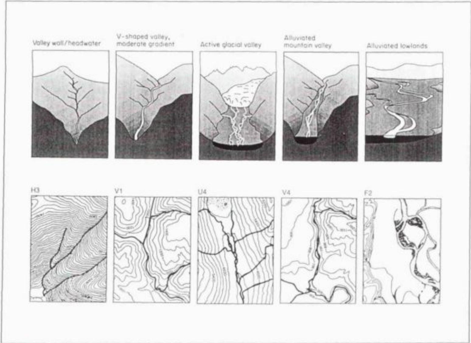
**Figure 2.5** Elements of the Cupp classification as used by the State of Washington, USA. Three-dimensional projections are made from topographic maps to assist in determining segment type.
