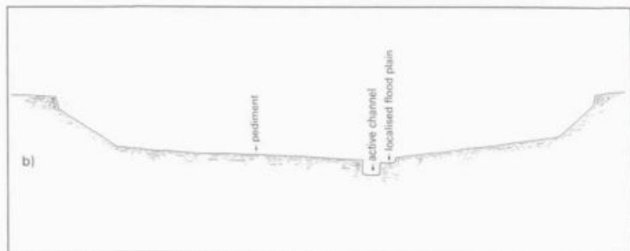
Figure 3.5 Cross sectional form of a semi arid river system
