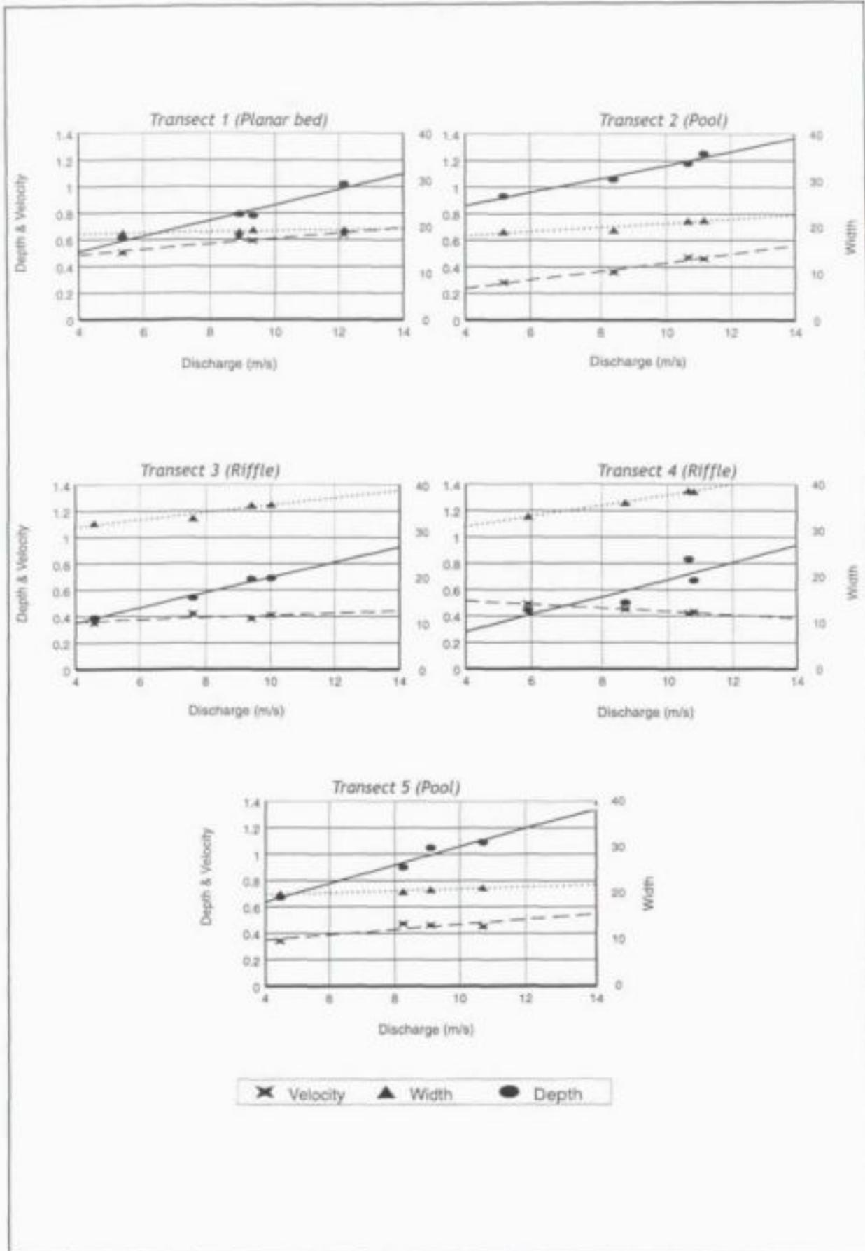
Figure 6.5 Hydraulic geometry, showing changes in width, depth and velocity with discharge
