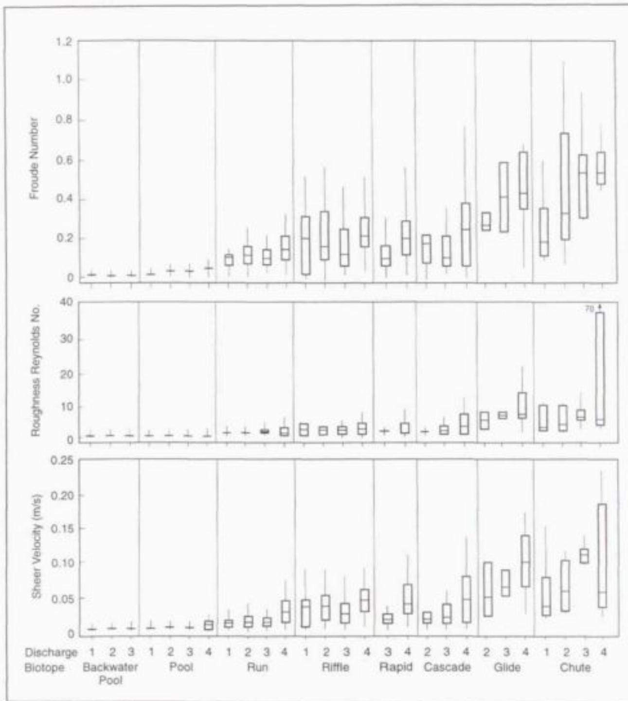
Figure 6.18 Box plots to show hydraulic variability as a response to increasing discharge.
