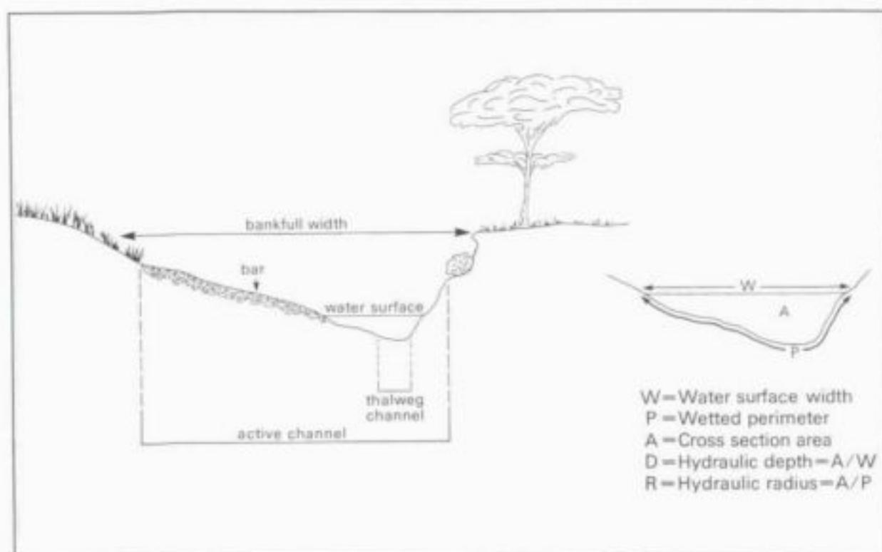
**Figure 3.7** Cross section form variables
