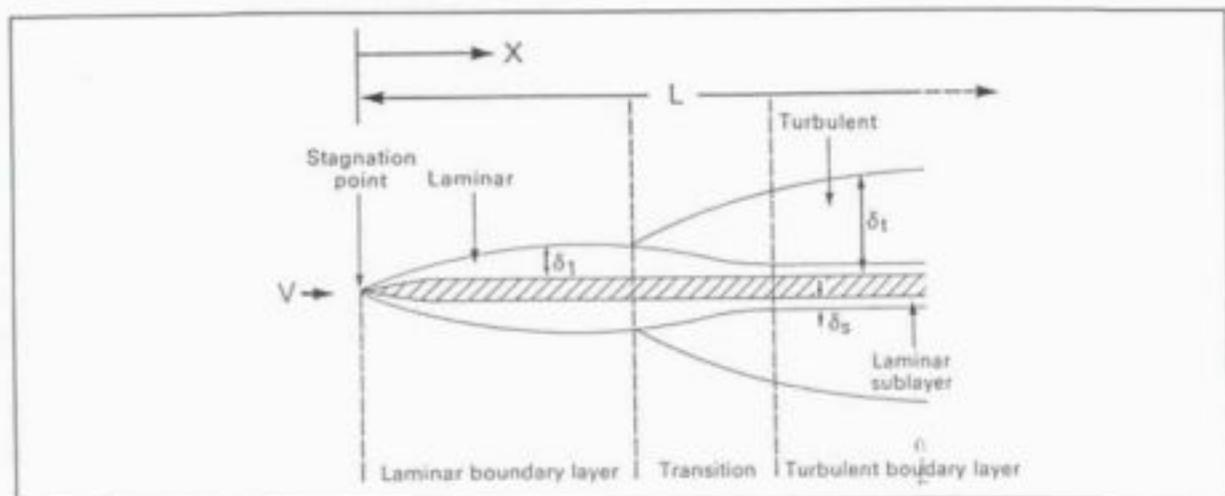
**Figure 5.4** Boundary layer formation around the top of a sharp flat plate ( $L$  is the "characteristic length",  $V$  is the approach velocity,  $x$  the distance from the leading edge and  $\delta$  the boundary layer thickness (for  $l$ , laminar;  $t$ , turbulent and  $s$ , viscous sublayer regions). From Gordon *et al.* (1992).
