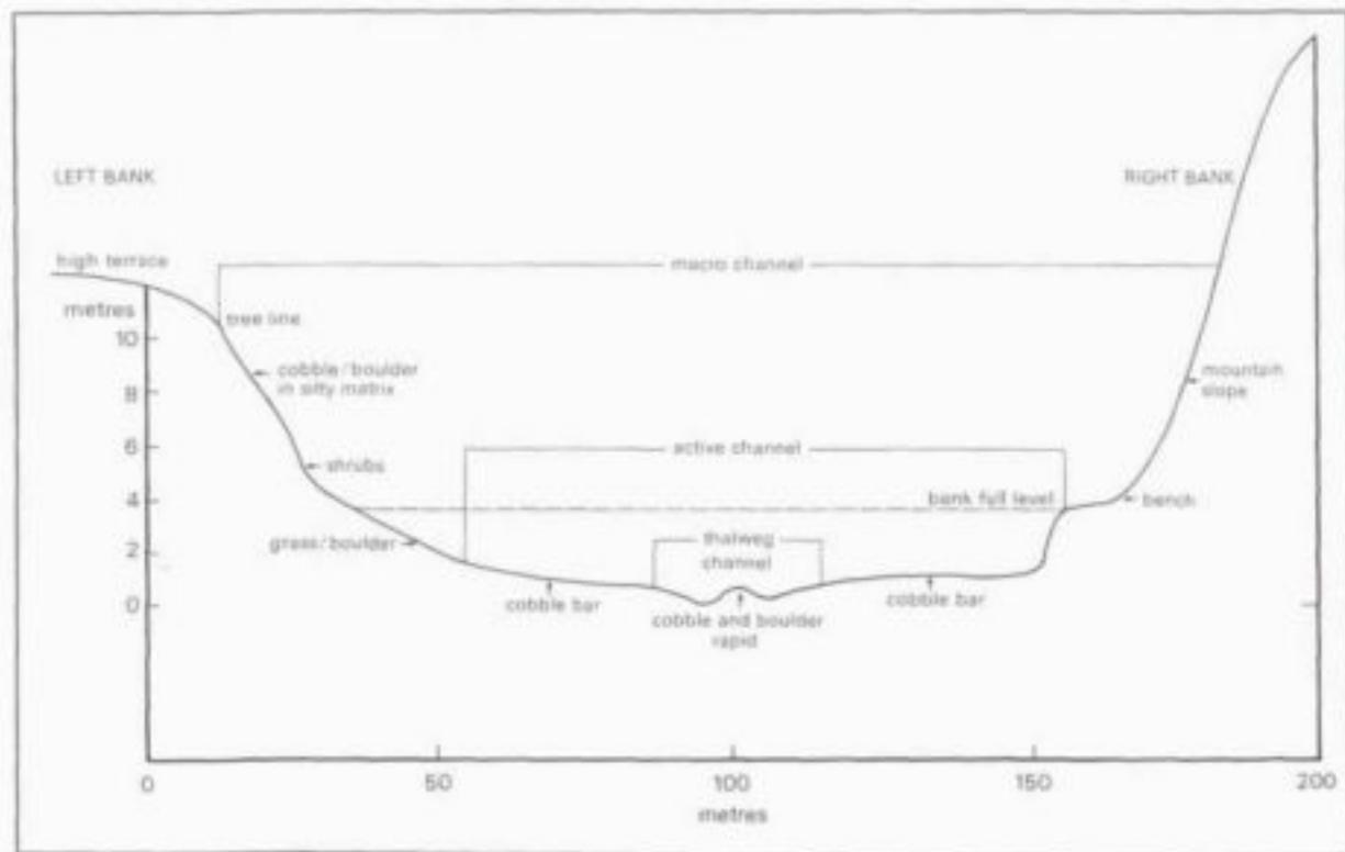
Figure 3.6 Example of a macro-channel in the Tugela River
