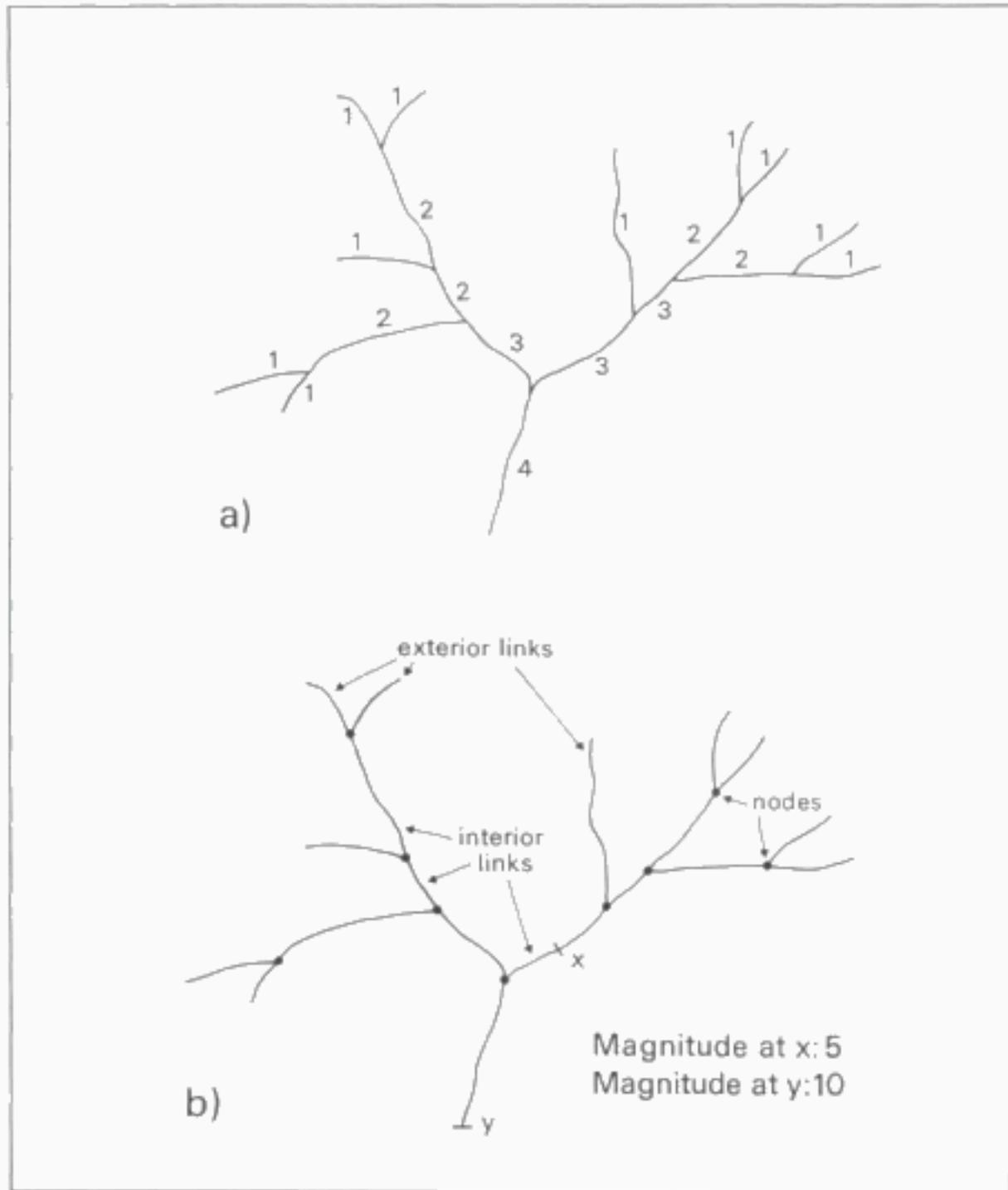
Figure 3.12 Stream Ordering of a) Strahler (1952) and b) Shreve (1966)
