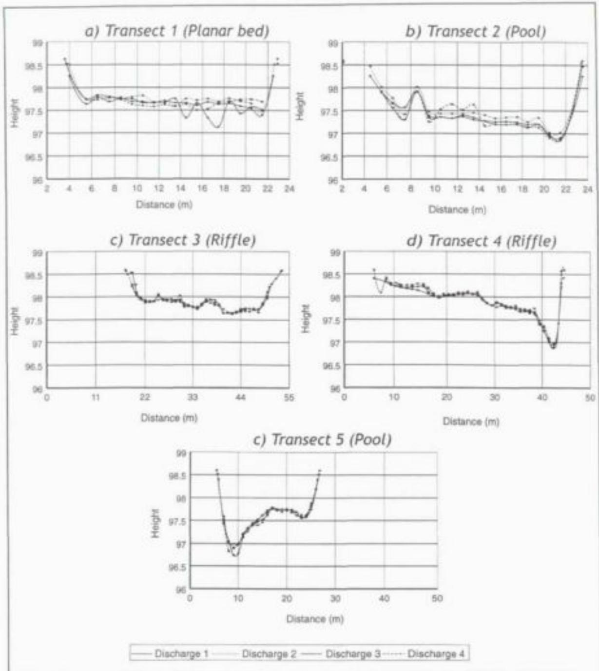
Figure 6.4 Changes in channel cross section with changes in discharge
