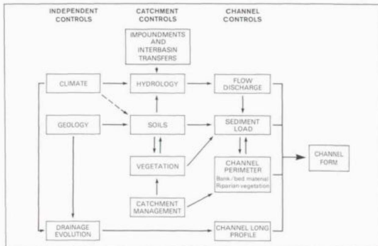
Figure 2.4. Variables in a catchment affecting the dynamics and morphology of a fluvial system, from Rowntree and Dollar (1996a).
