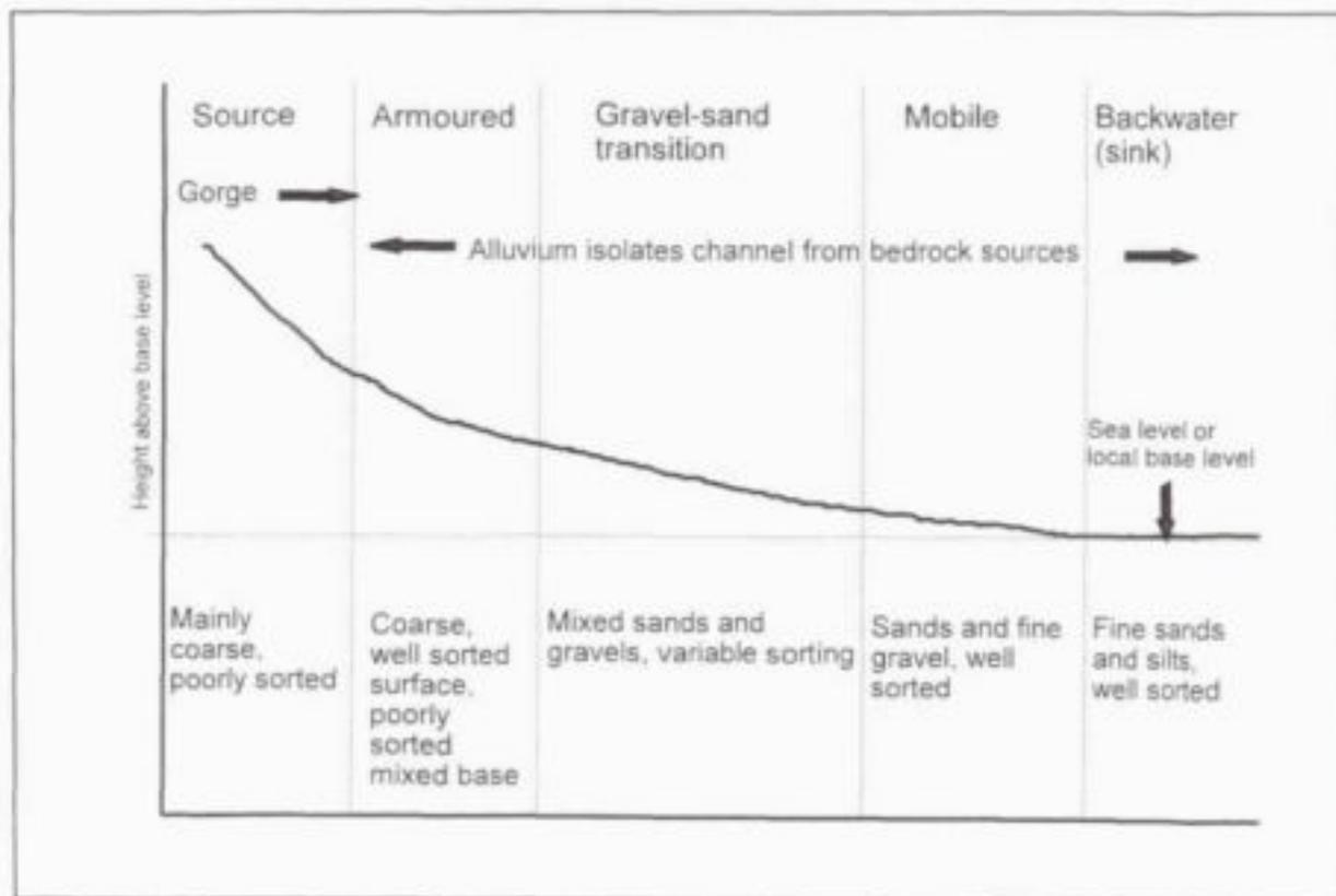
Figure 2.3 River zones characterised by particle size distribution after Pickup (1984)
