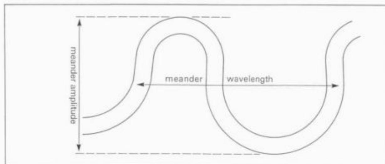
Figure 3.8 Variables describing meander geometry
