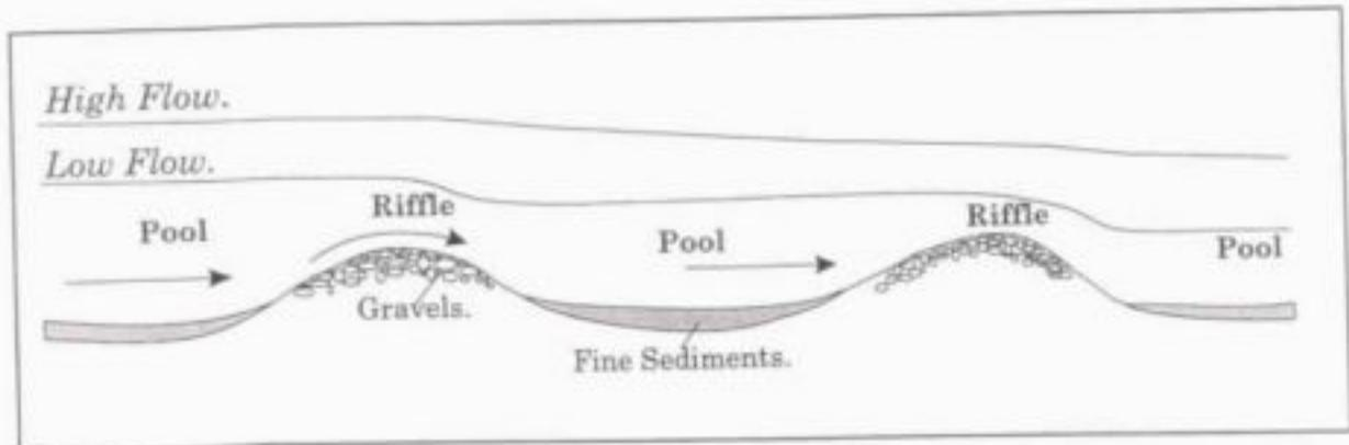
**Figure 4.2** Characteristic profile of pools and riffles, showing changes in depth and water surface slope with increasing discharge
