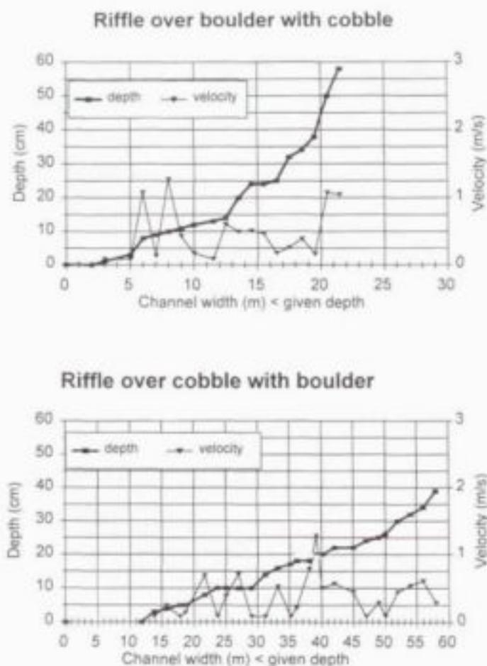
**Figure 8.5** Cumulative depth distribution curves over riffles at sites IFR5 (boulder with cobble) and IFR8 (cobble with boulder). Point velocities are given against the associated depth.
