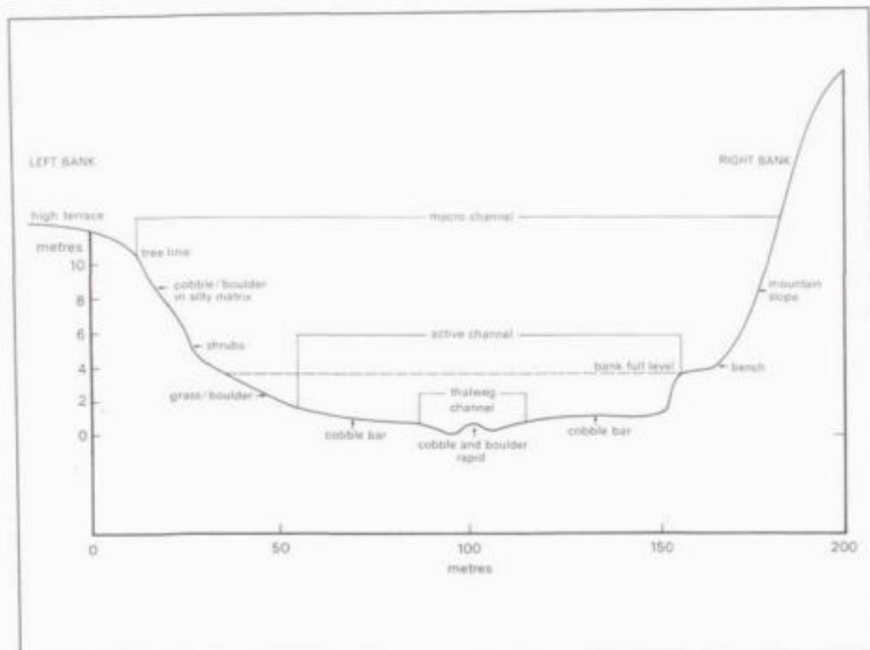
Figure 8.4 Surveyed cross section at IFR 5
