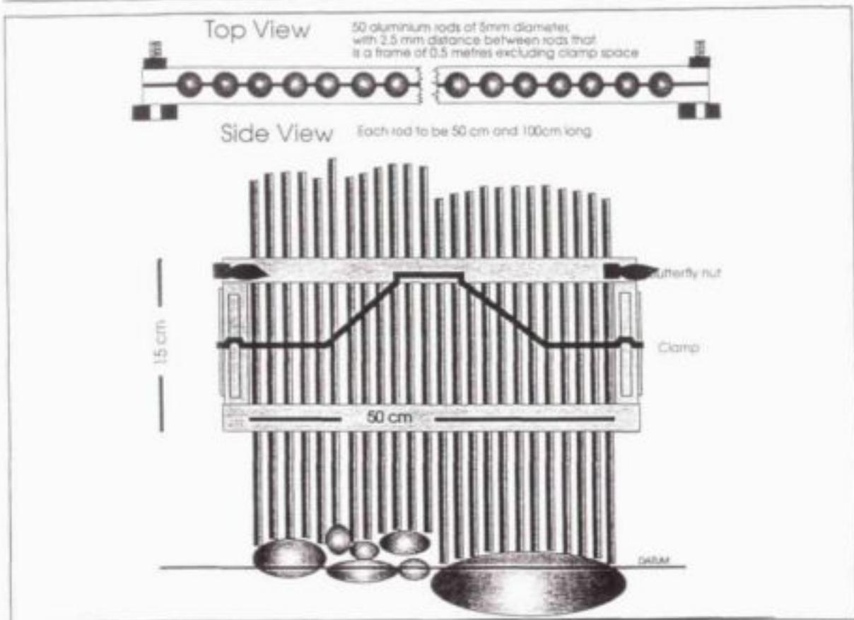
Figure 5.6 Diagram to show specifications of the frame used to measure roughness height.
