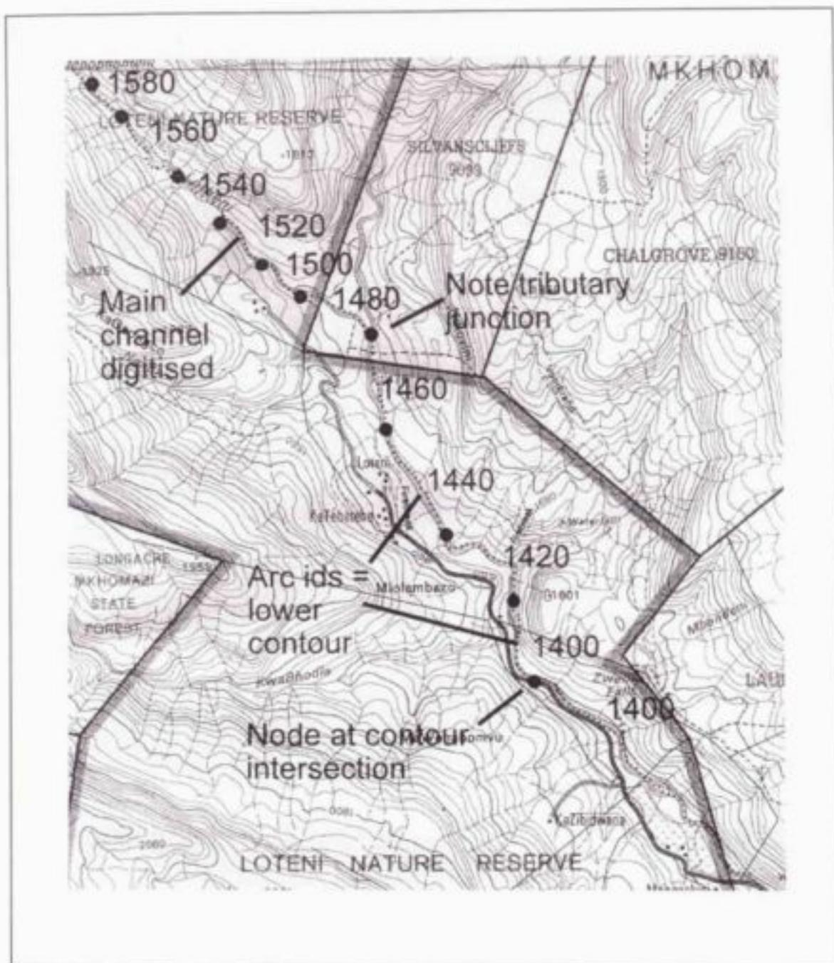
Figure 7.1 Example of a river course and contour intersections
