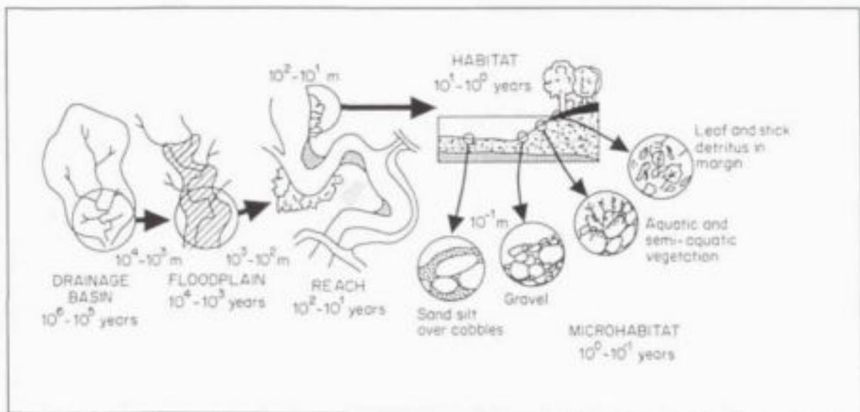
**Figure 2.6** Hierarchical organisation of a stream system with approximate linear spatial scales, from Frissell *et al.* (1986).
