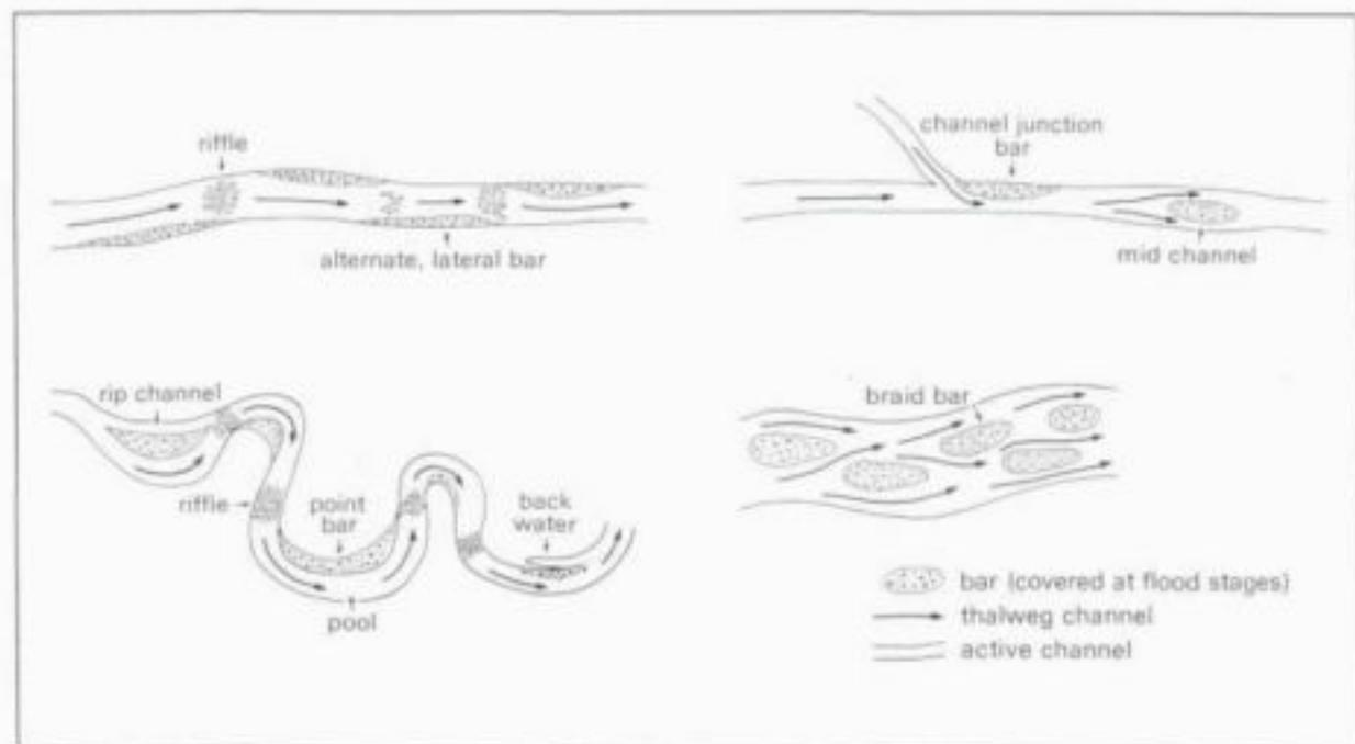
Figure 3.3 Classification of bar types and morphological units
