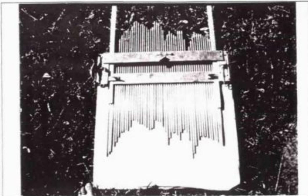
Plate 5.1 Photograph of frame used to measure roughness height.
