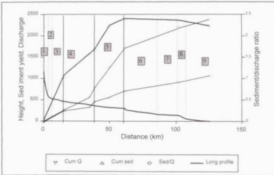
**Figure 7.5** Plot showing discharge and sediment yield data in the Buffalo River for the demarcation of river segments. Height in meters a.m.s.l., sediment yield in  $10^6$  tonnes per annum and discharge in  $10^9$  cubic metres per annum
