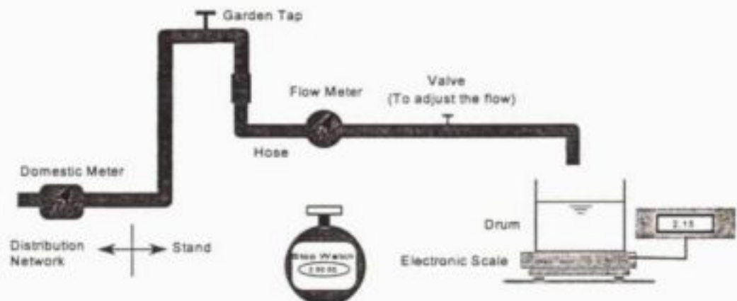
Figure 5 : Schematic of Test-Rig used in Johannesburg and Pinelands
