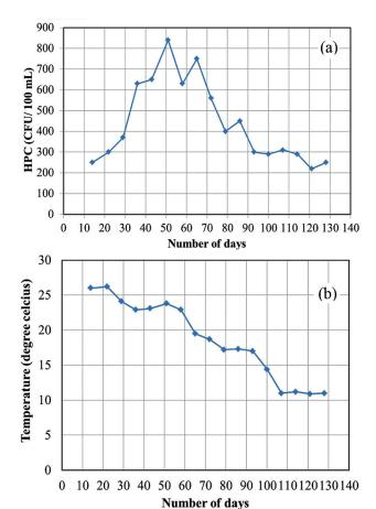
**Figure 3**Trends for (a) biofilm cell count (i.e. HPC) (b) water temperatures at 9:00 in the pipe-loop network for the period February–June 2017
