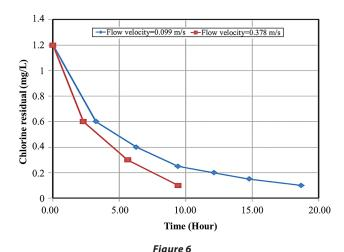
A plot of chlorine residuals against time for pipe-loop experiments demonstrating the effect of flow velocity on chlorine decay in the pipe-loop network
