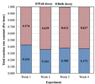
**Figure 5**Relative contribution of the bulk and wall reactions to chlorine decay
