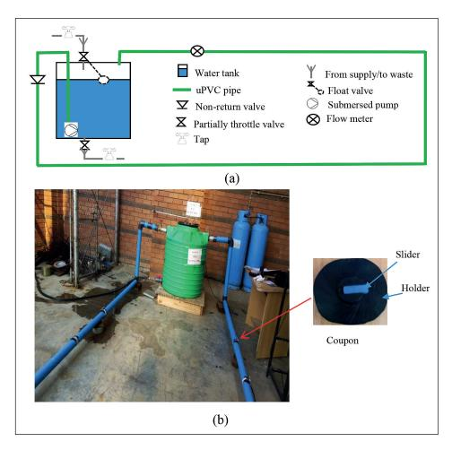
**Figure 1**Pipe-loop network (a) layout (b) experimental set-up
