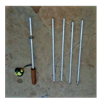
*Figure 1* Cone penetrometer components
