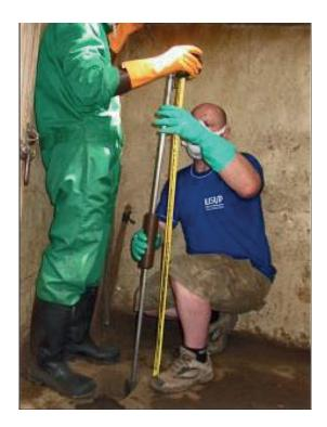
**Figure 2** Cone penetrometer in use
