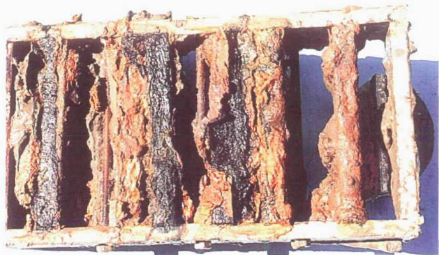
Figure 11(b): Edge coated cast-iron samples exposed under stagnant conditions at Vaal Dam. Note: Corrosion product (black/brown).
