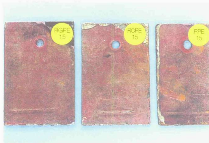
Figure 4(b): Failed coating at the edge (RPE 15). Note: Corroded edges (arrowed).
