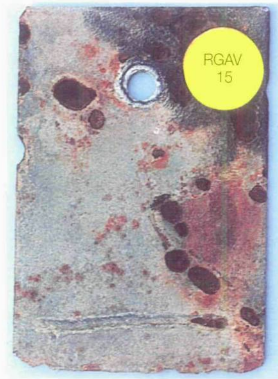
Figure 6(a): Galvanised-vinyl-coated sample from Roodeplaat Dam. Note: Isolated pits and edge effect.
