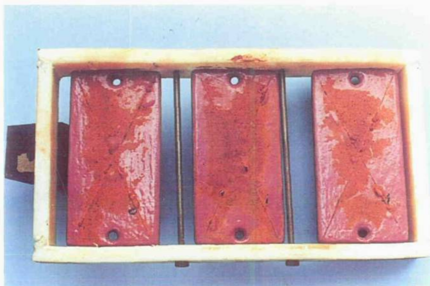
Figure 9(a): Coated samples from the stagnant conditions covered with corrosion product at Western Transvaal Regional Water Company.
