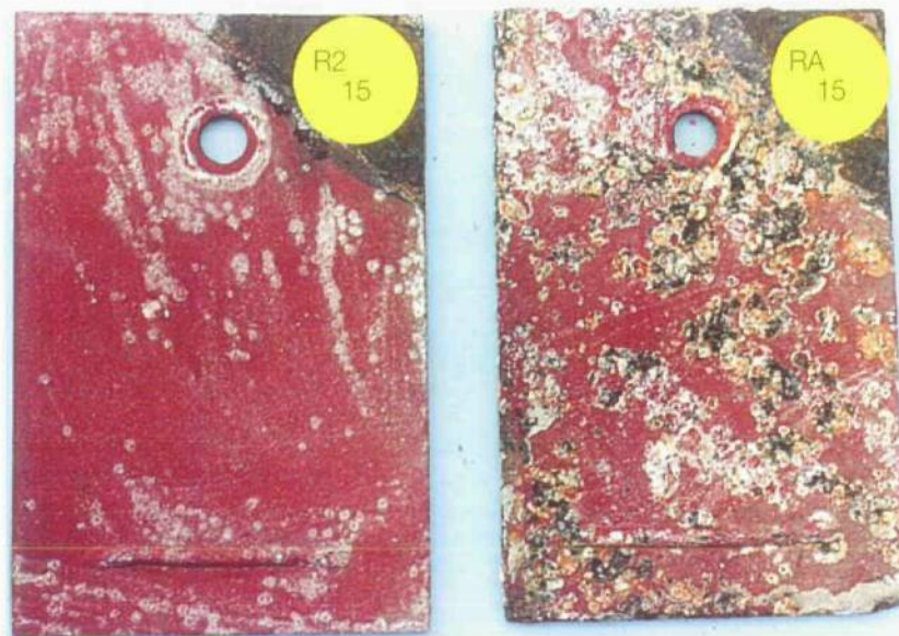
Figure 5(a): Non-metallic coated samples from Roodeplaat. Note: Isolated tubercles throughout the surface (RA 15), and corrosion product (black/brown).
