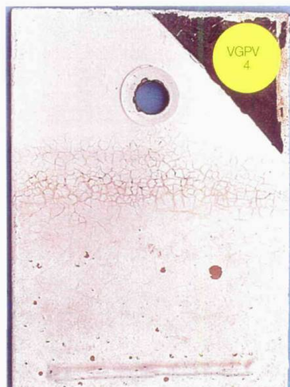
Figure 5(b): Non-metallic coated sample from Vaal Dam. Note: Cracked coating defect.
