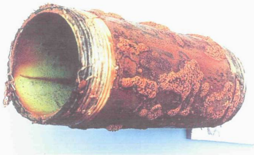
Figure 8(a): Internally lined pipe sample from stagnant condition (Cottesloe) Note: Cracking along weld.
