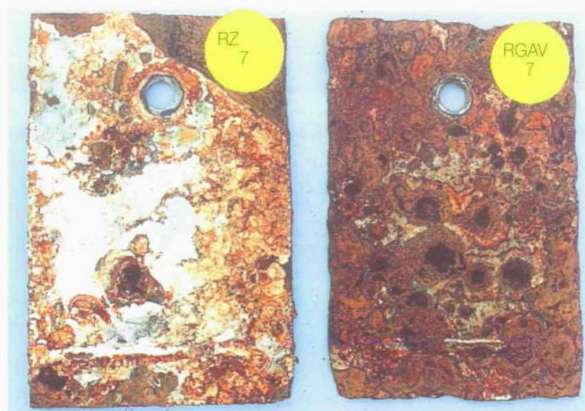
Figure 6(b): Zinc coated (RZ 7) and Galvanized-vinyl-coated samples from Roodeplaat Dam. Note: (RZ7) zinc coating removed and (RGAV7) with isolated pits.
