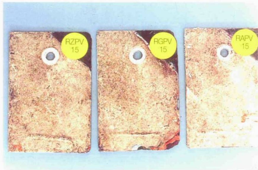
Figure 4(a): Coating defect at the bottom edge (arrowed) (RGPV 15).
