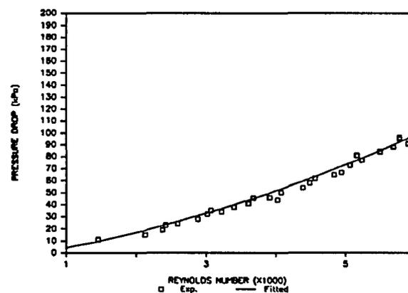
**FIGURE 3.3 : EXPERIMENTAL AND FITTED PRESSURE DROP DATA AT VARIOUS *Re*-NUMBERS - MODULE N100L615**
