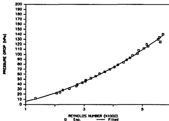
**FIGURE 3.4 : EXPERIMENTAL AND FITTED PRESSURE DROP DATA AT VARIOUS *Re*-NUMBERS - MODULE N150L300**
