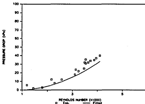
**FIGURE 3.5 : EXPERIMENTAL AND FITTED PRESSURE DROP DATA AT VARIOUS *Re*-NUMBERS - MODULE N150L405**
