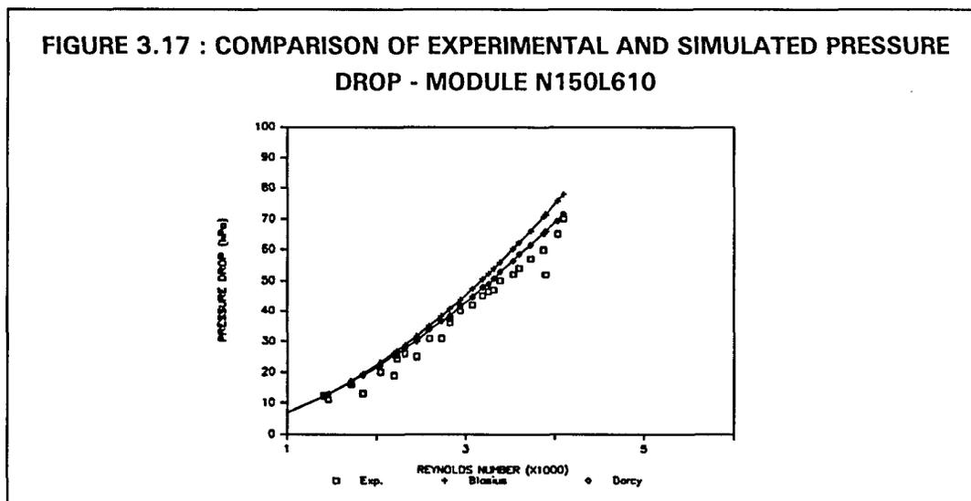
Figures 3.12 to 3.17 demonstrate that a good correlation is obtained between the actual experimentally determined pressure drop values and those predicted by the Darcy relationship given in equation (2). The Stanton friction factor  $f_s$ , which is used in conjunction with the Darcy relationship, may be calculated from the empirical law of Blasius or by reading off the experimental  $f_s$ - $Re$  curve in Figure 3.9.
