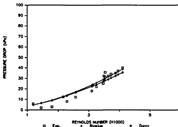
**FIGURE 3.16 : COMPARISON OF EXPERIMENTAL AND SIMULATED PRESSURE DROP - MODULE N150L405**
