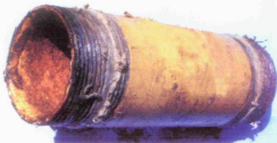
Figure 8(a): Internal appearance of pipe specimen with non-metallic coating No.9 before cleaning (X0,54).
