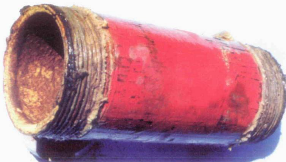
Figure 4(a): Internal appearance of pipe specimen with non-metallic coating No.4 before cleaning (X0,54).
