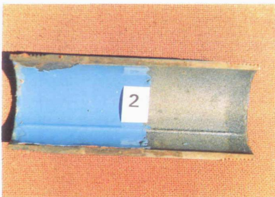
Figure 2(b): Surface appearance of non-metallic coating No.2 and carbon steel substrate after 42 months testing (X0,64).
