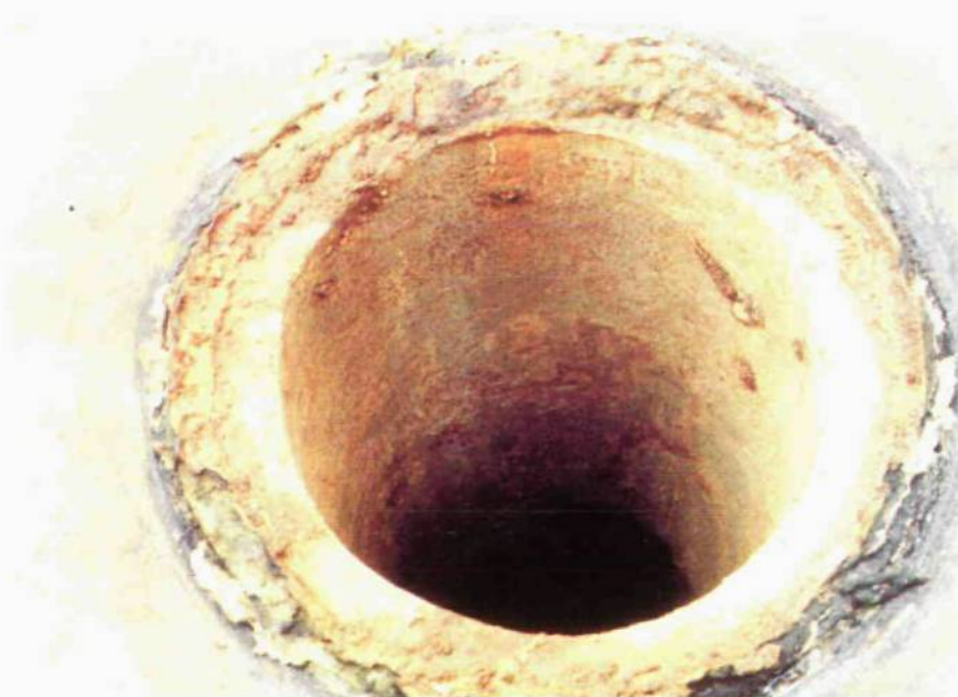
Figure 11(b): Mortar-lined carbon steel pipe showing the condition of the mortar lining (X0,42). No degradation of the cement mortar was noted.
