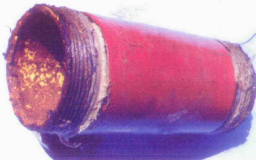
Figure 7(a): Internal appearance of pipe specimen with non-metallic coating No.8 before cleaning (X0,54).
