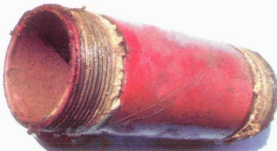
Figure 1(a): Internal appearance of pipe specimen with non-metallic coating No. 1 before cleaning (X0,54).
