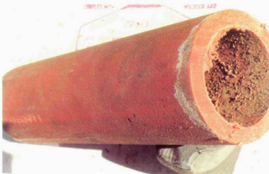
Figure 9(a): Non-metallic piping specimen after (polykop) 42 months testing. (Note: Brown product from metallic pipes).
