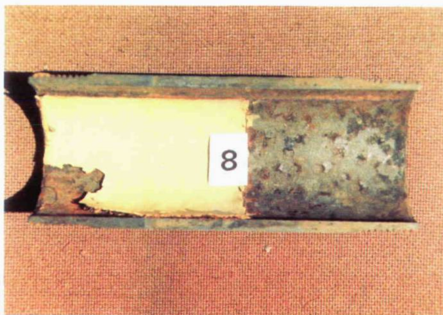
Figure 7(b): Surface appearance of non-metallic coating No.8 and carbon steel substrate after 42 months testing (X0,64).
