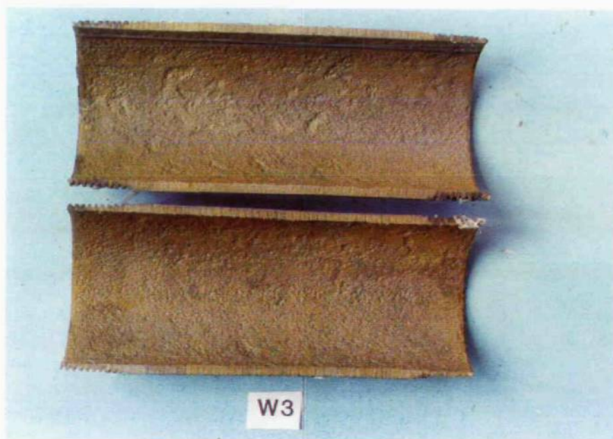
Figure 13(b): Internal surface of carbon steel pipe specimen after cleaning (X0,62). (Note: Average pit depth (0,4mm)).
