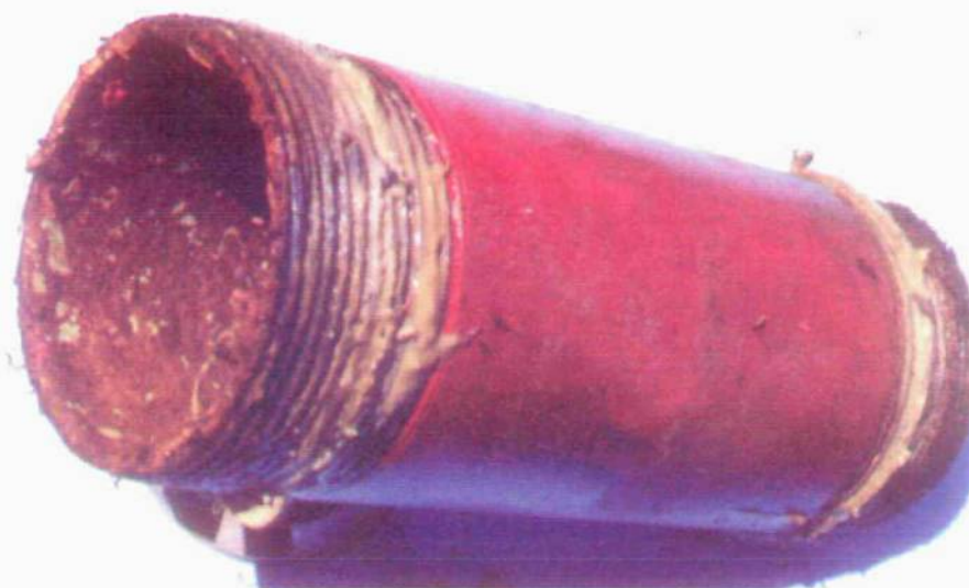
Figure 5(a): Internal appearance of pipe specimen with non-metallic coating No.5 before cleaning.
