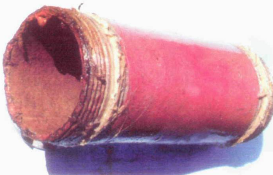
Figure 2(a): Internal appearance of pipe specimen with non-metallic coating No. 2 before cleaning (X0,54).
