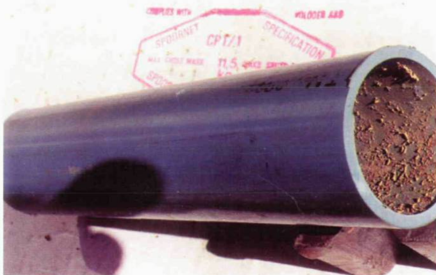
Figure 9(b): Non-metallic piping specimen (HDPE) after 42 months testing. (Note: Brown product from metallic pipes).
