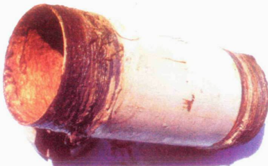
Figure 3(a): Internal appearance of pipe specimen with non-metallic coating No.3 before cleaning (X0,54).
