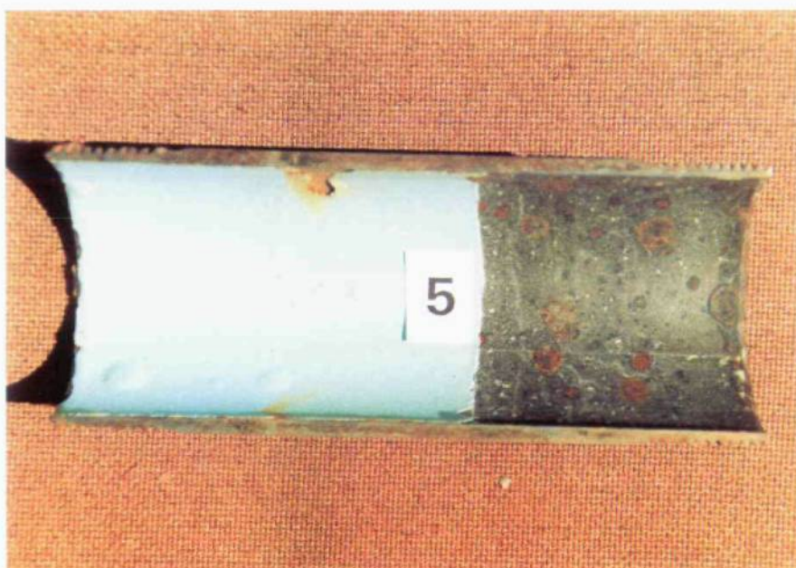
Figure 5(b): Surface appearance of non-metallic coating No.5 and carbon steel substrate after 42 months testing (X0,64).
