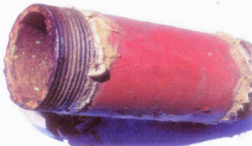
Figure 6(a): Internal appearance of pipe specimen with non-metallic coating No.6 before cleaning. (X0,54)
