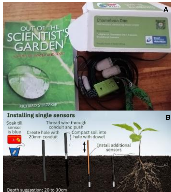
Figure 7.5. Chameleon card and sensors that were supplied to the communities (A) and the installation instruction manual (B).
