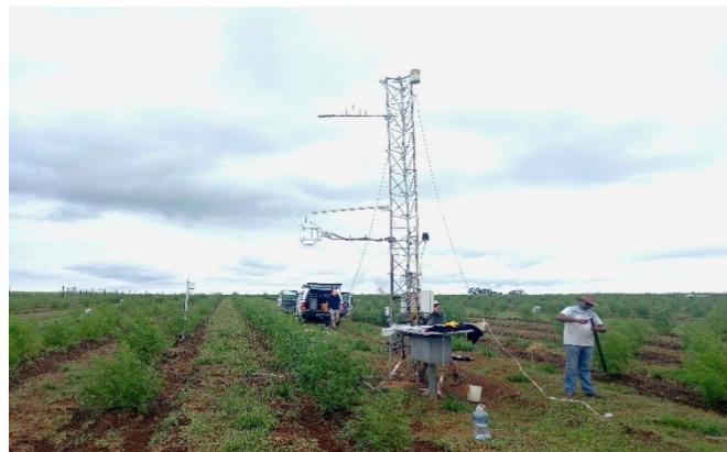
Figure 4.3 Installation of the Eddy Covariance flux tower at Site A
