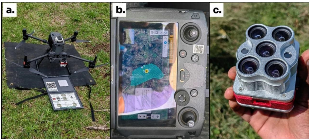
Figure 3.3 UAV image acquisition equipment: (a) the DJI Matrice 300 drone alongside a calibration reflectance panel, (b) the DJI smart controller displaying the flight plan, and (c) the MicaSense Altum camera
