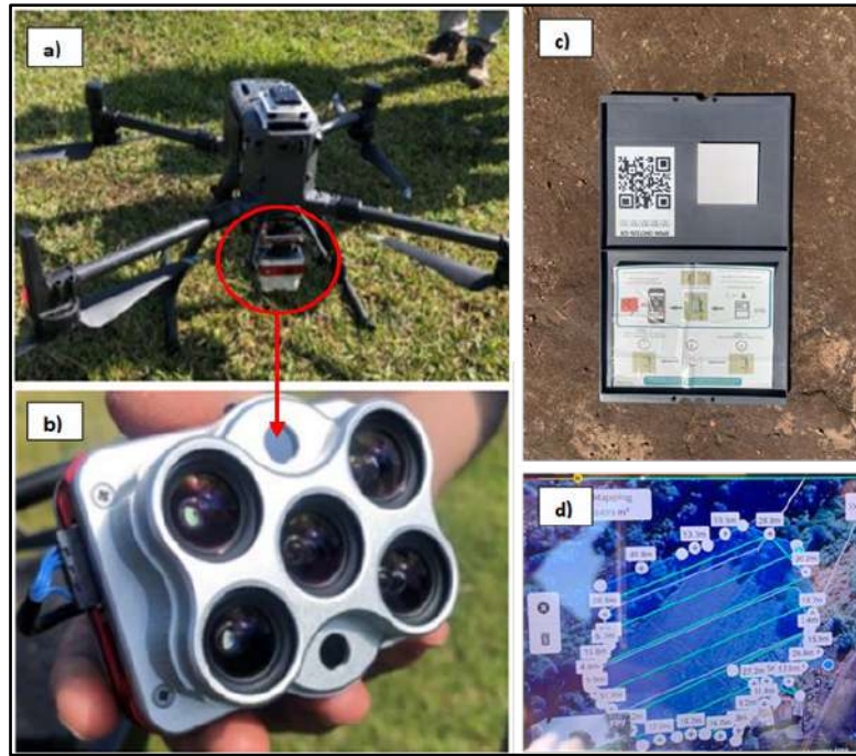
Figure 8-1 a) Matrice 300 UAV integrated with the Altum sensor serving as the imaging platform used in this study, b) the Altum camera, c) the calibrated reflectance panel and d) the flight path plan for the study image
