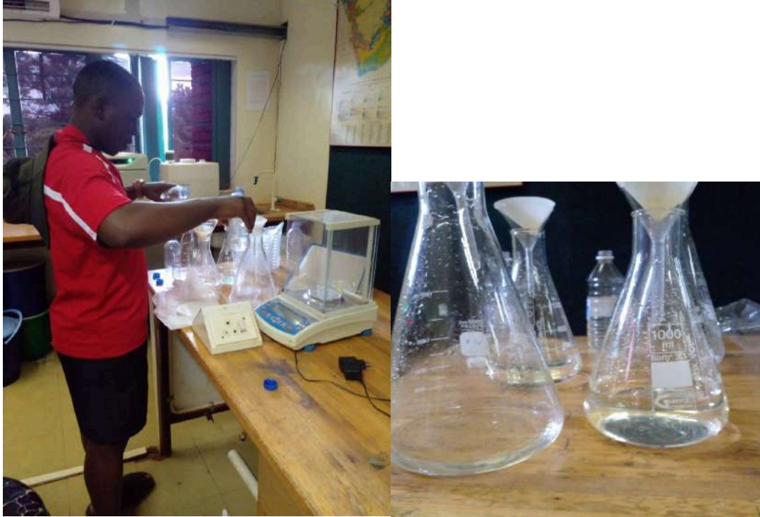
Figure 5.3 Sediment separation and sediment sample preparation.
