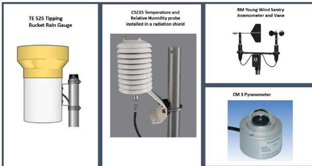
Figure 11. Standard sensors used as references to evaluate CWS stations at the UKZN site in Pietermaritzburg.
