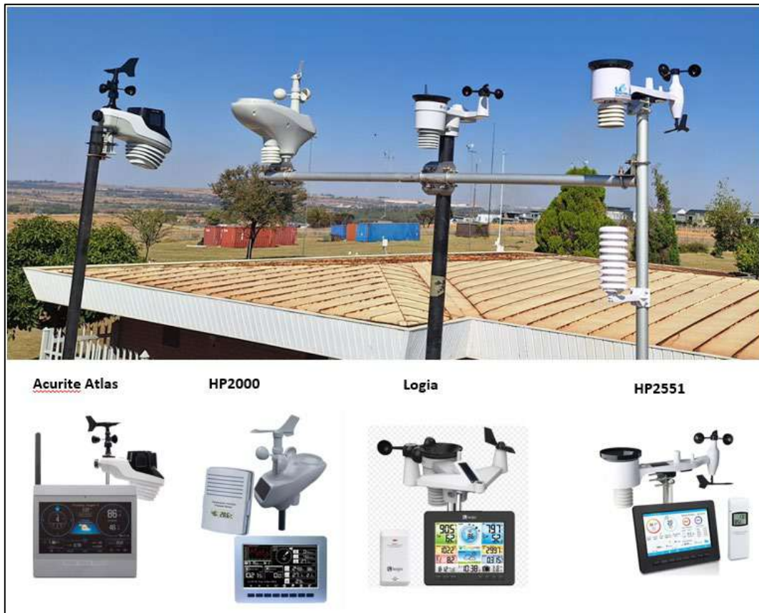
Figure 12. Commercially available Citizen Weather Stations (CWSs) used at the South African Weather Service Irene Office.
