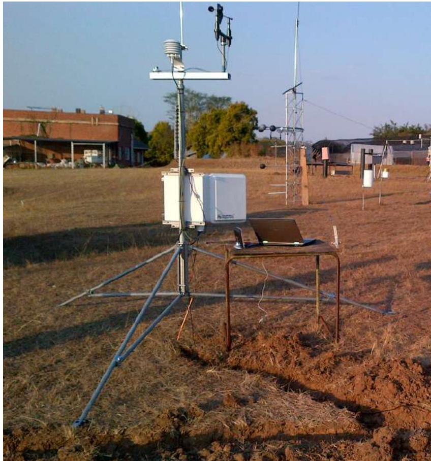
Figure 10. An automatic weather station (AWS) installed with standard sensors used to measure weather parameters at the UKZN site in Pietermaritzburg.
