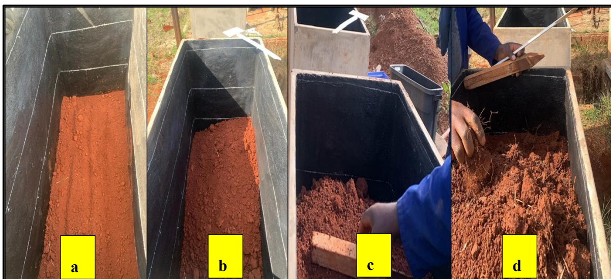
Figure 3.4: Soil packing inside the micro-lysimeters. (a) 60 - 70 cm layer placed above the medium-fine sand, (b) 40 - 60 cm layer placed above the 60 - 70 cm layer, (c) 20 - 40 cm layer placed above the 40 - 60 cm layer, and (d) 0 - 20 cm layer place above the 20 – 40 cm layer
