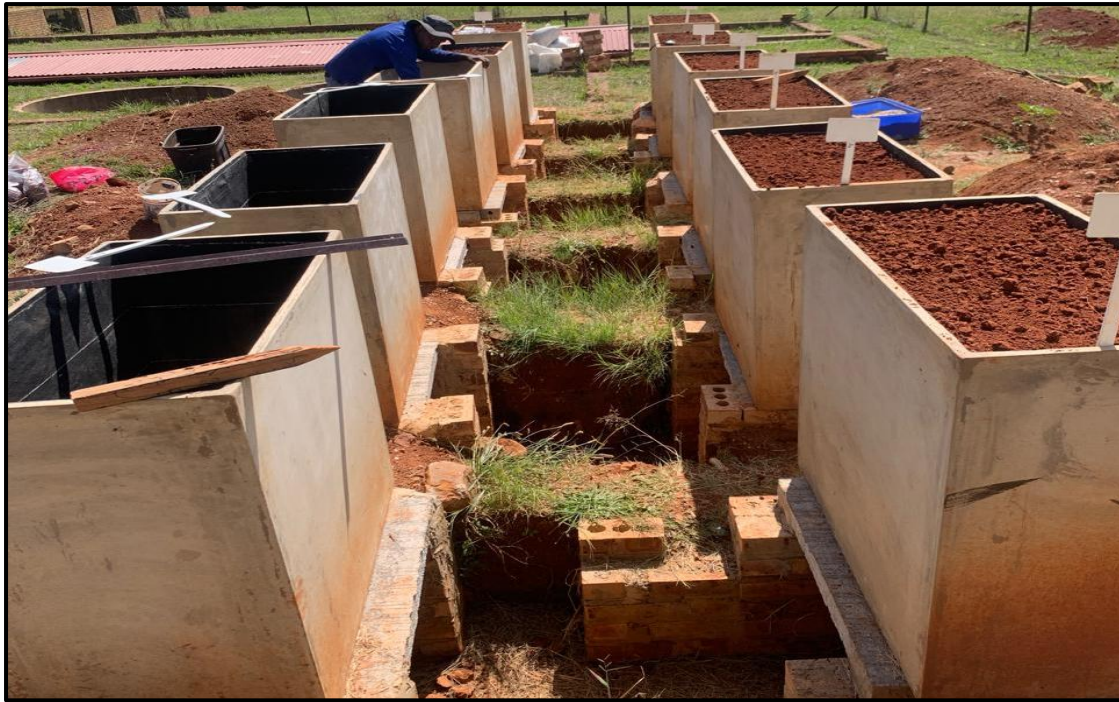
Figure 3.1: Field experimental layout and structure of the micro-lysimeters
