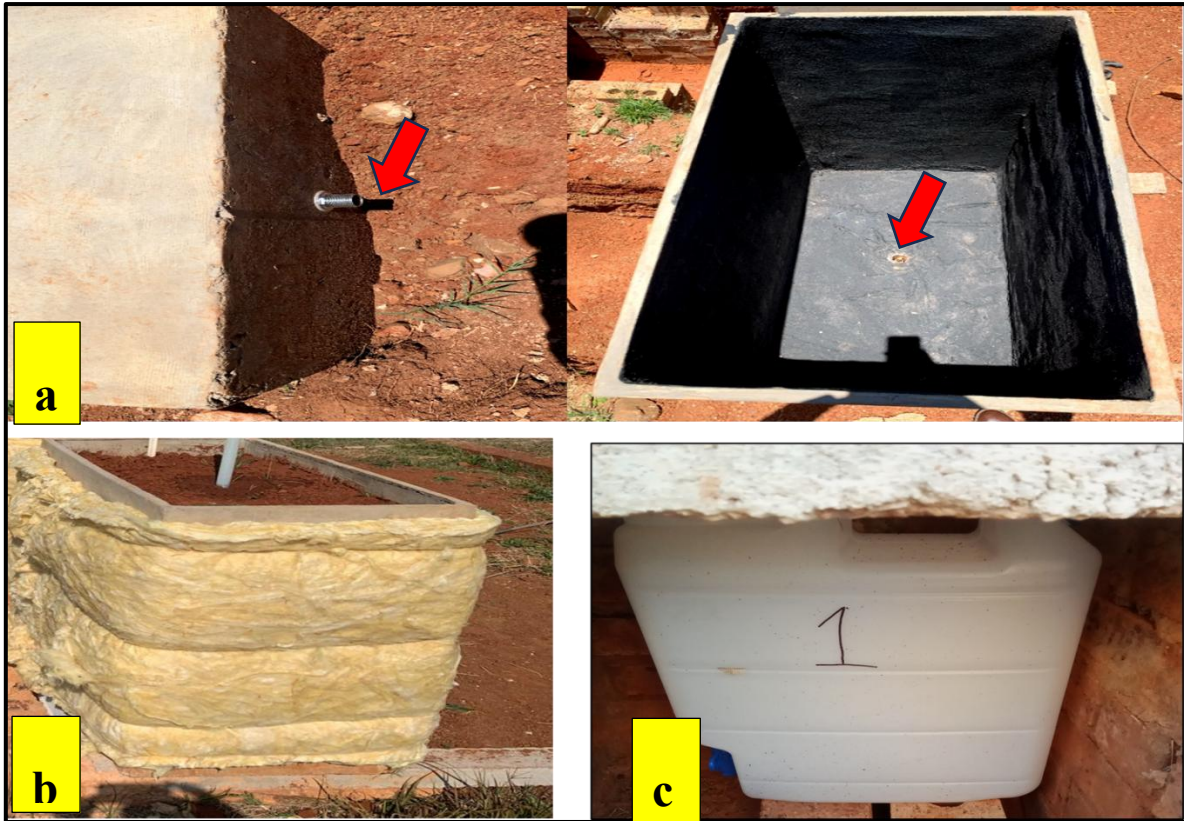
Figure 3.2: Detailed structural features of each micro-lysimeter, (a) drainage hole at the centre of the lysimeter, (b) fibre glass wool covering the outside of the lysimeter, and (c) collection cans placed at the bottom of each lysimeter
