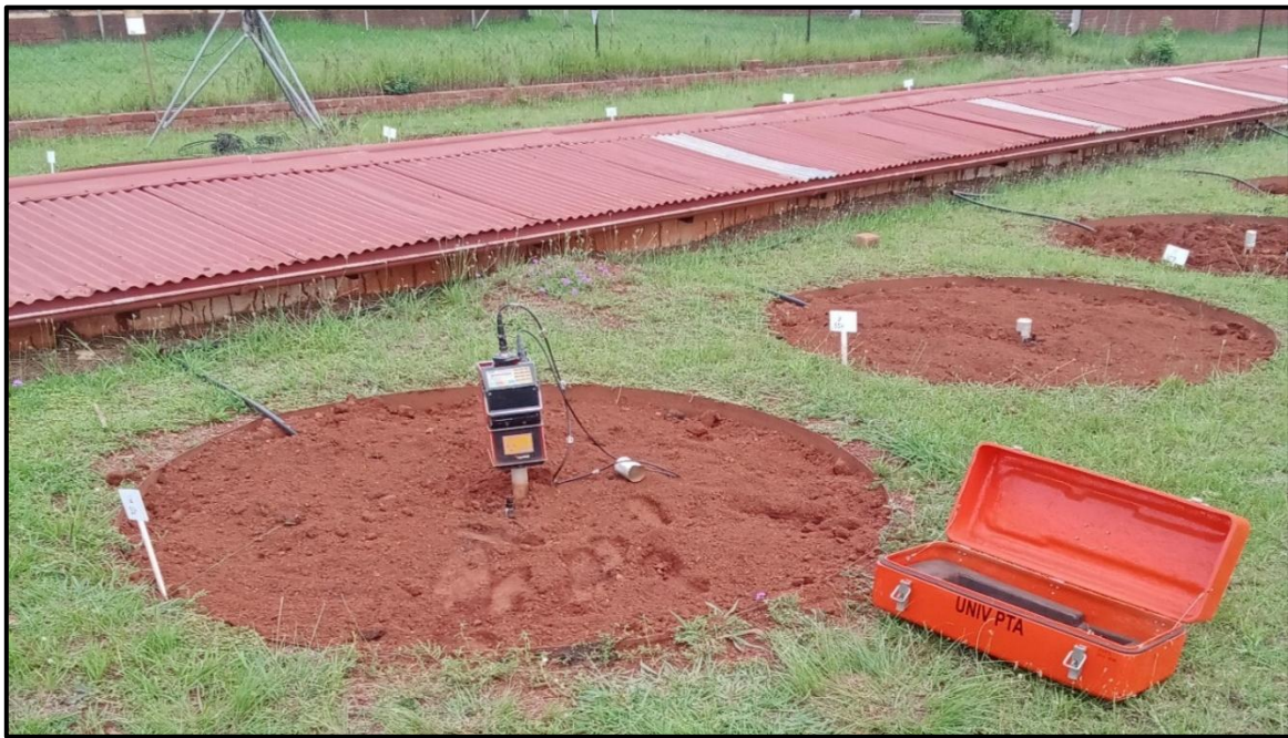
Figure 3.6: Field experimental layout and the structure of the macro-lysimeters
