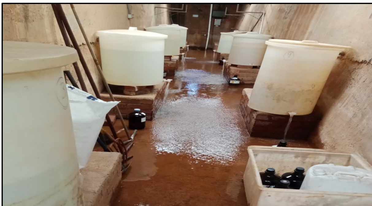
Figure 3. 7: Drainage collection tanks for macro-lysimeter housed underground
