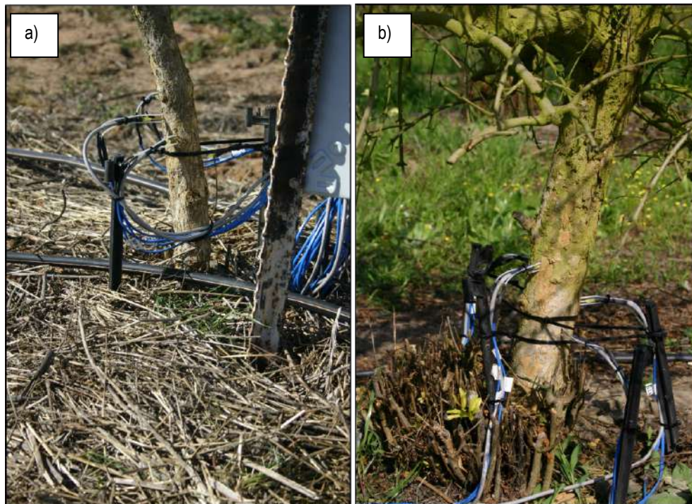
Figure 24. Heat pulse velocity heat ratio method equipment installed during August 2022 to monitor sap flow during the 2022/23 season in a) a young cv. ‘Wonderful’ pomegranate tree at Avontuur and b) a full bearing tree at Welgemoed. Four sets of thermocouples and heaters were installed in different positions around the stem.
