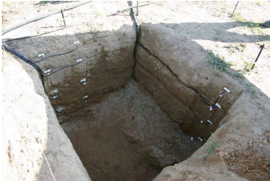
Figure 22. For the young pomegranate orchard at Avontuur CS650 soil water content reflectometers were installed in the tree row directly below the dripper nearest to the tree stem (most left-hand side) and midway to the next dripper (second from left). A set of four sensors were also installed perpendicular to the tree row in the work row (right).
