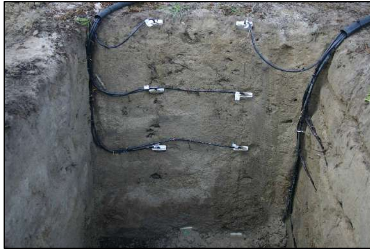
Figure 20. Soil profile pit at Welgemoed indicating a relatively uniform coarse sandy soil
