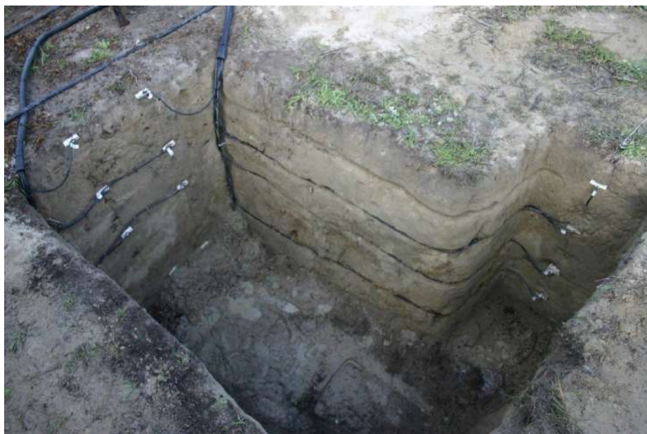
Figure 23. For the full bearing pomegranate orchard at Welgemoed CS650 soil water content reflectometers were installed directly below the dripper nearest to the tree stem (most left-hand side) and midway to the next dripper (second from left). A set of four sensors were also installed perpendicular to the tree row in the work row (right).
