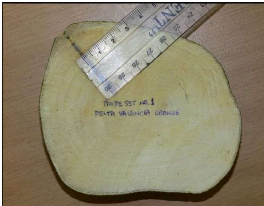
Figure 4 Determining the virtual wound width on a piece of wound cut crosswise from the tree trunk (Mahohoma, 2016)
