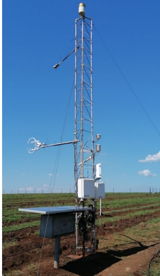
Figure 3-7 Eddy covariance system installed on a 6 m tall lattice mast
