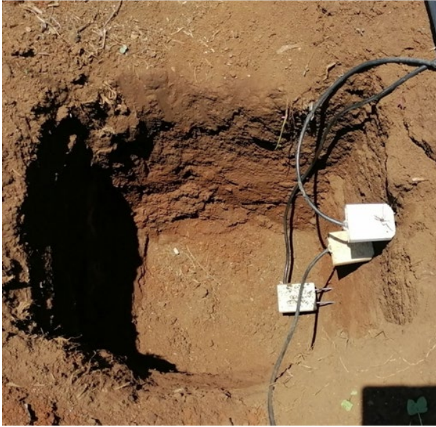
Figure 3-9 Soil volumetric water content probe to measure soil water profile
