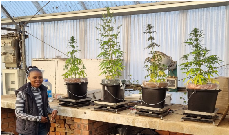
Figure 4-1 The plant pots with 3 females and 1 male plant placed on the loadcells eight weeks after planting
