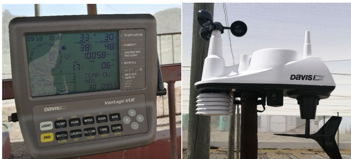
Figure 5.5: Davies weather station data logger (a) and atmospheric sensors (b).
