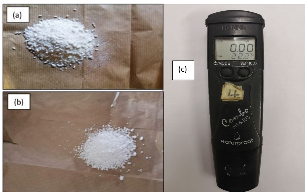
Figure 5.6: Hygroponic (a) and Calcium Nitrate (b) multi-component water soluble hydroponic fertilizers (c) Combo device (HANNA) used to measure Electrical conductivity in a solution. Adapted from (Araya and Moremi, 2021).
