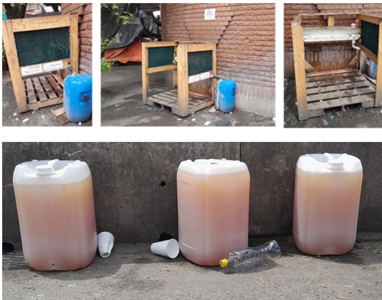
Figure 5.1. Urinals at the urine diversion research pilot urinary outside the toilets at the Durban Taxi Rank in Durban (top) and collected urine in 25 L containers (bottom).
