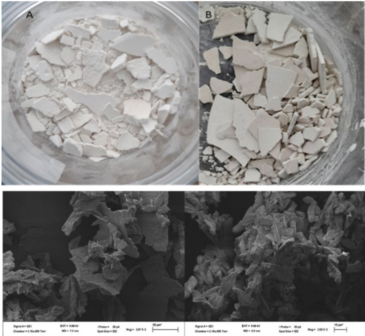
Figure 5.4. Precipitated struvite (top) 50% urine (A) and 100% urine (B) and SEM images of struvite precipitated using 50% diluted urine (bottom).
