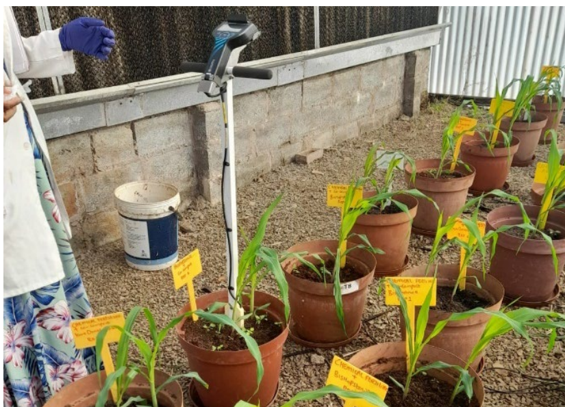
Figure 6.16. Measuring soil moisture in maize planted pots using the Hydrosense™ soil moisture meter.
