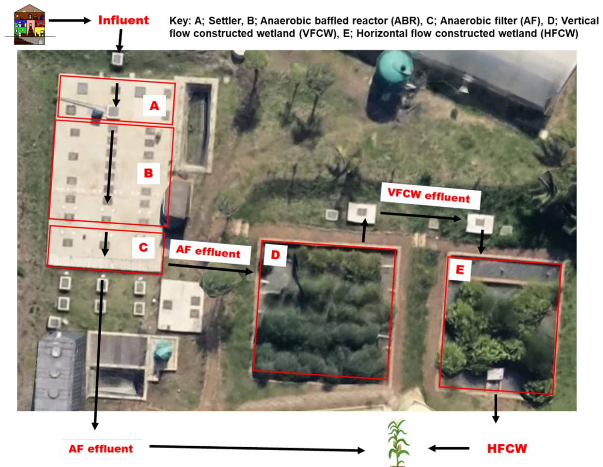
Figure 2.6: An aerial view of the decentralised wastewater treatment system (DEWATS) at Newlands Mashu showing different modules for wastewater treatment. Diagram by William Musazura.
